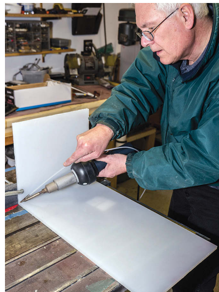
For long welds. Homer used the speed-welding tip. The rip fence on the table saw worked well as a jig to hold the material, but that did not prevent it from warping.
