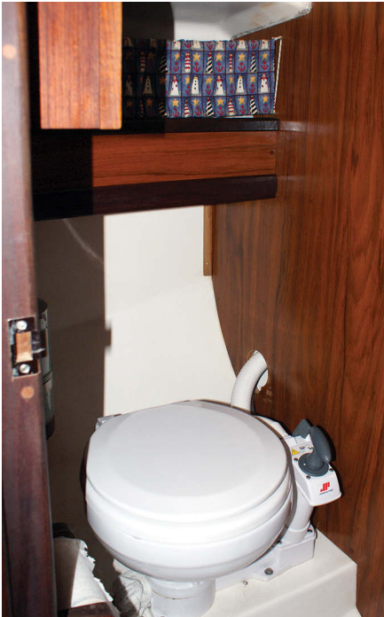
The head has a marine toilet to port and hanging locker to starboard. A privacy door in the main bulkhead closes it off from the saloon but not from the V-berth.
