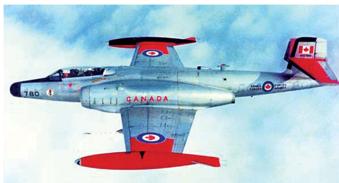
The size and best location for the tip tanks on the long-range Canadian CF-100 interceptor, introduced in 1952, was determined from wind-tunnel testing. This configuration was echoed in the location of lead bulbs on high-aspect-ratio sailboat fins. The winglets on the trailing tips further reduce the vortices streaming off the tanks, and these, too, were copied on sailboats.
