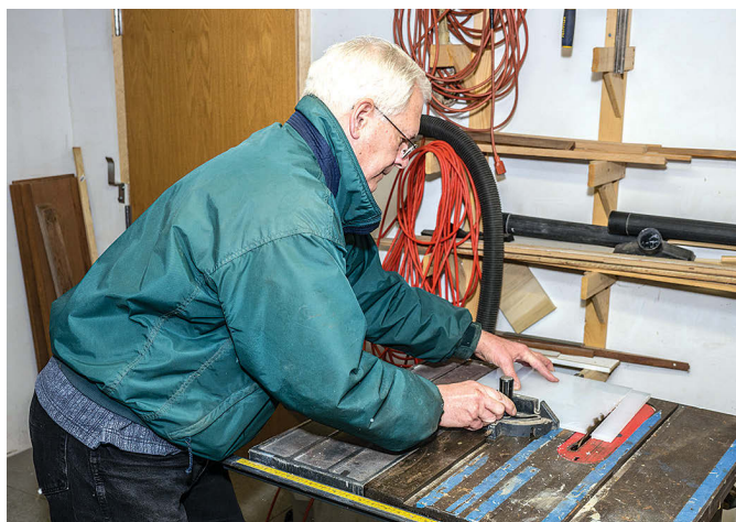
Homer made his new holding tank to fit under the V-berth with all the fittings accessible, at top. He used polypropylene sheet, which can be cut on a table saw using a carbide-tipped blade, above.
