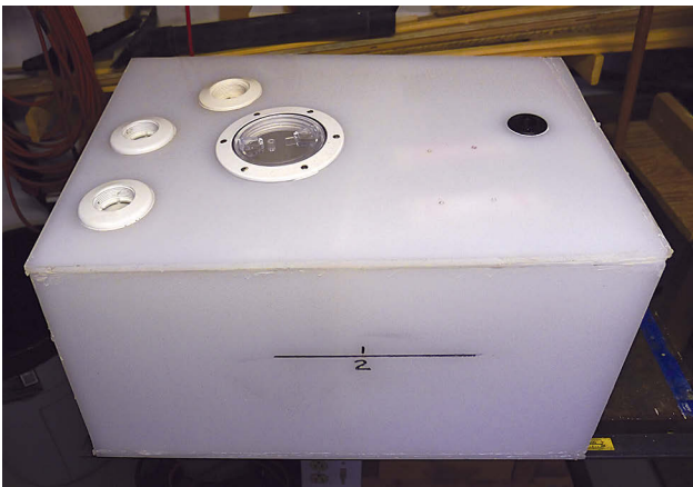
Before welding the tank top in place, Homer installed the pipe fittings, at left, and the inspection port, at right, that allows a look inside.
