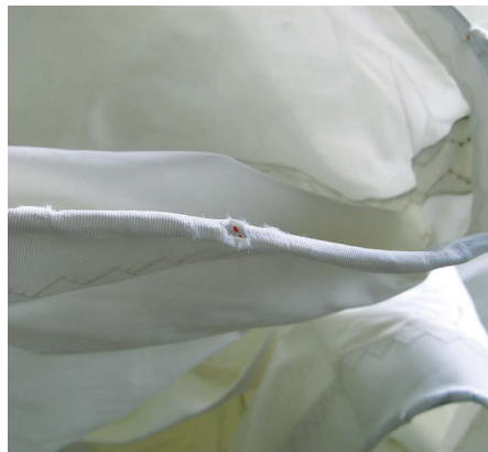
Look for damage along the leech, where chafe on rigging can expose the leech line.
