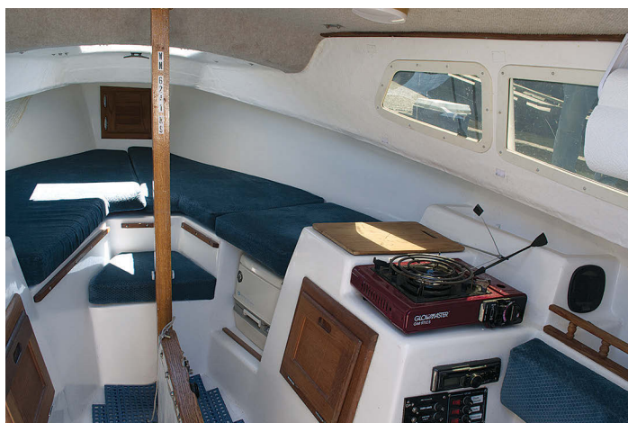
The daggerboard blocks passage through the cabin somewhat when raised, at left, but takes up less space than a centerboard trunk when it's lowered, above. A molded fiberglass liner forms most of the furniture and provides a place for a single-burner butane stove on the starboard side and a sink on the port side.
