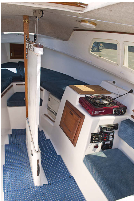
The daggerboard blocks passage through the cabin somewhat when raised, at left, but takes up less space than a centerboard trunk when it's lowered, above. A molded fiberglass liner forms most of the furniture and provides a place for a single-burner butane stove on the starboard side and a sink on the port side.
