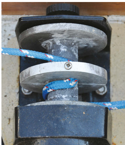
The lifting line leads from the winch and up the davit arm through a series of blocks, above. The divider on the winch drum allows the lines from both davit arms to wind or unwind simultaneously, below.
