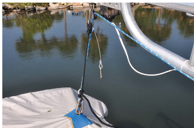
Roger built a teak box to contain the winch and the control unit to protect them from the elements, at left. It is sturdy enough to use as a step. Wire stops clip onto the davit and dinghy to provide extra support, at right. The black stop lowers the stern so the boat will drain.
