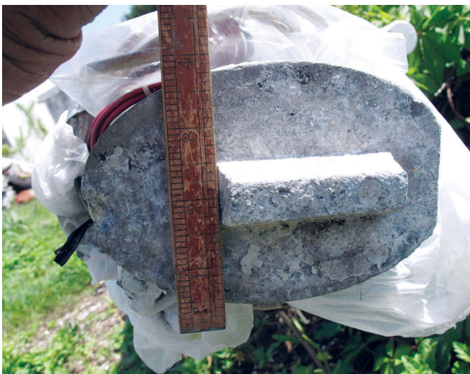
The tenon that sat in the mast step was also white with oxide.
