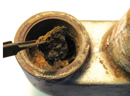
When the rust clot lining the elbow broke away, it completely blocked the passages for both the water and the exhaust gases, at left. Ed removed the debris for show and tell, at right.
