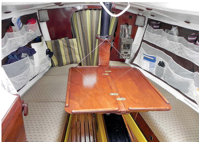
Jerry made a folding saloon table that pivots around the compression post, at left. It can be used as extra counter space for the galley or for dining, at right. The boat originally lacked storage space for cruising, so Karen made net hammocks that fit behind the saloon settees.
