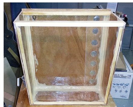
Before gluing the tank together, Ric taped together the plywood front, sides, top, and bottom, at left, to double-check the size and fit. He began the assembly by epoxying the front, bottom, sides, and corner moldings together, then covered the seams with thickened epoxy, center. He applied a layer of fiberglass cloth over the front, bottom, and sides, at right, and laid an extra layer of fiberglass tape over the monitoring ports.
