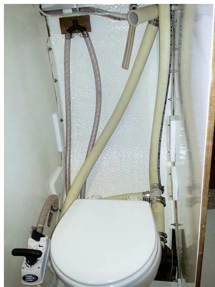
With the back in place, the tank was almost complete, at left. Ric installed all the hoses prior to mounting the tank, at right. The tee fitting in the discharge permits use of a deck pumpout.
