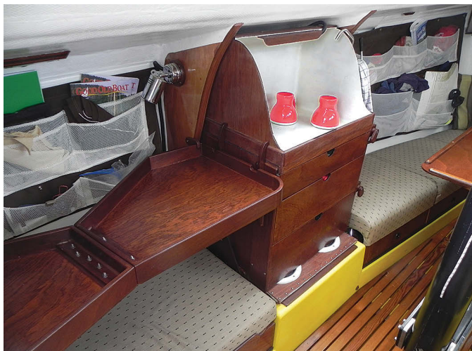
As a raceboat, the Mega 30 was originally fitted with a minimal galley. Among the modifications Jerry made were the foldaway counter and “spray booth,” at left, where he and Karen rinse dishes with a handheld pressure washer. The booth doubles as a countertop. On the starboard side, the galley has just enough space for a two-burner stove top with microwave oven beneath it, at right. The keel trunk is in the middle.
