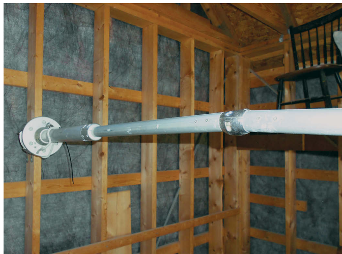
The bottom section of this headsail furler connects to the main foil at the luff feeder, creating a weak point when the system is uninstalled.
