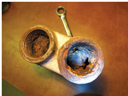
When the rust clot lining the elbow broke away, it completely blocked the passages for both the water and the exhaust gases, at left. Ed removed the debris for show and tell, at right.
