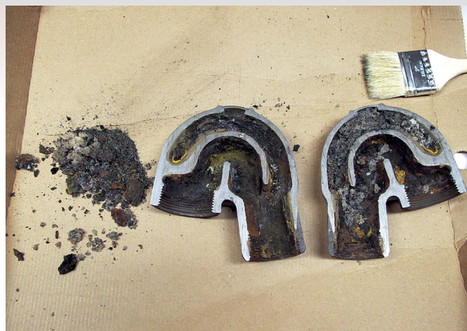
The water inlet on the mixing elbow was almost completely clogged, at left. Splitting the elbow revealed the extent of the blockages, at right.
