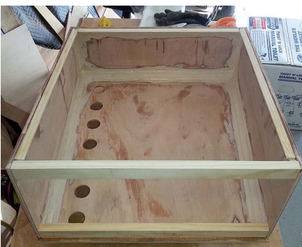
Before gluing the tank together, Ric taped together the plywood front, sides, top, and bottom, at left, to double-check the size and fit. He began the assembly by epoxying the front, bottom, sides, and corner moldings together, then covered the seams with thickened epoxy, center. He applied a layer of fiberglass cloth over the front, bottom, and sides, at right, and laid an extra layer of fiberglass tape over the monitoring ports.
