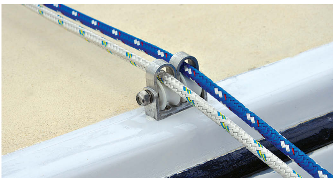
Roger's basic unit fits two sheaves into one piece of aluminum channel, at left. Where he needed to run six lines over the top of the saloon coachroof, at right, he connected three two-sheave blocks with a single through-bolt as a common axle.
