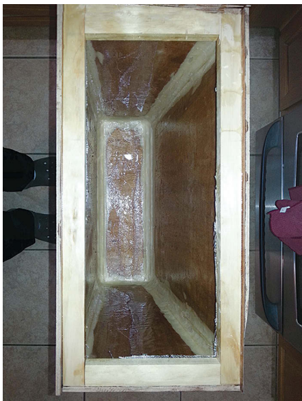
With the back in place, the tank was almost complete, at left. Ric installed all the hoses prior to mounting the tank, at right. The tee fitting in the discharge permits use of a deck pumpout.
