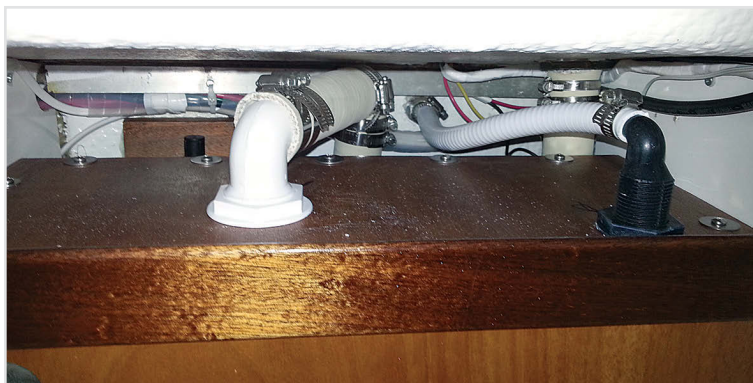
The tank discharges from the bottom, at left, and the "windows" show the level of the contents. After fitting the fill and vent, Ric screwed the lid in place, above.
