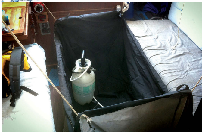
Cliff's Paceship PY 26 had no shower, so he rigged an outdoor grill cover to fit between the saloon settees and uses a garden sprayer.
