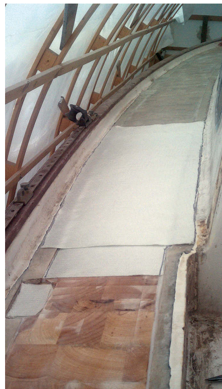
Once the new core was epoxied in place on the foredeck, above, it was time to begin laminating the top skin. First, though, Matt laminated the small pieces of cloth, at right, in place of the core in areas where stanchions and other fittings would be located. This will prevent water intrusion in the future.
