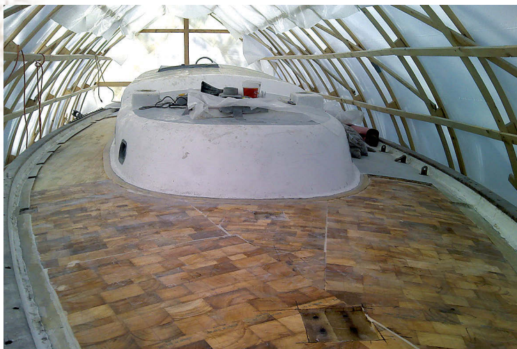
Once the new core was epoxied in place on the foredeck, above, it was time to begin laminating the top skin. First, though, Matt laminated the small pieces of cloth, at right, in place of the core in areas where stanchions and other fittings would be located. This will prevent water intrusion in the future.
