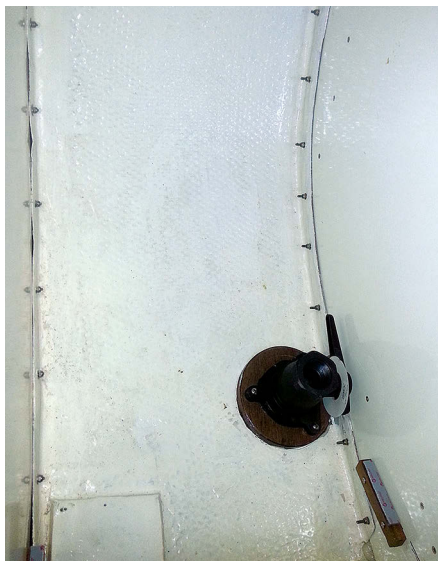
After gutting the head compartment, Ric fitted new bulkheads and a Marelon through-hull valve, at left. He made the cardboard mock-up for the tank after fitting the new head, at right.
