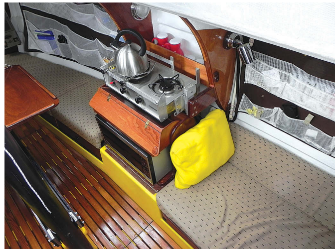
As a raceboat, the Mega 30 was originally fitted with a minimal galley. Among the modifications Jerry made were the foldaway counter and “spray booth,” at left, where he and Karen rinse dishes with a handheld pressure washer. The booth doubles as a countertop. On the starboard side, the galley has just enough space for a two-burner stove top with microwave oven beneath it, at right. The keel trunk is in the middle.
