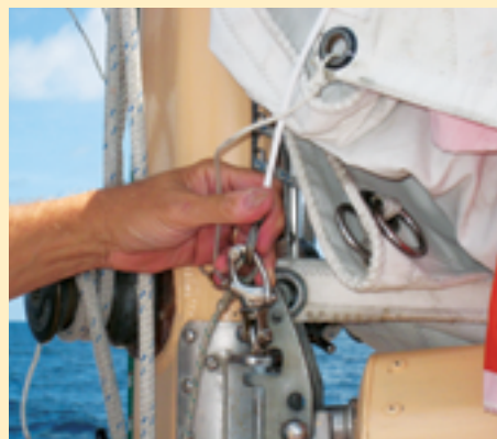
The Mainster's wire luff hooks to a snap-shackle attached to the gooseneck.
