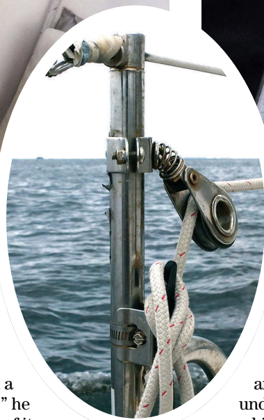
Cliff stows the downhaul line on a stanchion cleat at the cockpit, far left. The downhaul leads through stanchion blocks, inset, all the way to the bow pulpit. He clips it to the head of the sail with a snap shackle, above.
