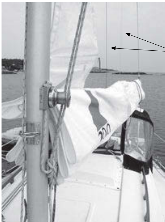
Two lines lead through the sail, causing it to fold like a fan.
