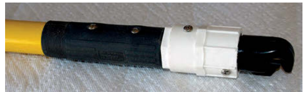
Some assembly is required for the inboard module of Clarence's whisker pole, above. Once the pieces are assembled, the inboard end begins to look like a functional whisker pole, below.
