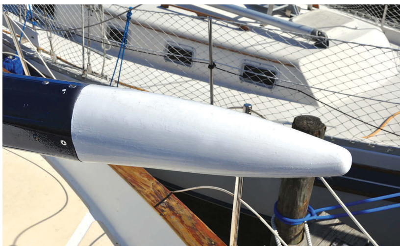
Roger fashioned yard ends out of cedar blocks and painted them traditional white, at left. They are removable so he can access the rope winch driver, at right, that turns the mandrel inside the yard at one end and the thrust bearing and tension adjuster at the other.
