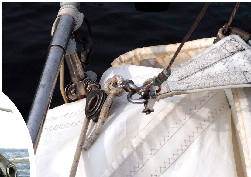
Cliff stows the downhaul line on a stanchion cleat at the cockpit, far left. The downhaul leads through stanchion blocks, inset, all the way to the bow pulpit. He clips it to the head of the sail with a snap shackle, above.
