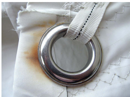
One of the more visible causes of chemical damage to sails is rust, which might arise from stowing a wet sail, upper image, or from corrosion of sail hardware, above.
