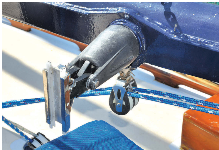
The gooseneck, at left, is a rather intricate affair as it has to allow the yard to rotate in several directions for sailing or stowing in a marina-friendly manner. Roger tested the furling system in his daughter's warehouse, at right, with a sail made from a plastic tarp.
