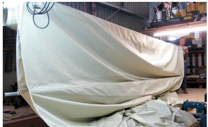
As the sail grew in size, Annie found herself shoving ever larger bundles of assembled fabric across the table as she sewed, at left. When she had completed most of the sewing, she suspended the sail from the boom, at right, to check her handiwork. The material is used for awnings.
