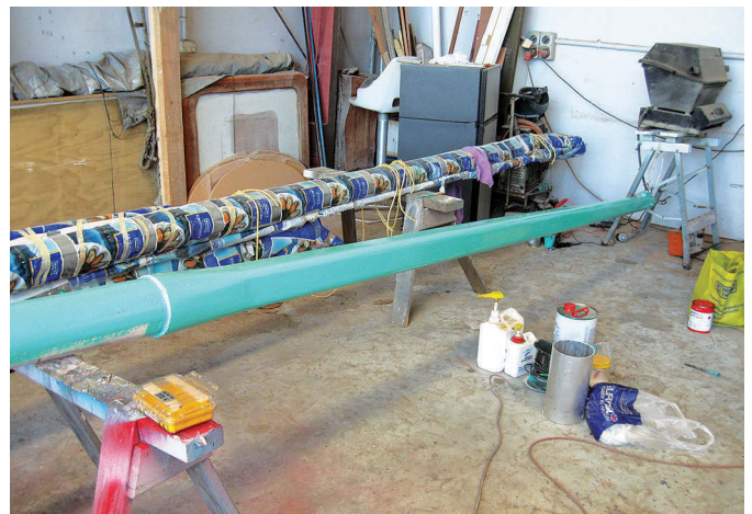
Annie built the upper part of the mast of Douglas fir, top of page. To make the butt of this topmast round to fit tightly into the aluminum bottom part, she built it up with wood and epoxy, at left. She built up a shoulder the same way. Painted her favorite color, the topmast is complete, at right.
