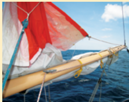
The clew outhaul stays rigged through its cheek block on the boom, always ready for action.
