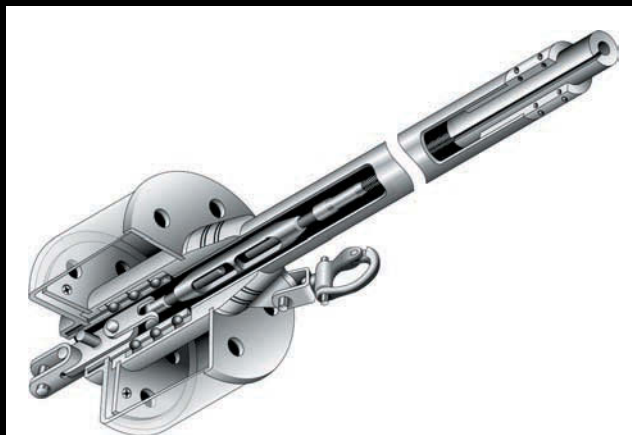
Cutaway views of the typical roller furling unit: drum, at left, and upper swivel, at right.
