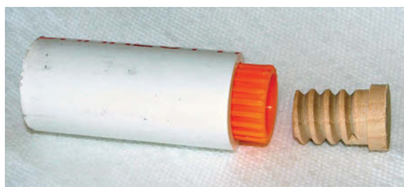
He cut the pipe to that length ( 2\frac{3}{4} inches) and cut the dowel at the same mark.
