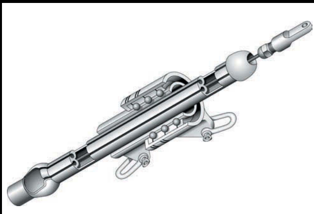
Cutaway views of the typical roller furling unit: drum, at left, and upper swivel, at right.
