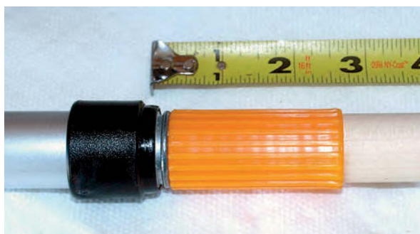
Clarence measured from where the PVC pipe seated on the pole to the end of the coupler and added \frac{1}{4} inch.
