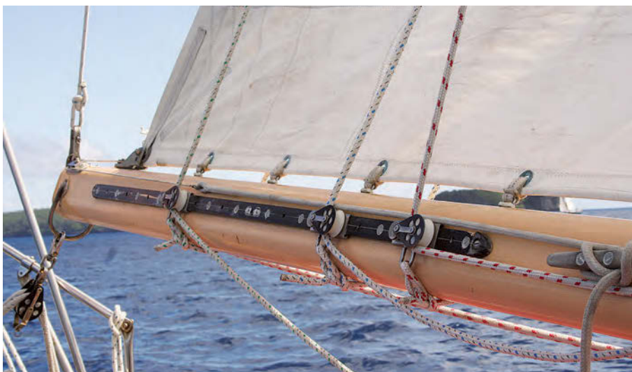
Three reefs in the mainsail means three clew outhauls, above. Under a full mainsail, the outhaul tails are short, but once the first reef is tied in, the tails of all three need to be coiled and securely stowed, below.
