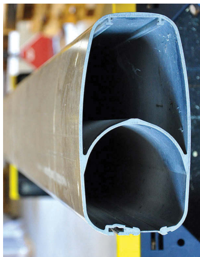
An in-yard roller-furling square sail is not a stock item at most sailmakers, so Roger had to improvise. He purchased a length of section for in-mast furling, at left, and trimmed it.
