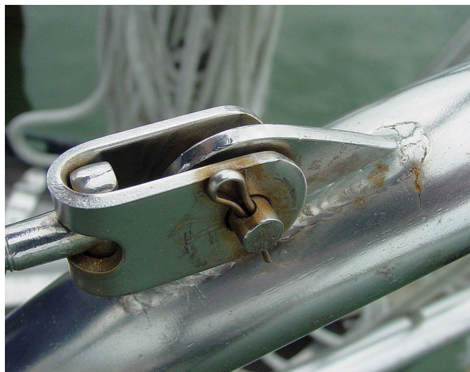
A stress crack and some corrosion are visible at the base of the lifeline-attachment eye where it's welded to the pulpit, at left. Also, the cotter pin looks loose and could fall out if the clevis pin it's securing rotates over time due to vibration. Where a vinyl-coated lifeline passes through a stanchion, the coating can chafe away, at right, creating a path for water to enter the wire and initiate corrosion.
