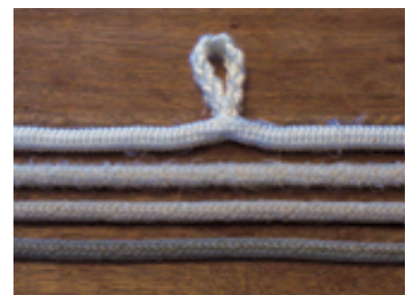
The rope samples line up ready to be tested, left. From the bottom: A, B, C, D, E, F, per the table above. In some cases, washing caused the core of new rope to "pop" through the cover, center. Washing makes polyester rope fuzzy, right.
