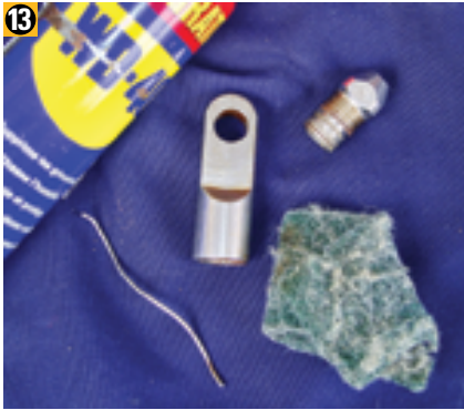
Clean both threaded parts of the terminal before reusing them.
