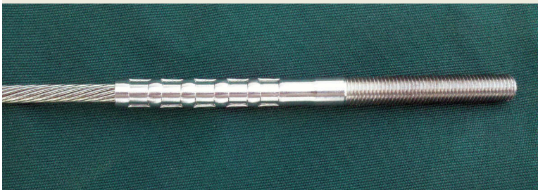
Each terminal requires five crimps, above. The jig made sawing the cable easy, at right, and the result was a clean square cut.
