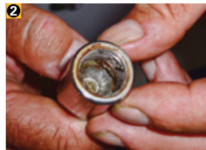
Inspect the female thread for signs of rust and traces of thread sealant.
