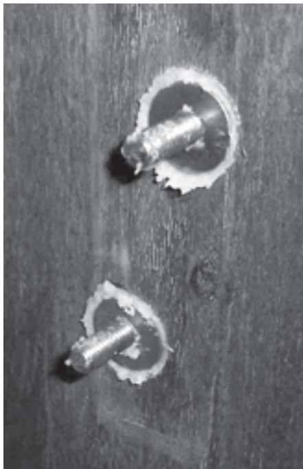
Chainplate holes drilled for bushings, top; a washer with epoxy ready for insertion, center; and a washer and epoxy packing, bottom.
