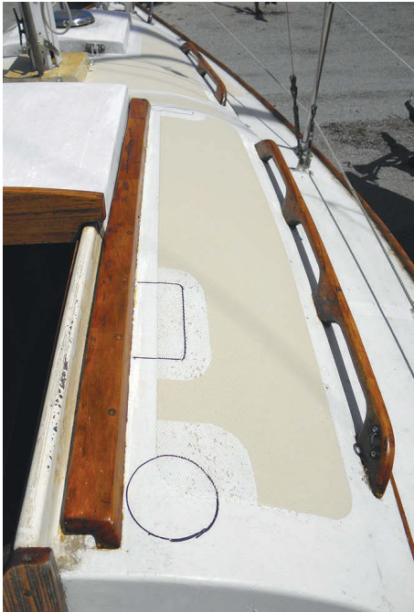
Measure twice and cut once isn't enough for Steve. After marking where he thought the organizer, clutches, and winch should be fitted, at left, he finished other projects before making a final check, at center and at right, before finally drilling holes in the cabintop, below.
