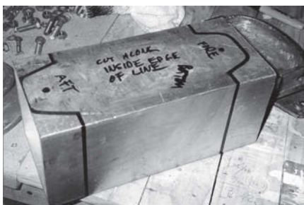
1/4-inch x 4-inch-square aluminum tubing scrap with the outline of the original step casting. This will become the mast step riser that sits on the keel. It's worth less than $10 from a scrap metal dealer.
