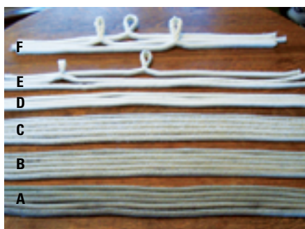
The rope samples line up ready to be tested, left. From the bottom: A, B, C, D, E, F, per the table above. In some cases, washing caused the core of new rope to "pop" through the cover, center. Washing makes polyester rope fuzzy, right.
