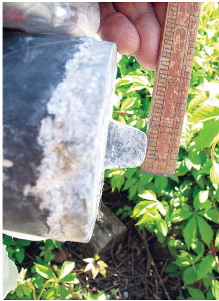
The old mast foot was severely corroded, as was the base of the mast around it.
