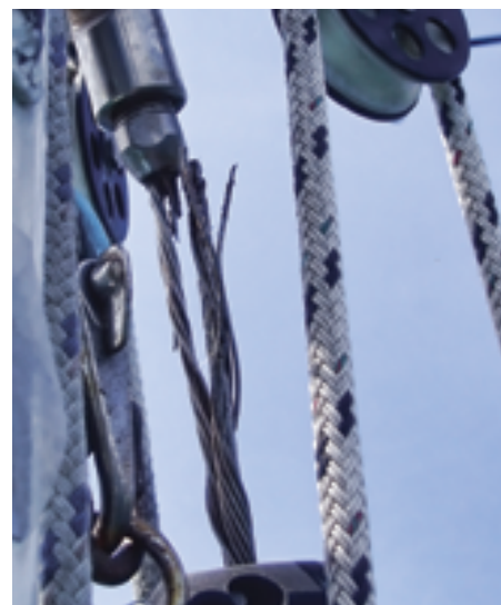
Leslie and Philip discovered this damage at the upper end of their forestay while anchored in a remote anchorage hundreds of miles from the nearest rigging supplier.
