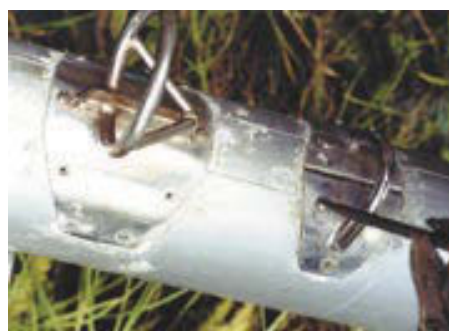
Even this badly corroded stay, top, had plenty of good metal left. Removing all the mast hardware, above.
