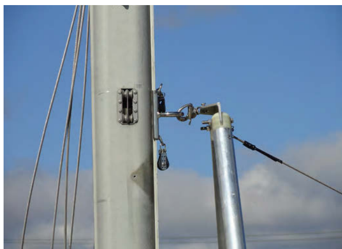
The apex of the after A-frame attaches to the ring on the spinnaker-pole car with a snapshackle. The stainless-steel wire leading forward connects it to the forward A-frame.
