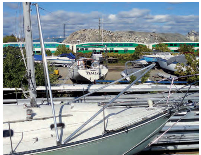
When the mast reaches its fully vertical position, it remains supported by the A-frame while the shrouds are connected to the chainplates.
