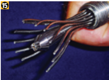
Slide the wedge over the wire core and carefully re-lay the strands.
