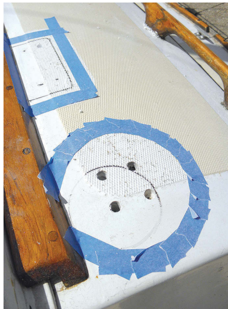
Measure twice and cut once isn't enough for Steve. After marking where he thought the organizer, clutches, and winch should be fitted, at left, he finished other projects before making a final check, at center and at right, before finally drilling holes in the cabintop, below.
