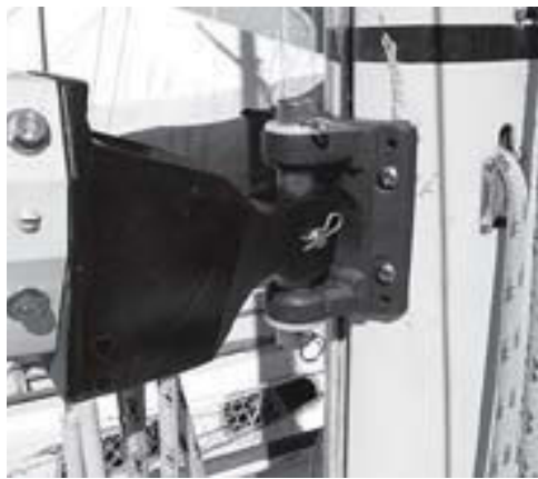
The used boom was a bargain, but the pin for the gooseneck was missing. A new pin was one of the last additions.
