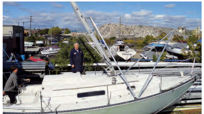
The pivot point of the A-frames is not level with that of the mast, but the apex of the after A-frame, attached to the spinnaker-pole car, accommodates the offset by rising up the mast as the mast is being raised.
