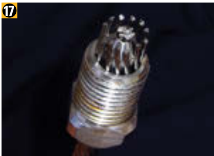
Properly assembled, the strands lie uniformly around the wedge.
