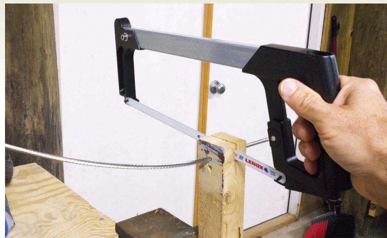
Each terminal requires five crimps, above. The jig made sawing the cable easy, at right, and the result was a clean square cut.
