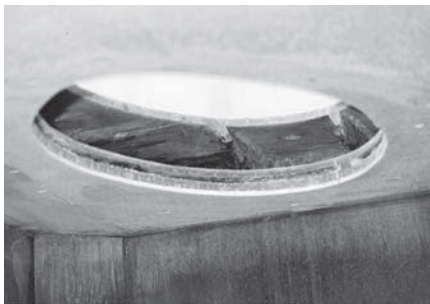
Shown from below, loose adhesive between the headliner and bottom deck laminate has been removed. Note that the staining on the headliner has been cleaned off. There was only cosmetic discoloration of the bulkhead tops. Inspect any bulkheads in the immediate vicinity for water damage.
