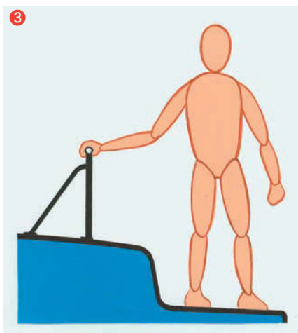
The pilot rail is inboard and waist high so a sailor can reach it without bending. A brace is essential at each end of the rail.
