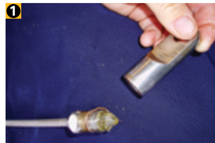
The first step in disassembling a terminal is to unscrew the two parts.
