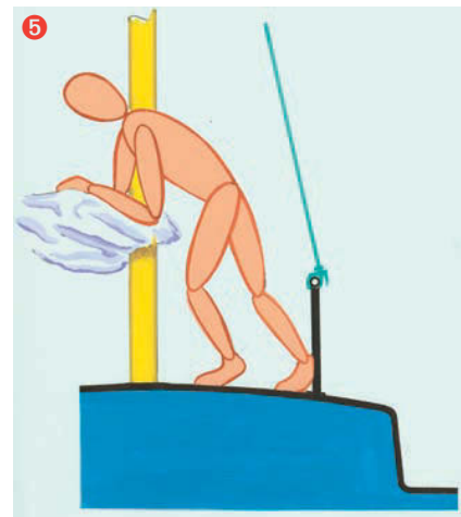
A pilot rail also offers a foot brace for working on the mainsail in a seaway and a handy attachment point for halyards.
