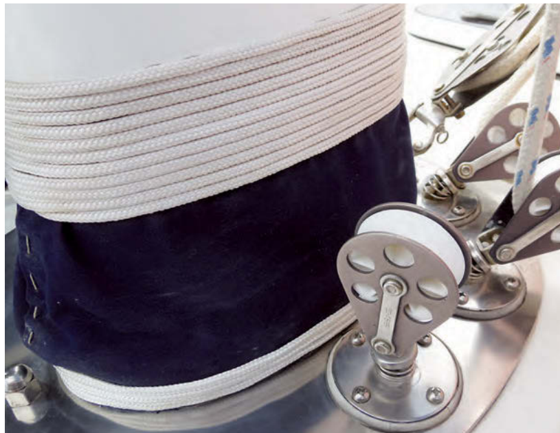
Since the rubber boot didn't look "finished," David covered it with a dress boot made of Sunbrella, then added whippings top and bottom.
