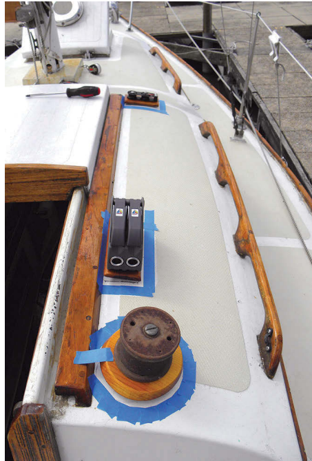
Measure twice and cut once isn't enough for Steve. After marking where he thought the organizer, clutches, and winch should be fitted, at left, he finished other projects before making a final check, at center and at right, before finally drilling holes in the cabintop, below.
