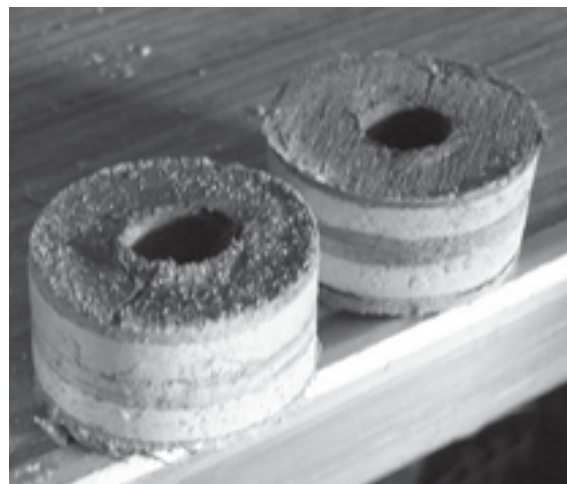
These bushing cores brought relief. The wood in the bore of the holes had been worked by repetitive forces but was not wet or damaged.
