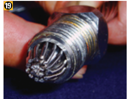
Unscrew the terminal end and examine the assembly for uniformity.
