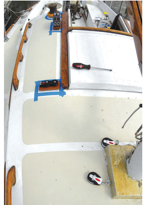
Measure twice and cut once isn't enough for Steve. After marking where he thought the organizer, clutches, and winch should be fitted, at left, he finished other projects before making a final check, at center and at right, before finally drilling holes in the cabintop, below.
