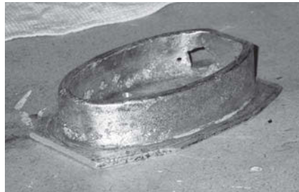
The mast step is now clean and bare with the ears cut off and holes drilled. Note the area where it corroded all the way through. This will be filled with thickened epoxy.
