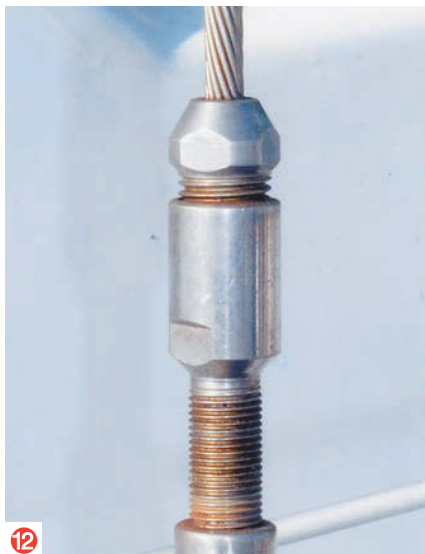
Check for breaks in the rigging wires (10). Check for cracks on the fittings (11). A common do-it-yourself swageless fitting (12).
