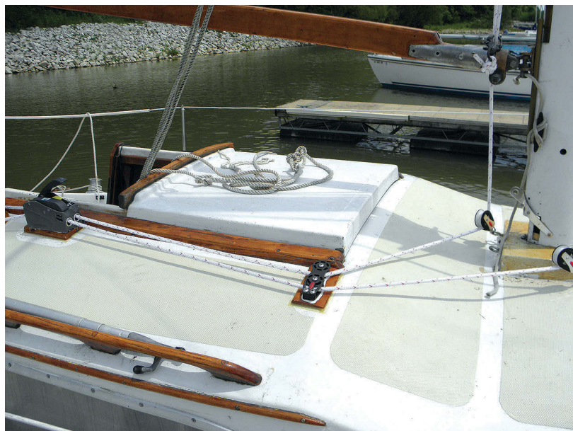
All the deck woodwork received several coats of varnish while Steve worried about drilling holes, at left. Installed at last, above, the organizer and clutches handle the halyards for the mainsail and jib. Note the boom and gooseneck.
