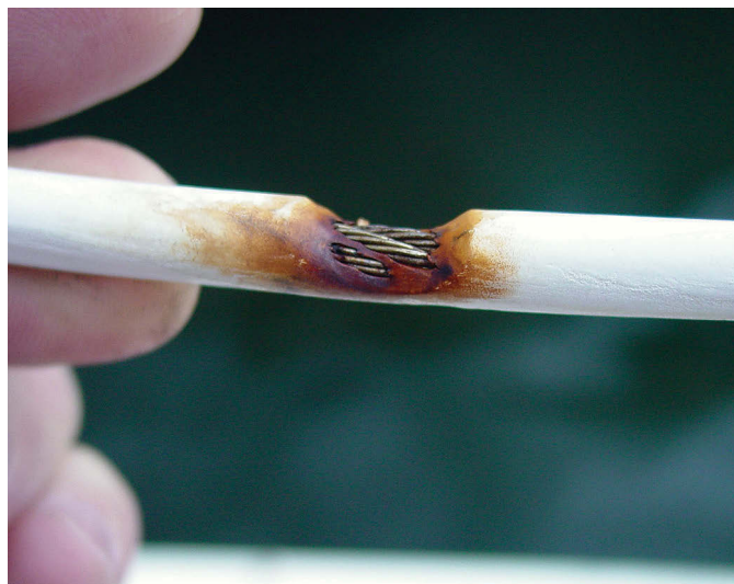
A stress crack and some corrosion are visible at the base of the lifeline-attachment eye where it's welded to the pulpit, at left. Also, the cotter pin looks loose and could fall out if the clevis pin it's securing rotates over time due to vibration. Where a vinyl-coated lifeline passes through a stanchion, the coating can chafe away, at right, creating a path for water to enter the wire and initiate corrosion.
