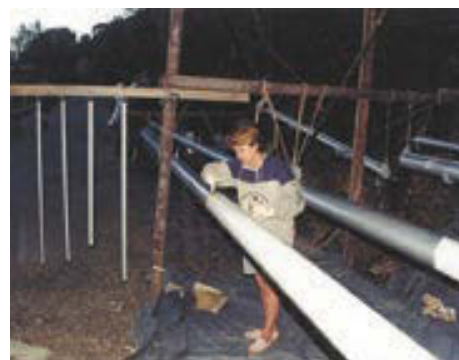
Michael cleans the old paint off the stripped masts, top. Preparing the aluminum spars, center, using a fine random-orbital sander. Tere touches up the overlap from white to silver paint, above. This photo also shows the mast-support gantry and spreaders.
