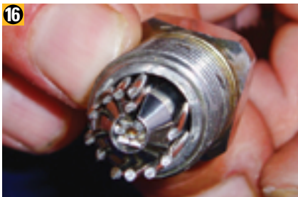
In this poor assembly, a strand is lodged in the slit in the wedge.
