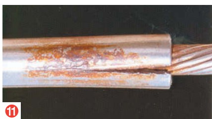
Check for breaks in the rigging wires (10). Check for cracks on the fittings (11). A common do-it-yourself swageless fitting (12).
