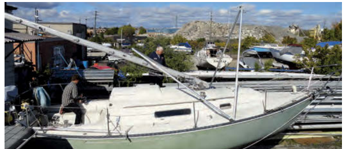
Two A-frames share common pivot points at the deck and are connected by a wire between their apexes. The forward one provides the raising lever and the after one lateral support for the mast.
