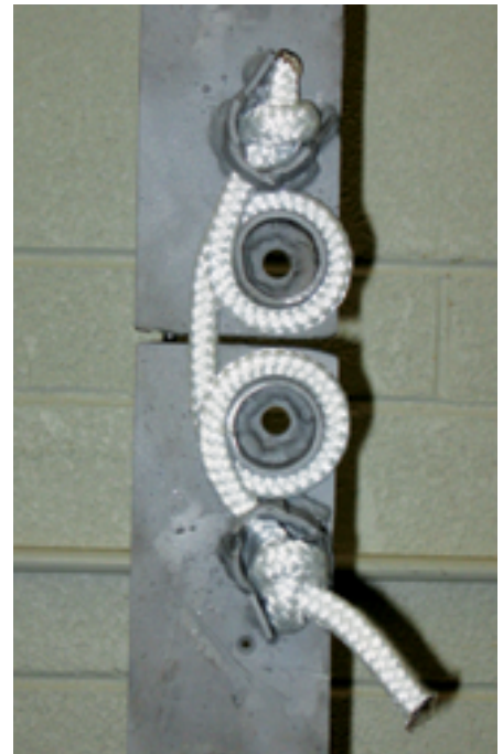
Washing old rope softens it, at left above. From the rear, the unwashed sample is the stiffest, followed by once washed and 10-times washed. Each rope sample was subjected to the 30,000-pound test machine, center, secured between two capstan grips, at right.
