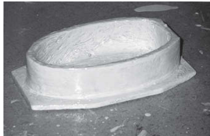
Phillip bedded and through-bolted the step casting to the top plate of the riser. Then he bedded and screwed the riser to the keel. He coated the screws and bolts with 3M 5200 where they contacted the aluminum.
