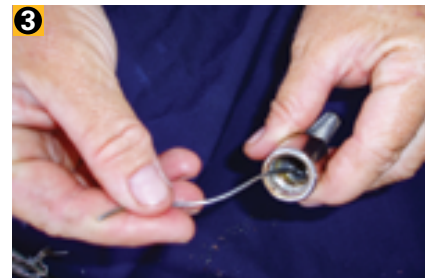
Clean the threads inside the fitting. A strand of wire works well for this.
