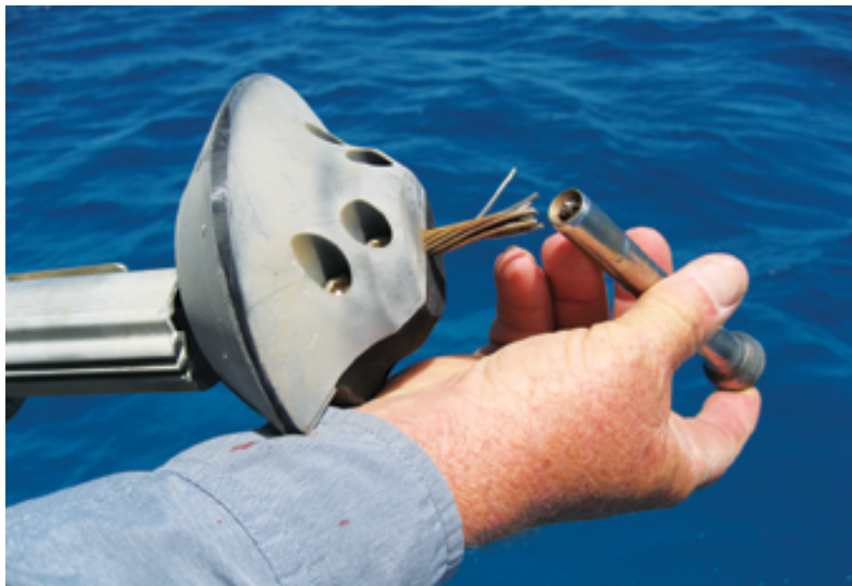
Stainless-steel rigging can succumb to metal fatigue, especially in places such as this, where the weight of a jib-furler caused the forestay to flex at the swaged-on fitting.
