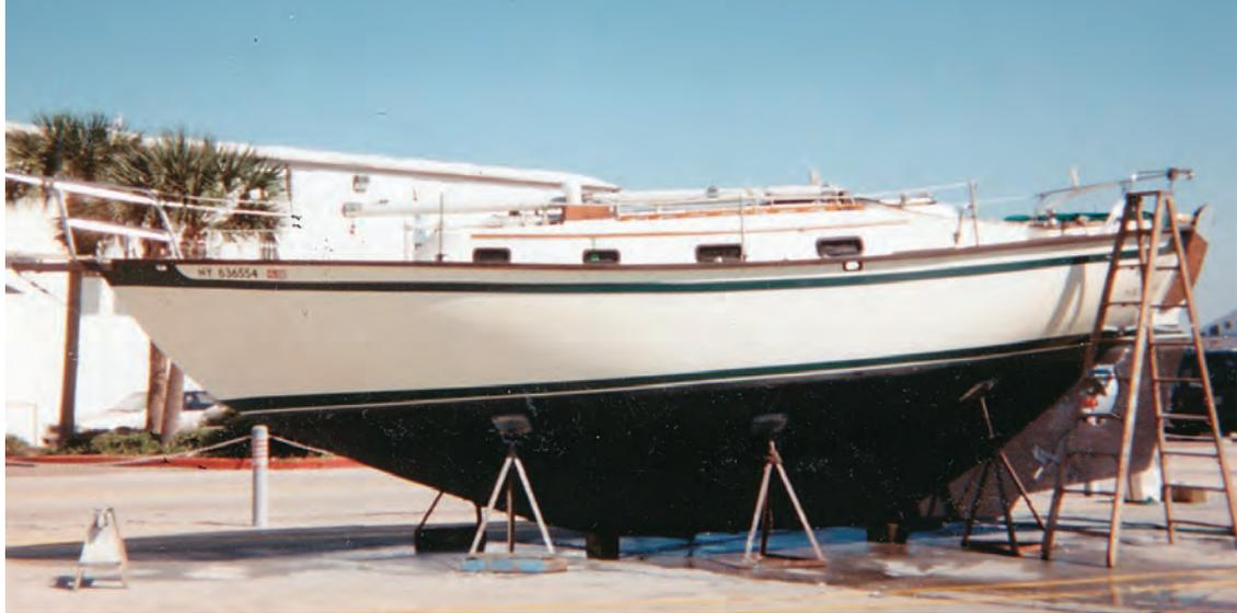
The boat's underwater profile, as we've already seen, is old-fashioned, well tested, and therefore greatly comforting to conservative cruisers. The outboard rudder is efficient and easy to get to if anything goes wrong.
