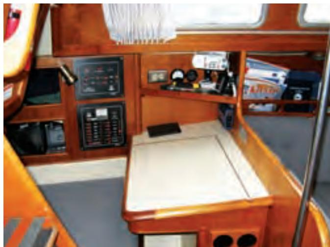
The Ericson 32-III has a neat, well-organized galley with stove/oven, ample storage, and lots of teak, at left. For a boat of this size, the chart table is quite generous. Its seat is the head of the quarter berth, which at 6 feet 6 inches makes an adequate sea berth, at right.
