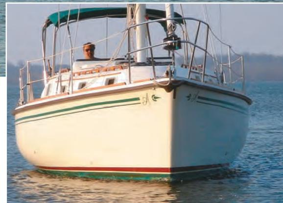
of 11 feet 4 inches and waterline of 27 feet 11 inches result in a spacious interior. This feature alone accounted for most of the boat's popularity, especially with liveaboards. The Allmand 31's wide beam also accounts for its significant form stability.
