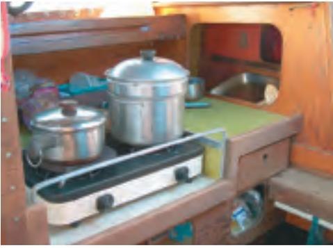
board. On *Scrimshaw*, there are both freshwater and saltwater pumps. To port is another counter with recessed two-burner propane stove. The galley has ample Formica-topped counter space, with storage areas below the counters and behind them and forward under the cockpit. There are large fixed ports on either side.
