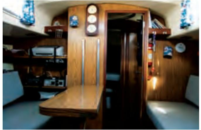
Good old test boat, *Tomfoolery*, has the “traditional” arrangement, in which the compact galley is laid out either side of the companionway, above left. In the saloon, settees facing each other across the dining table make good sea berths, above right. With the table stowed, access forward to the head and stateroom is much improved, below.
