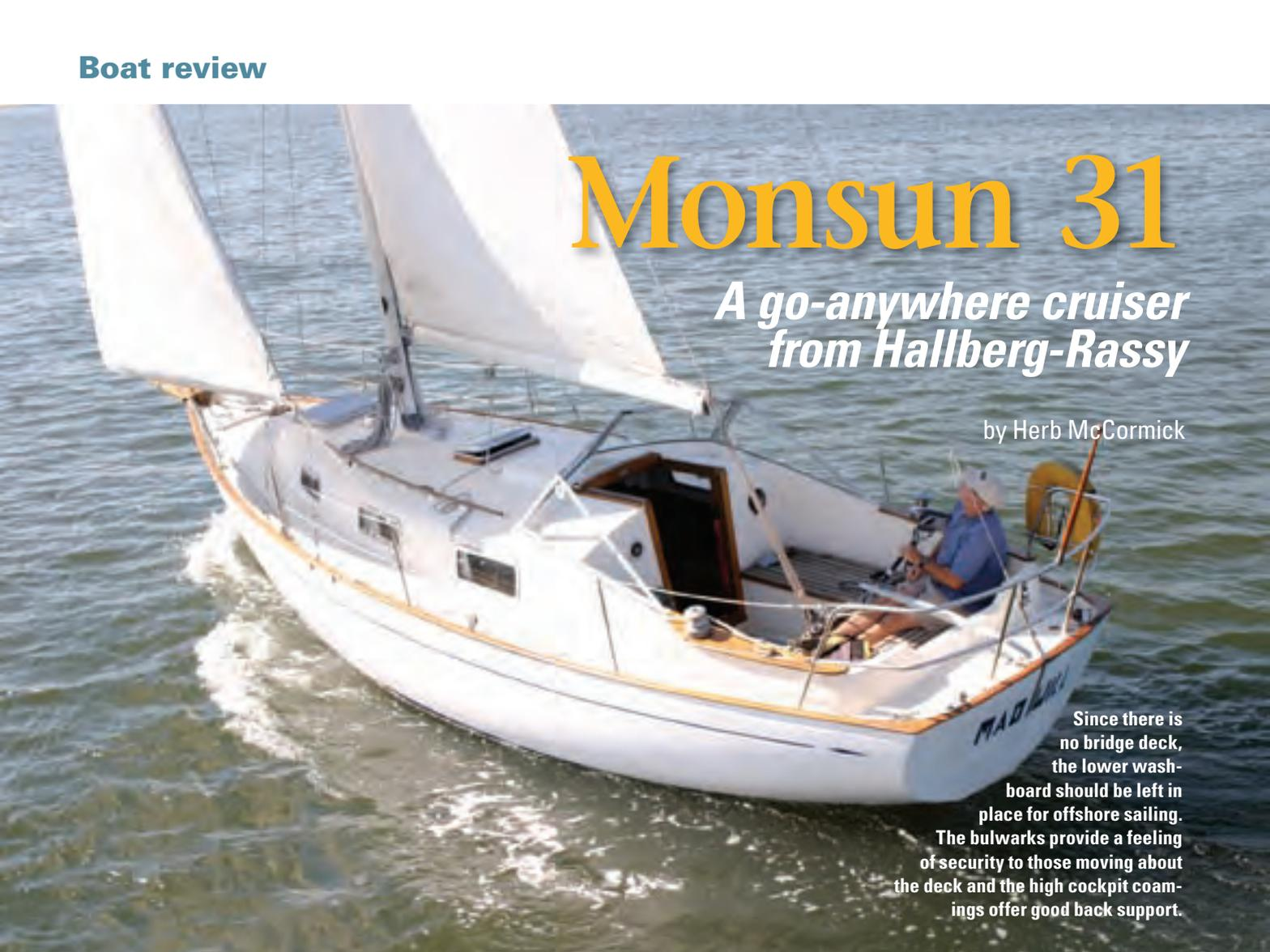
Since there is no bridge deck, the lower washboard should be left in place for offshore sailing. The bulwarks provide a feeling of security to those moving about the deck and the high cockpit coamings offer good back support.
