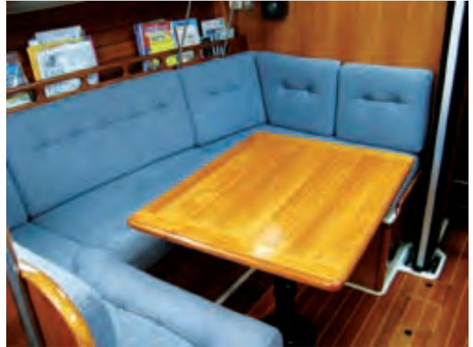
In this view, looking forward from the saloon to the forward cabin, the tie rods connecting the starboard chainplates to the Tri-Axial Force Grid are clearly visible, at left. The dinette table drops to make a 4-foot-wide double berth, at right. The cabin sole is teak-and-holly veneer-faced plywood.
