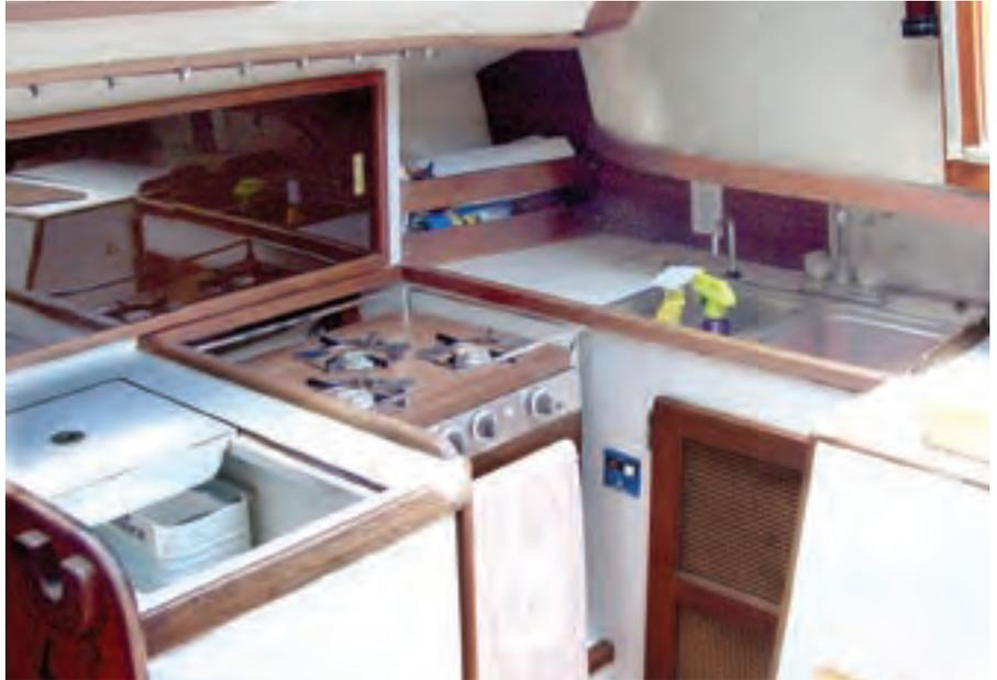
**The galley is aft to starboard, with a double sink under the bridge deck, a three-burner gimbaled stove/oven, and icebox. There isn't much counter space.**
