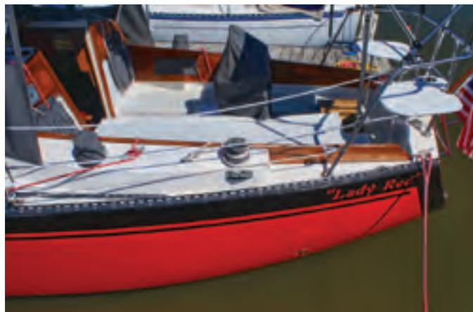
Though many Ranger 33s have been retrofitted with anchor rollers, *Drifter* retains the original arrangement, with individual navigation lights, two chocks, and a single cleat, at left. Teak coamings add a touch of elegance in the cockpit, at right, but do require some work if they are to be kept oiled or varnished. Primary and secondary winches and cleats on the cockpit coamings reflect the boat's age and its racing origins.
