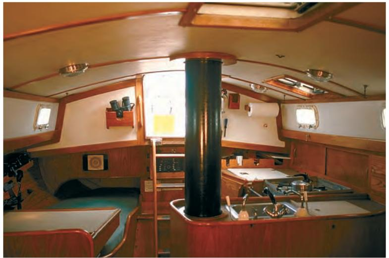
***Wastrel's interior is sumptuous. Even here, however, the traditional sailor realizes that this boat has a very different kind of rig. The main mast is in the bow, the mizzen is two thirds of the way aft.***
