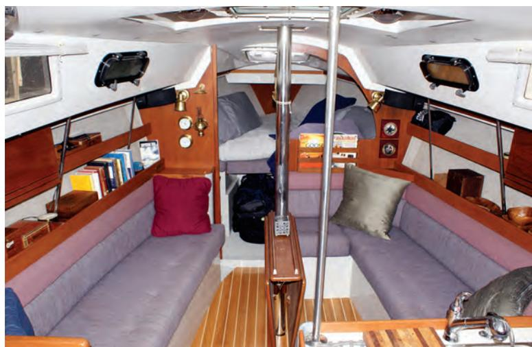
A dedicated navigation and “command” station is always appreciated, especially in a 32-foot boat, at left. The door at left is to the head. With the panel between the saloon and forward cabin (to starboard of the mast) swung open, the interior seems huge, at right. The open shelves outboard add to the sense of space.
