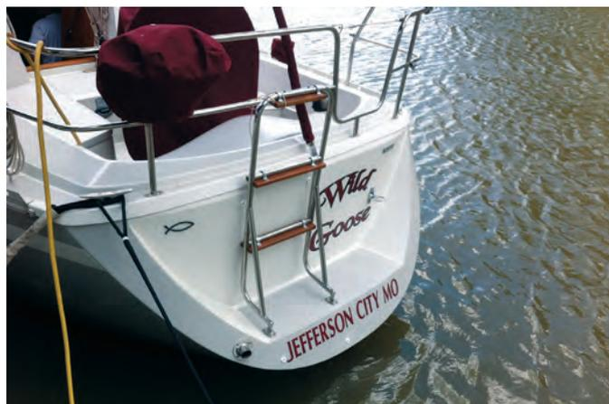
The sharply sculpted cockpit is comfortable, at left, and the T-configuration makes getting by the wheel less onerous, but the seats are not long enough for naps. The scoop transom, at right, with its offset gate and folding swim ladder, is a popular feature because it provides a safe and convenient way to board the boat.
