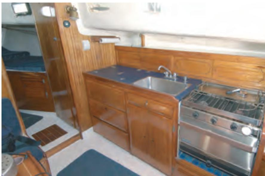
**Two views of the interior of the Columbia 33 at right. Both the 36 and the 33 have the long galley on the starboard side and an, otherwise traditional, layout. The 33 gives up space in the head and sacrifices the nav station for a small table.**
