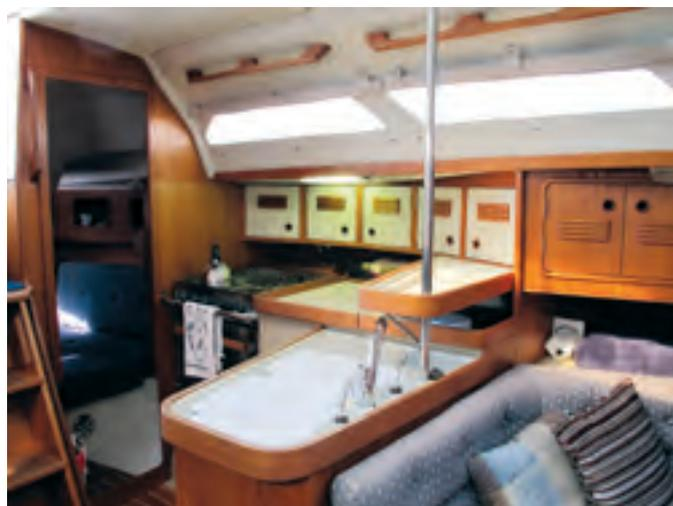
The C&C 34+ has quite a plush interior, at left, and the openings in the forward bulkhead expand its spacious feel. While a little short on counter space, the galley, at right, does have a double sink, decent storage, and a gimbaled stove. The private quarter berth is just visible aft. The nav station and head are to starboard of the tall companionway ladder, below, and the dining table surrounds the keel-stepped mast.
