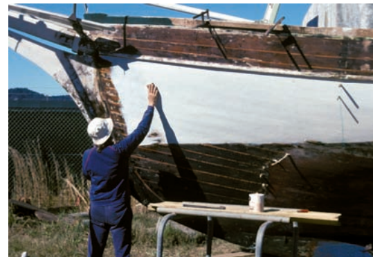
Alan Lucas, left, fitting a new knee. Renee had no hanging knees either in the cabin or sidedeck construction. This one was laminated from strips of oak.
