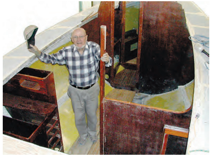
After assessing the boat's overall condition, Stephen decided there was nothing to do but remove everything from inside the hull, at left. By the time his father came to visit, at right, Stephen had begun reassembling the interior. The yellow color is the Kevlar laminate he added.
