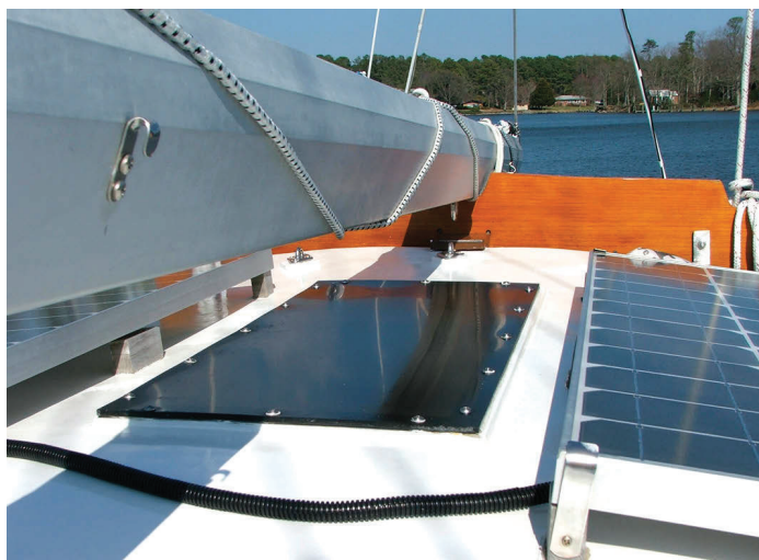
A Lexan panel in the top of the wheelhouse sends light inside and makes the mainsail visible from the helm, at left. Solar panels are installed on both sides of the Lexan. The dinghy gets to look at its reflection in the hull after the most recent hull-painting, at right.
