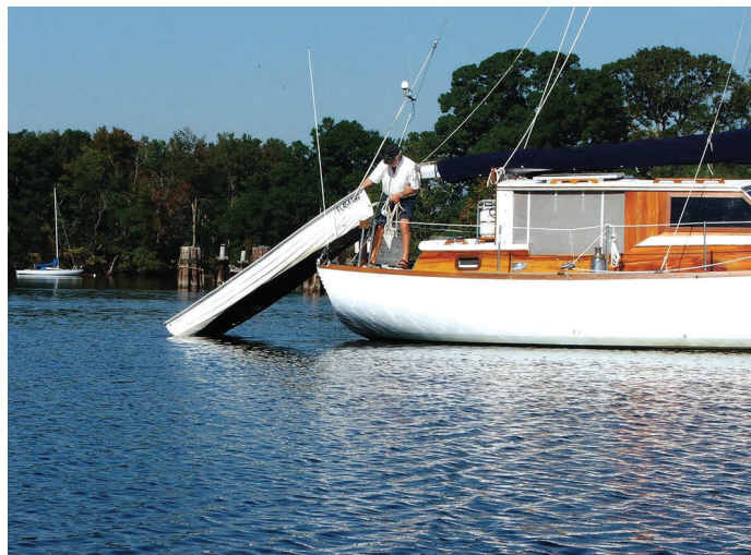
A split backstay allows the dinghy to be carried on top of the aft cabin. David hoists the dinghy over the transom, at left, then secures the dinghy to a sturdy cleat on the boom gallows, at right. The two backstays prevent the dinghy from shifting side-to-side when sailing.
