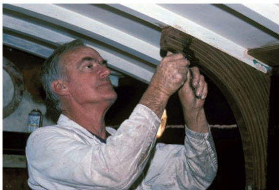
Alan Lucas, left, fitting a new knee. Renee had no hanging knees either in the cabin or sidedeck construction. This one was laminated from strips of oak.
