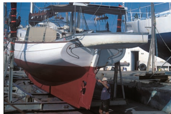
Reminiscent of the Herreshoff shape, Renee's stern sections, below, resolve into tumblehome and champagne-glass transom. She was designed in the 1950s by Hugh Angelman and Charles Davies.
