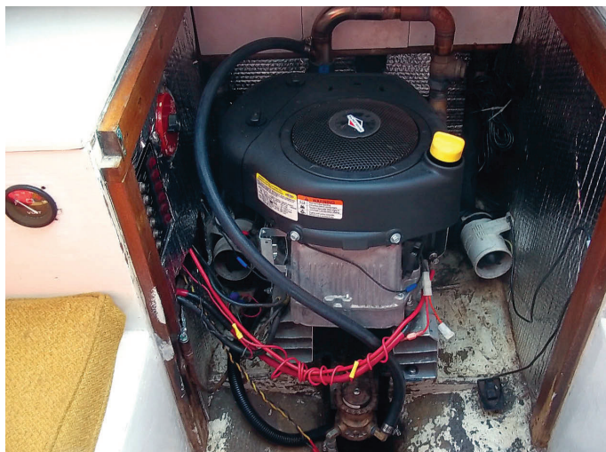
The motor in the Pacific 30, at left, turned out to be a Baldwin — an Evinrude outboard modified to drive a conventional prop shaft. Peter had it working with a new (old) powerhead but eventually replaced it with a Briggs & Stratton air-cooled lawn mower engine, at right.
