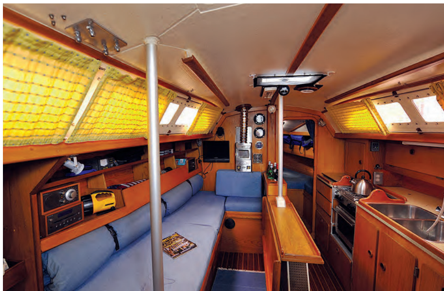
Rob opened up CanCan 's interior to run new electrical wiring and plumbing, at left. He added amenities including a cabin heater and new stove, below, and fitted fridge/freezers into the cabinets. Note the trunk for the swing keel that allows the boat to be beached.
