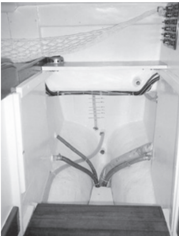
Atom's head, at top, showing the Lavac toilet behind a watertight bulkhead. And the former engine compartment, above, showing the watertight cockpit locker drain hoses (shutoff valves are located under main cabin floorboard) and integral water tank built between the hull and cockpit floor.
