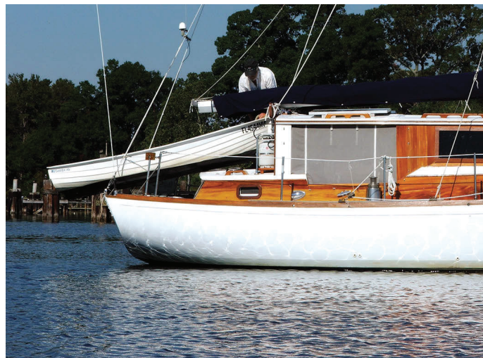
A split backstay allows the dinghy to be carried on top of the aft cabin. David hoists the dinghy over the transom, at left, then secures the dinghy to a sturdy cleat on the boom gallows, at right. The two backstays prevent the dinghy from shifting side-to-side when sailing.
