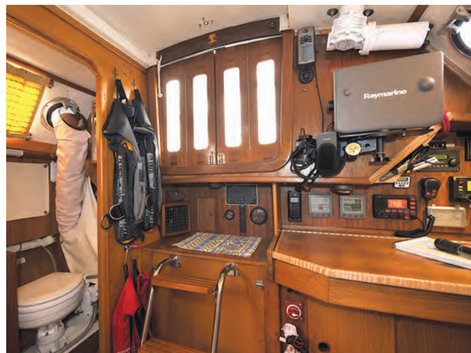
CanCan has a large interior for a 28-foot boat. The sleeping cabin is forward, at left, and the aft end of the main cabin, at right, is devoted to the head, to starboard, and the nav station, to port. The wrapped duct in the head is part of Rob's "air-to-air" air conditioning system.
