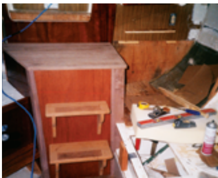
Dave fitted a small chart desk into the space on the port side next to the new engine box.
