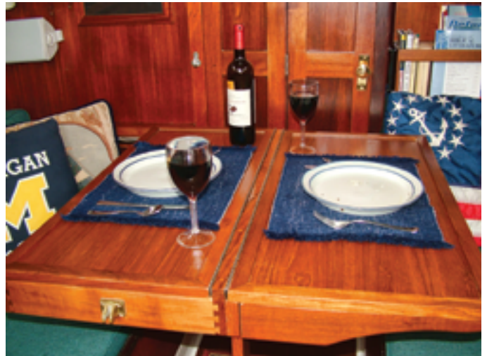
Dave had a table custom made for Scholarship II . When not in use, it folds up against the main bulkhead to open up the saloon, at left. It serves as the dining table, at right, and also as the chart table.
