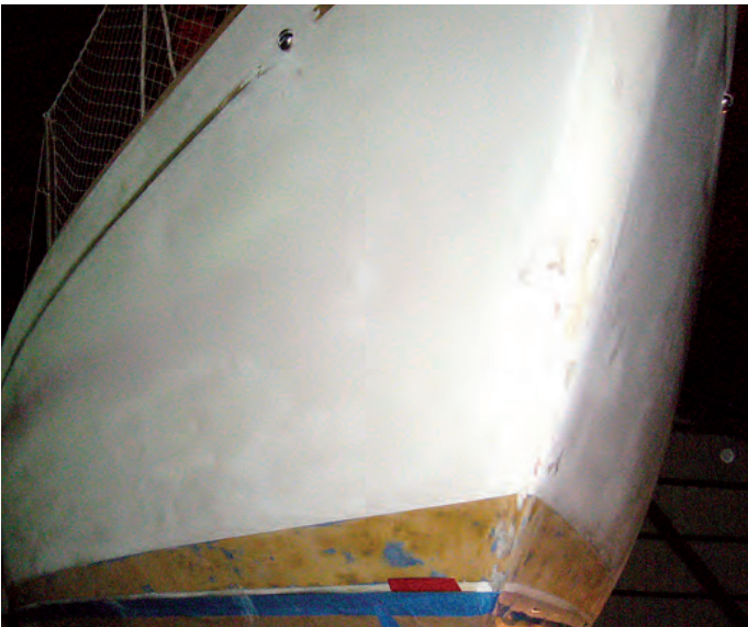
Nobody liked the "blah" off-white hull color so, over their first winter with the boat, E-J and Tim stripped the bootstripe and spent 80 hours sanding the hull, at left. The deep blue and the red bootstripe certainly banished the blahs, at right.
