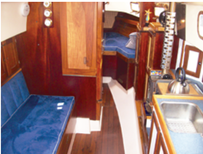
By applying mahogany to the saloon bulkhead and renewing the upholstery, Dave brought the decor up to date, at left. New cane-front lockers give the forward cabin a fresh look and the cabin heater will make the whole boat cozy in spring and fall, at right.
