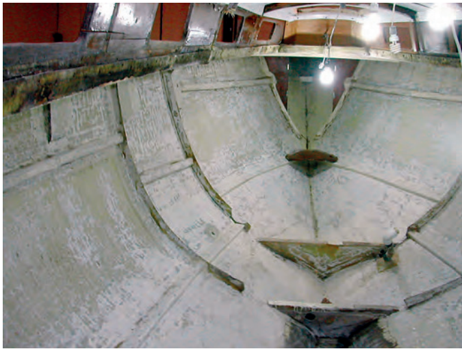
After assessing the boat's overall condition, Stephen decided there was nothing to do but remove everything from inside the hull, at left. By the time his father came to visit, at right, Stephen had begun reassembling the interior. The yellow color is the Kevlar laminate he added.
