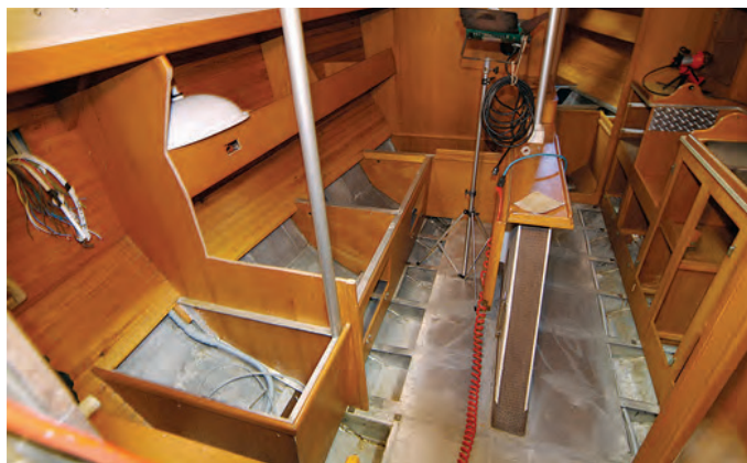
Rob opened up CanCan 's interior to run new electrical wiring and plumbing, at left. He added amenities including a cabin heater and new stove, below, and fitted fridge/freezers into the cabinets. Note the trunk for the swing keel that allows the boat to be beached.
