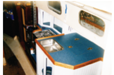
The new galley counter provides a large work surface and encloses an Igloo cooler.
