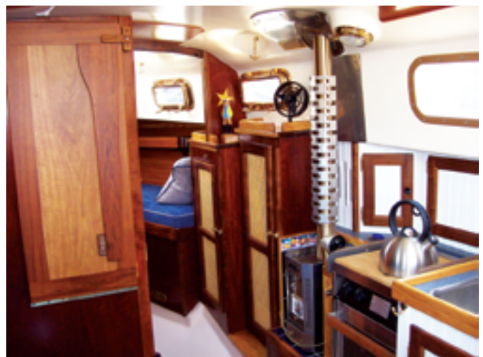
By applying mahogany to the saloon bulkhead and renewing the upholstery, Dave brought the decor up to date, at left. New cane-front lockers give the forward cabin a fresh look and the cabin heater will make the whole boat cozy in spring and fall, at right.
