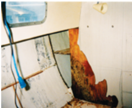
Leaks around the chainplates led to water damage to the main bulkhead.
