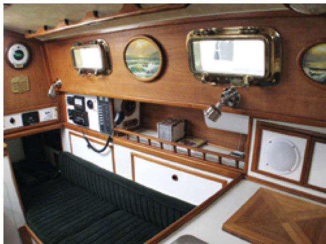
The galley-forward layout on the Voyager 26 is not fashionable today but, in a boat of this size, it uses the width in a practical way, at left. On the port side, aft of the sink, the settee berth doubles as a navigator's seat. The bronze portlights add a big-ship touch, at right.
