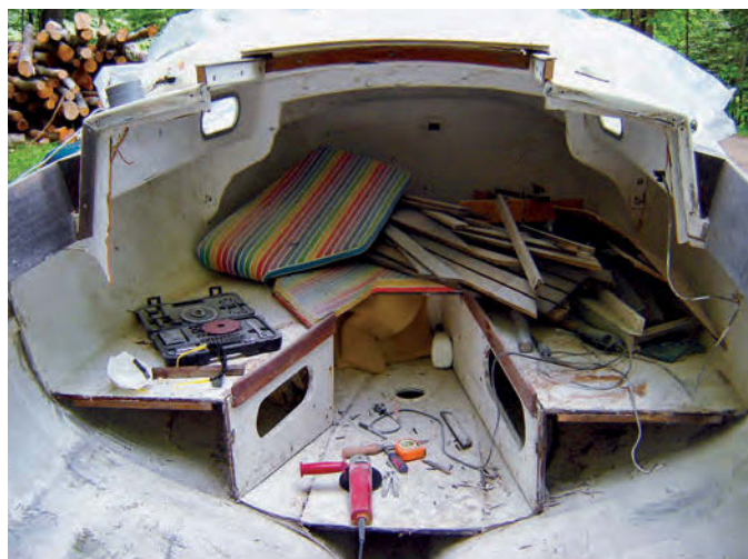
By the time Kegan had removed all the decayed wooden parts, the boat was looking rather bare, at left. At last reconstruction began, with the base for the main bulkhead, at right.
