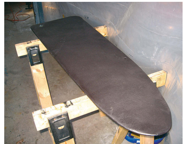
Nathan had a metalworking shop sandblast the centerboard. He then coated it with POR-15 rust-preventive paint and epoxy barrier coats and faired it, using wax paper to wrap and form fairing compound around the edges, at left. Two coats of bottom paint, at right, finished the job.
