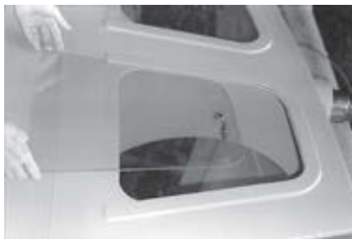
Dabbler's removable, waterproof, polycarbonate windows.
