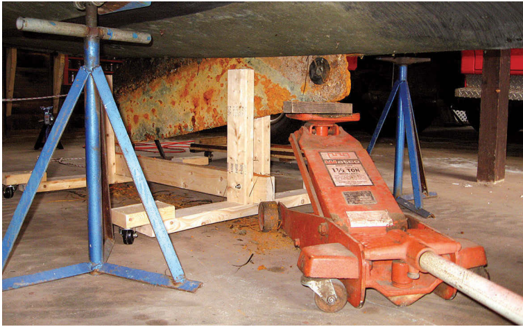
The 165-pound centerboard was covered in rust and presented a challenge. However, Nathan's ingenuity in building a trolley on casters, and muscle in the form of a floor jack, at left, enabled him to extract it and move it around for sandblasting and painting, at right.
