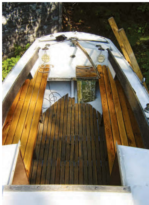
With new cockpit seats and the sole refinished, Occam's Razor began to look like a proper yacht once more.
