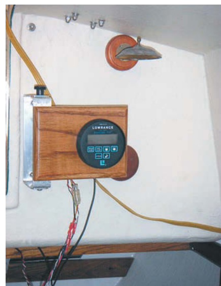
The new compression beam installed, at left above; the new switch panel and automatic bilge pump switches, at right above. The GPS gets a new mounting bracket, at left; and the depth sounder in its new swing-away bracket, at right. Facing page: the new combination mast light, at top; the Vire 7 engine, at left; and the workings of the engine compartment — the water pump, muffler, and prop shaft — at right.
