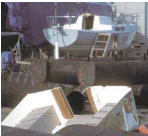
The cockpit gets cut out, above. Dave rides it to the dump, below left. The hull is gutted, below right, and gets sanded back to clean fiberglass.
