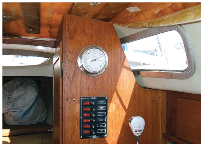
A view of the starboard side shows the former sad state of the overhead liner and the bulkhead, at left. A similar view after Ken completed the work, at right, shows the new teak veneer covering the blemishes on the bulkhead and fresh varnish elsewhere. The new overhead is in place, fastened to fore-and-aft stringers with screws and trim washers, and Ken's clock and barometer from a previous boat adorn the port bulkhead.
