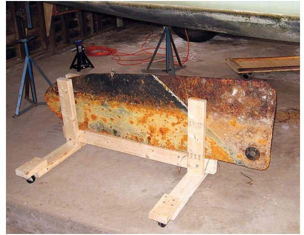
The 165-pound centerboard was covered in rust and presented a challenge. However, Nathan's ingenuity in building a trolley on casters, and muscle in the form of a floor jack, at left, enabled him to extract it and move it around for sandblasting and painting, at right.
