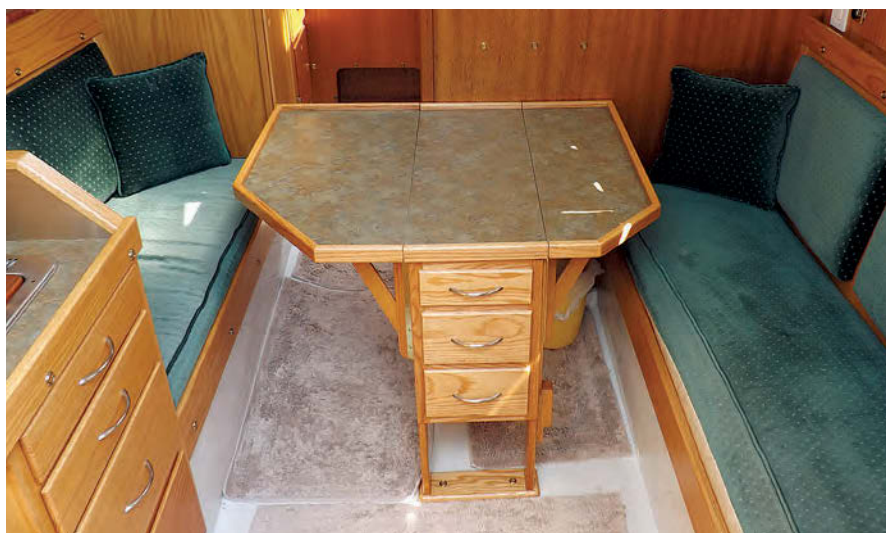
The saloon table has drawers built into its base and a support for the extending starboard settee berth.
