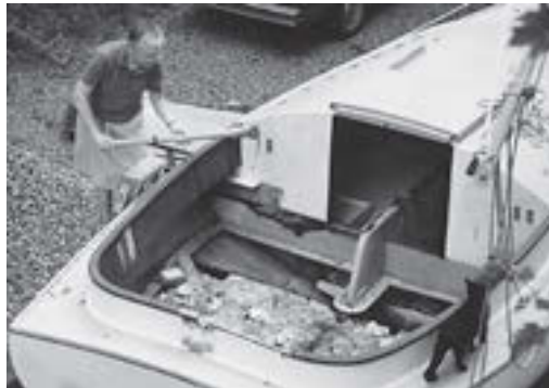
Demolition: out come 200 pounds of rotten and waterlogged cockpit.
