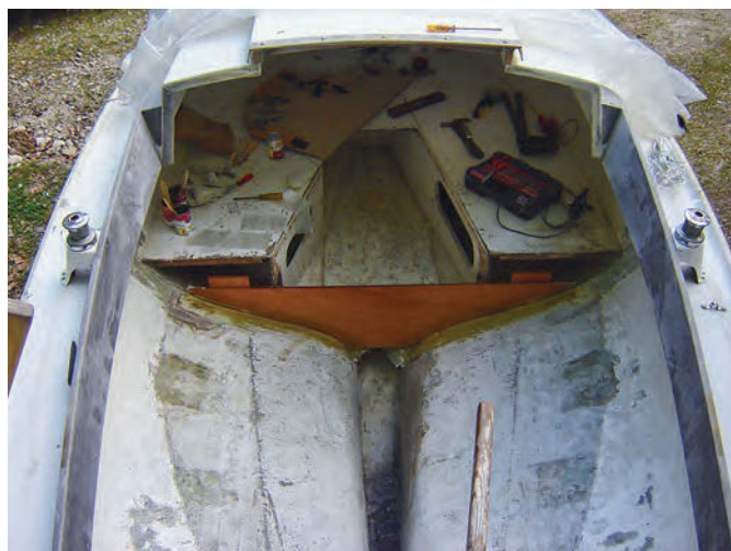
By the time Kegan had removed all the decayed wooden parts, the boat was looking rather bare, at left. At last reconstruction began, with the base for the main bulkhead, at right.
