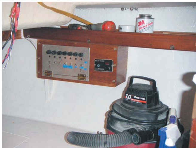
The new compression beam installed, at left above; the new switch panel and automatic bilge pump switches, at right above. The GPS gets a new mounting bracket, at left; and the depth sounder in its new swing-away bracket, at right. Facing page: the new combination mast light, at top; the Vire 7 engine, at left; and the workings of the engine compartment — the water pump, muffler, and prop shaft — at right.
