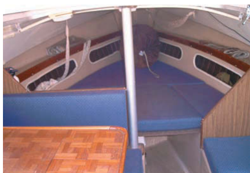
Bonita's interior — once full of 18 inches of green, slimy water and the accumulated dirt of many years of neglect — was vastly improved with the help of Windex (removes algae), a thorough scrubbing, and new cushions.
