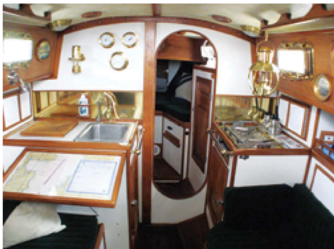
The galley-forward layout on the Voyager 26 is not fashionable today but, in a boat of this size, it uses the width in a practical way, at left. On the port side, aft of the sink, the settee berth doubles as a navigator's seat. The bronze portlights add a big-ship touch, at right.
