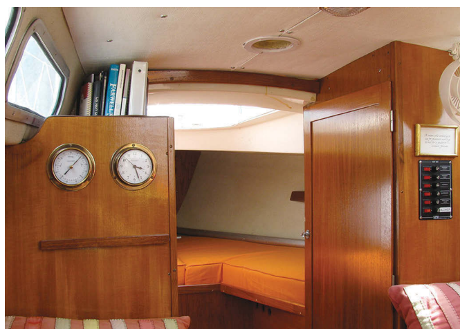
A view of the starboard side shows the former sad state of the overhead liner and the bulkhead, at left. A similar view after Ken completed the work, at right, shows the new teak veneer covering the blemishes on the bulkhead and fresh varnish elsewhere. The new overhead is in place, fastened to fore-and-aft stringers with screws and trim washers, and Ken's clock and barometer from a previous boat adorn the port bulkhead.
