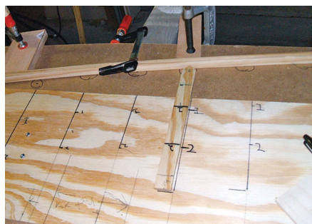
Ken used scrap lumber to hold pieces of the old overhead liner in place while the adhesive set, at left. Using tick stick marks and a flexible batten, he drew the shapes of the new overhead liner on hardboard, center, then screwed the hardboard patterns in place and marked them for trimming, at right.
