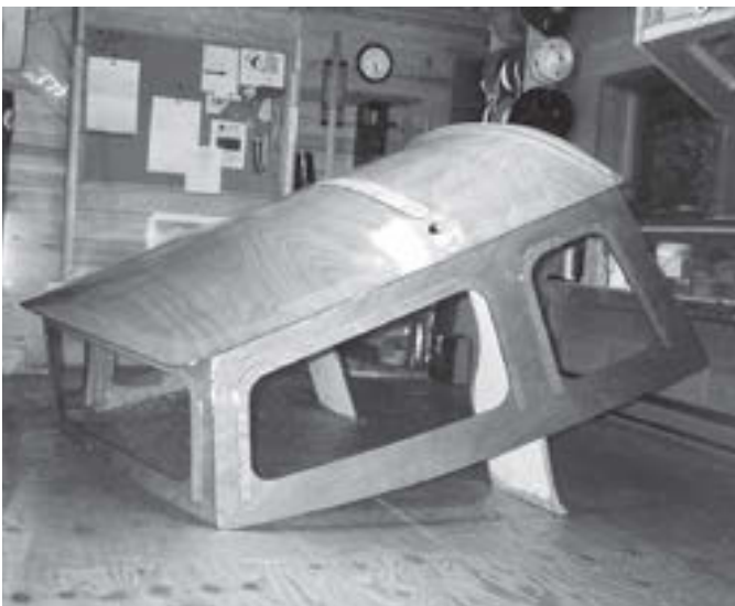
The new cabintop takes shape in the sail loft.
