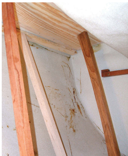
Ken used scrap lumber to hold pieces of the old overhead liner in place while the adhesive set, at left. Using tick stick marks and a flexible batten, he drew the shapes of the new overhead liner on hardboard, center, then screwed the hardboard patterns in place and marked them for trimming, at right.
