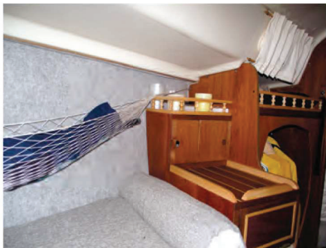
Adding the vanity in the forward cabin, at left, made living aboard easier and hardly affected use of the V-berth, which is too small for two anyway, at center. Behind the new carpeting on the hull sides is a layer of insulation. The rail that supports the bed slats is visible on the settee front, at right. More of Dan's shelves can be seen above the settee back.
