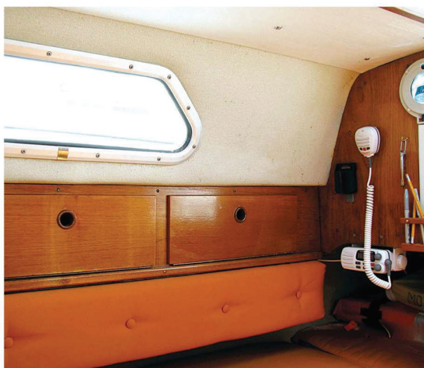
The Nu-Teak sole brightened up the interior and gave the job a final touch, far left. Ken finished the curved hull sides with Ultra Tuff non-skid. The new material on the overhead closely matched the old material on the coachroof sides, at left.
