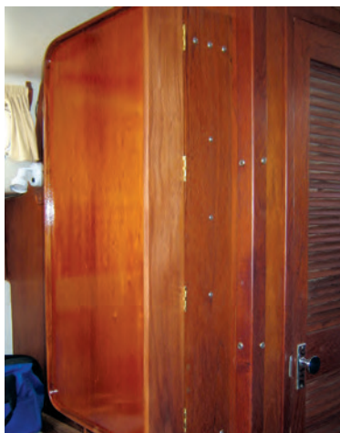
Sundew's new table, above left, folds against the bulkhead, where a hinged flap holds it in place, above center. Jim's flexible shower grating is a work of art, above right. Granite counters brightened up the galley, below left and center, and the head, below right.
