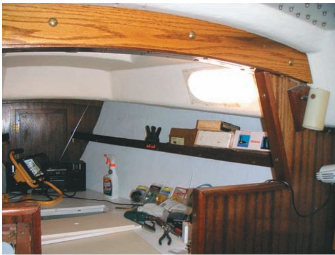
The new compression beam installed, at left above; the new switch panel and automatic bilge pump switches, at right above. The GPS gets a new mounting bracket, at left; and the depth sounder in its new swing-away bracket, at right. Facing page: the new combination mast light, at top; the Vire 7 engine, at left; and the workings of the engine compartment — the water pump, muffler, and prop shaft — at right.
