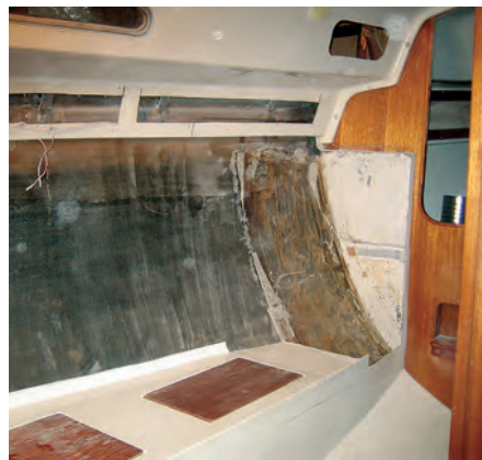
The saloon originally had some white surfaces and open storage shelves behind the settees, at left. Ken began his refit of Reinsnest by removing much of the saloon furniture, center. He also took out the V-berth, built a new holding tank into the hull beneath it, at right, and fitted a water tank on top of that.
