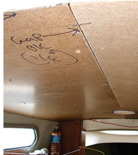
Ken used scrap lumber to hold pieces of the old overhead liner in place while the adhesive set, at left. Using tick stick marks and a flexible batten, he drew the shapes of the new overhead liner on hardboard, center, then screwed the hardboard patterns in place and marked them for trimming, at right.
