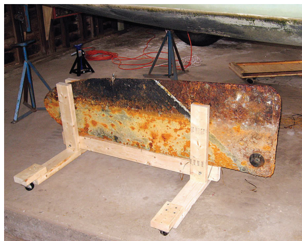
The 165-pound centerboard was covered in rust and presented a challenge. However, Nathan's ingenuity in building a trolley on casters, and muscle in the form of a floor jack, at left, enabled him to extract it and move it around for sandblasting and painting, at right.
