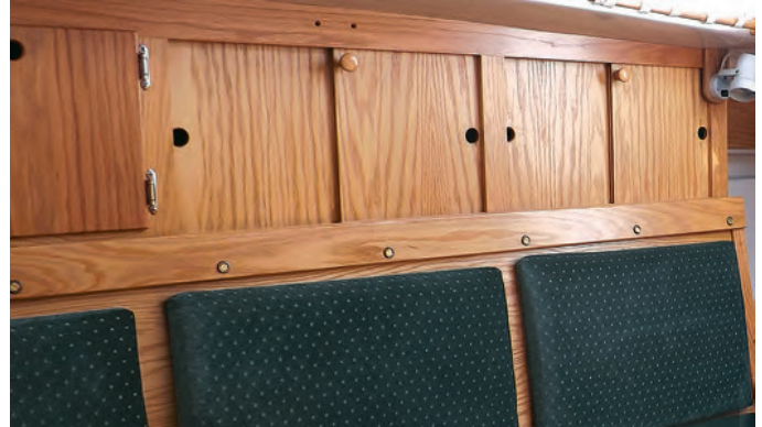
Ken shortened the port-side settee and extended the galley forward, at left. He made his new cabinets and furniture of red oak for its light color. On the port side, Ken fitted lockers behind and above the seat backs, at right. The seat-back cushions are attached to panels that lift up and out to give access to the lockers.
