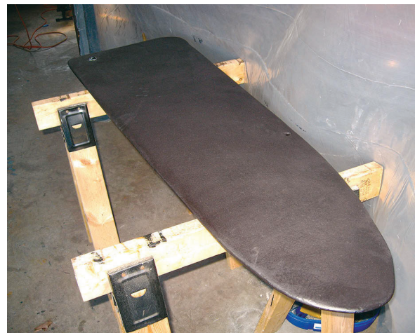
Nathan had a metalworking shop sandblast the centerboard. He then coated it with POR-15 rust-preventive paint and epoxy barrier coats and faired it, using wax paper to wrap and form fairing compound around the edges, at left. Two coats of bottom paint, at right, finished the job.
