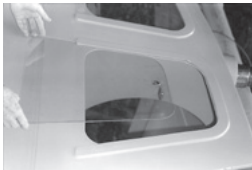
Dabbler's removable, waterproof, polycarbonate windows.
