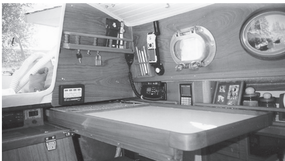
The nav station slides out from the quarterberth area when needed. It occasionally doubles as a table for indoor dining.
