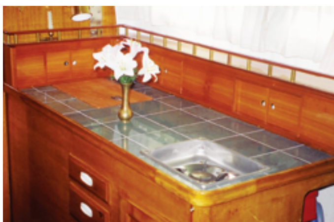
The Cal 25's galley was basic, above left. Chris removed the stove and mocked up cabinets to surround the countertop, above right. The finished galley, with its tiled top, glows, at left.
