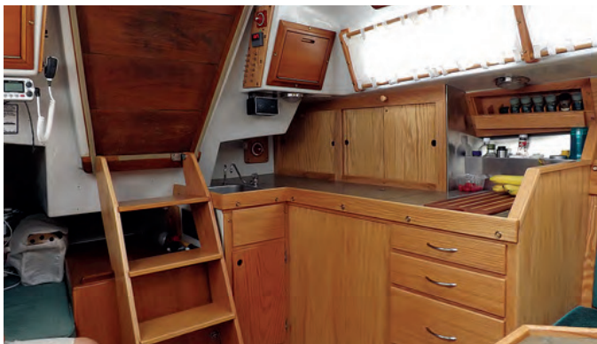
Ken shortened the port-side settee and extended the galley forward, at left. He made his new cabinets and furniture of red oak for its light color. On the port side, Ken fitted lockers behind and above the seat backs, at right. The seat-back cushions are attached to panels that lift up and out to give access to the lockers.
