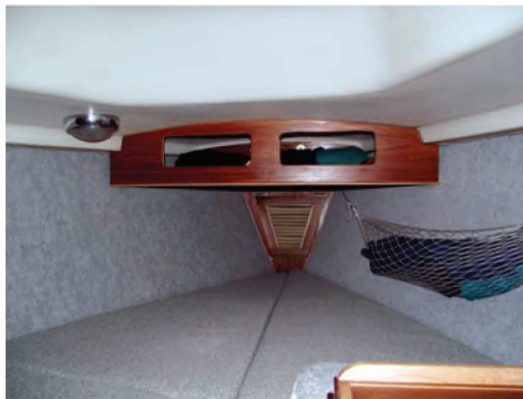
Adding the vanity in the forward cabin, at left, made living aboard easier and hardly affected use of the V-berth, which is too small for two anyway, at center. Behind the new carpeting on the hull sides is a layer of insulation. The rail that supports the bed slats is visible on the settee front, at right. More of Dan's shelves can be seen above the settee back.
