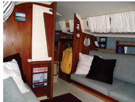
Adding the vanity in the forward cabin, at left, made living aboard easier and hardly affected use of the V-berth, which is too small for two anyway, at center. Behind the new carpeting on the hull sides is a layer of insulation. The rail that supports the bed slats is visible on the settee front, at right. More of Dan's shelves can be seen above the settee back.
