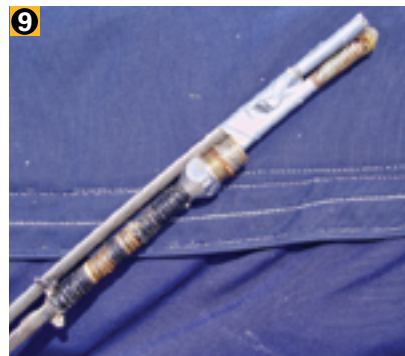
9 Tape the old wire, with the wedge still in place, to the new wire.
