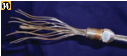
Slip the socket over the end of the new wire and unlay the strands.
