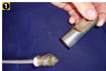
1 The first step in disassembling a terminal is to unscrew the two parts.
