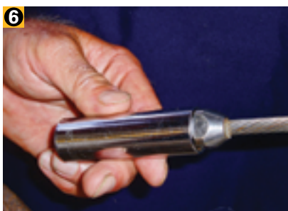
6 The socket should rest up against the hex end of the terminal socket.
