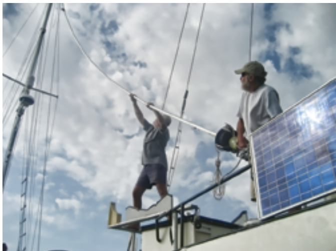
The team on RDreamz , at left, walked forward on deck carrying Carina's furling drum while supporting the extrusion to clear the stern rail as it came down. Leslie and Philip labeled the components as they carefully dismantled and inspected the Profurl furling assembly, at right.
