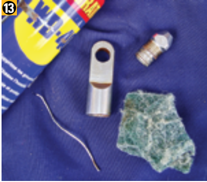
Clean both threaded parts of the terminal before reusing them.
