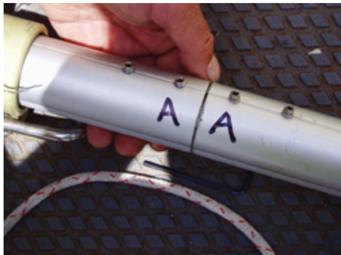
The team on RDreamz , at left, walked forward on deck carrying Carina's furling drum while supporting the extrusion to clear the stern rail as it came down. Leslie and Philip labeled the components as they carefully dismantled and inspected the Profurl furling assembly, at right.
