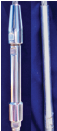
Hi-Mod terminals use a "crown ring," far left. An assembled Hi-Mod alongside a swaged fitting, at left. In the Quick Attach (and the similar Blue Wave) terminals, above, the wedge fits over the entire wire.
