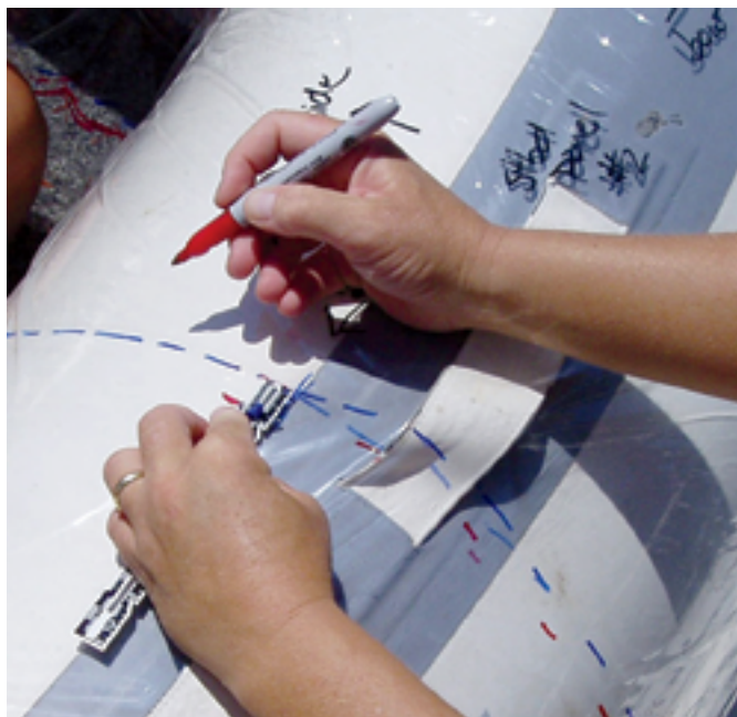
Use a small metal ruler with an adjustable reference to rapidly label a panel cut line relative to a seam line, at left. Use small pieces of duct tape to secure clear plastic patterning material to the dinghy for a snug fit, above.
