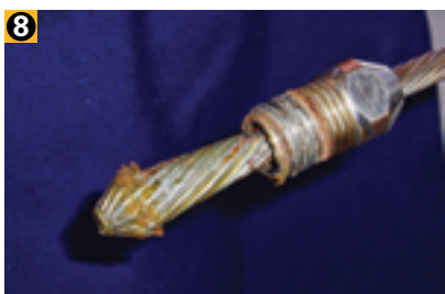
8 The terminal socket slides up the wire revealing the sealant inside.
