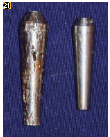
The corroded wedge (left) indicates water ingress into a terminal.
