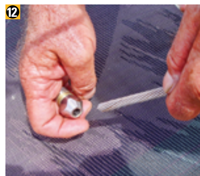
12 Slide the terminal socket off the cut end of the old wire.
