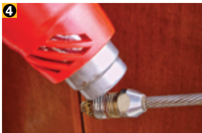
4 If sealant was used in assembling the terminal, soften it with a little heat.
