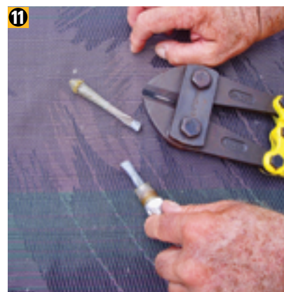
11 To remove the terminal socket from the old stay, cut the wire.
