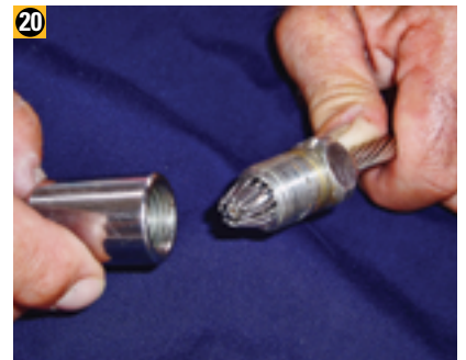
Make the final assembly with sealant and thread-locking compound.
