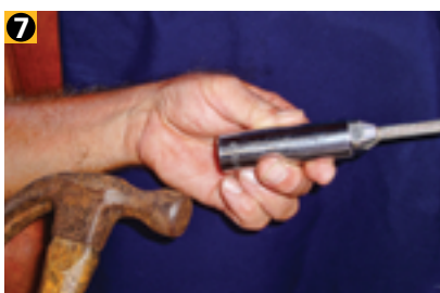
7 Tap the end of the socket with a hammer to loosen it from the wedge.
