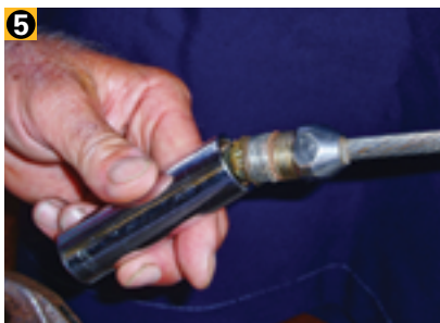
5 Select a long socket that will just fit over the end of the terminal.
