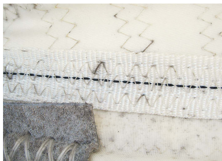
Mildew, which often appears as black specks, degrades sailcloth biologically.
