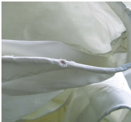
Look for damage along the leech, where chafe on rigging can expose the leech line.
