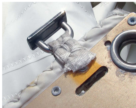
UV light from the sun is an unrelenting cause of sail damage, degrading everything from stitching, upper image, to the webbing seizings on sail slides, above.
