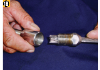
Thread the female terminal end onto the socket and draw it up hand tight.
