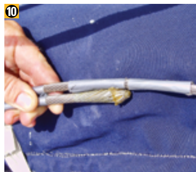
10 At the other end, wrap tape around the new wire and mark for the cut.
