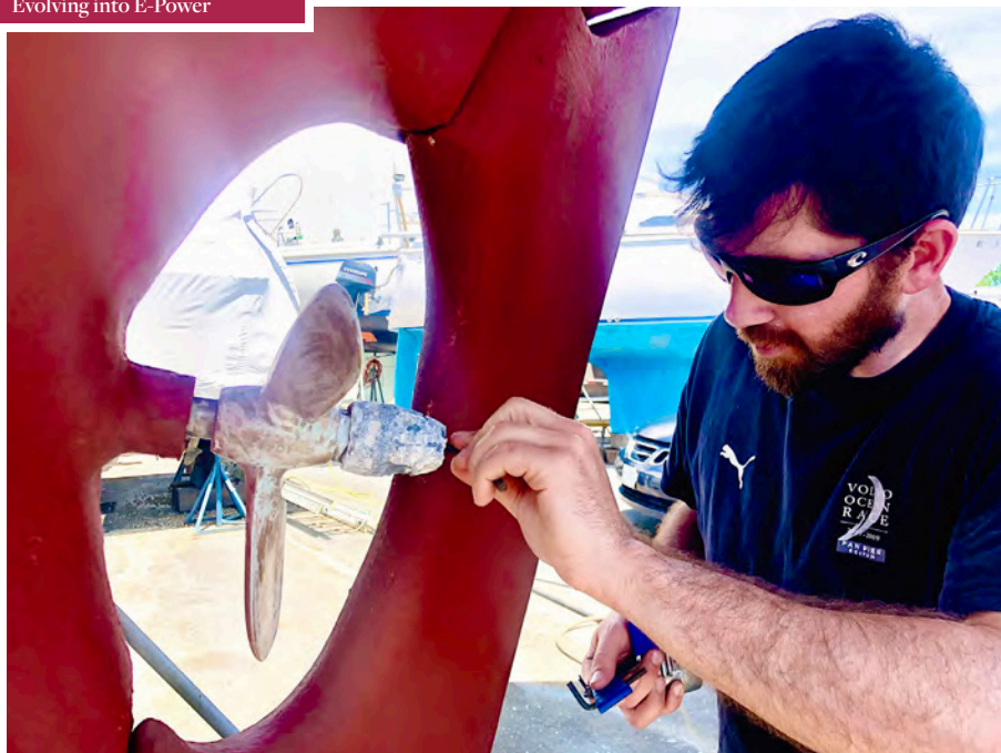
Adam performs some annual maintenance on the propeller, replacing the zinc and applying a new coating of Prospeed.
