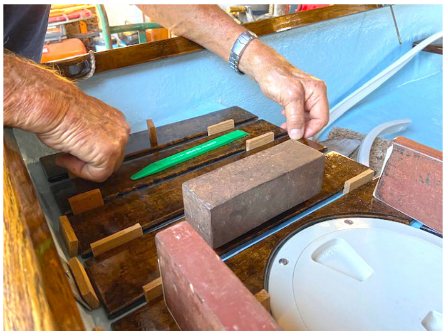
Bricks and spacers were used to ensure the slats for the aft seat were in the proper place.
