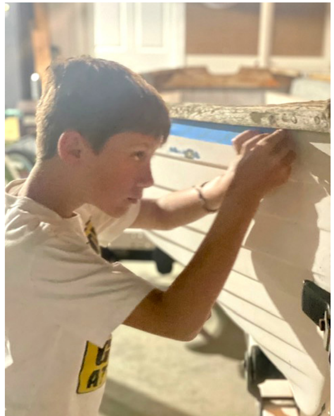
Taping the hull to prepare the gunnel for sanding and varnish.
