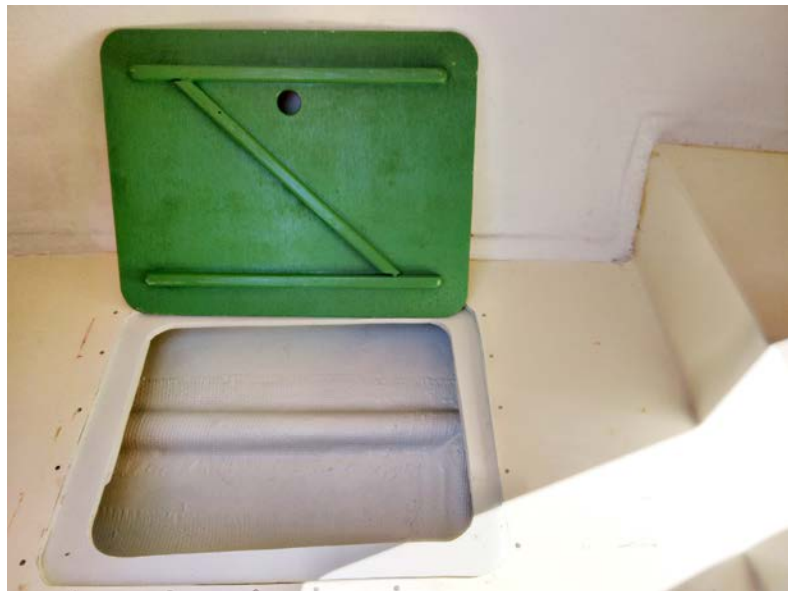
A lift-off hatch and interior bulkhead were added to the starboard quarter berth to make a stowage compartment.
