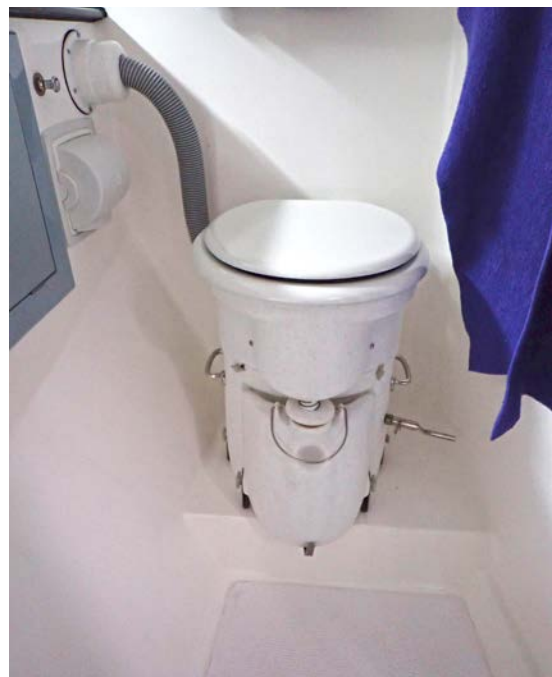
An Air Head on a Rapido 40 trimaran, which has the advantage of being a low-weight unit.
