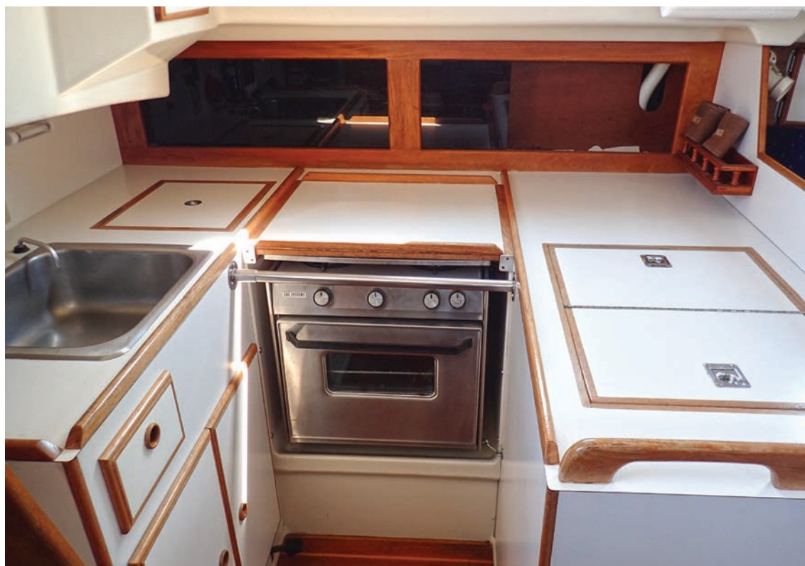
The original galley layout of the Pearson 365 included a small, 9-inch sink and adjacent deep storage cabinet.
