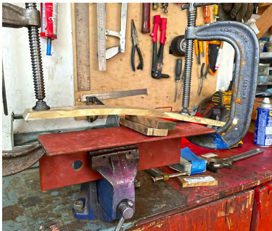
The author cold-bent the shroud chainplates on a simple homemade jig.
