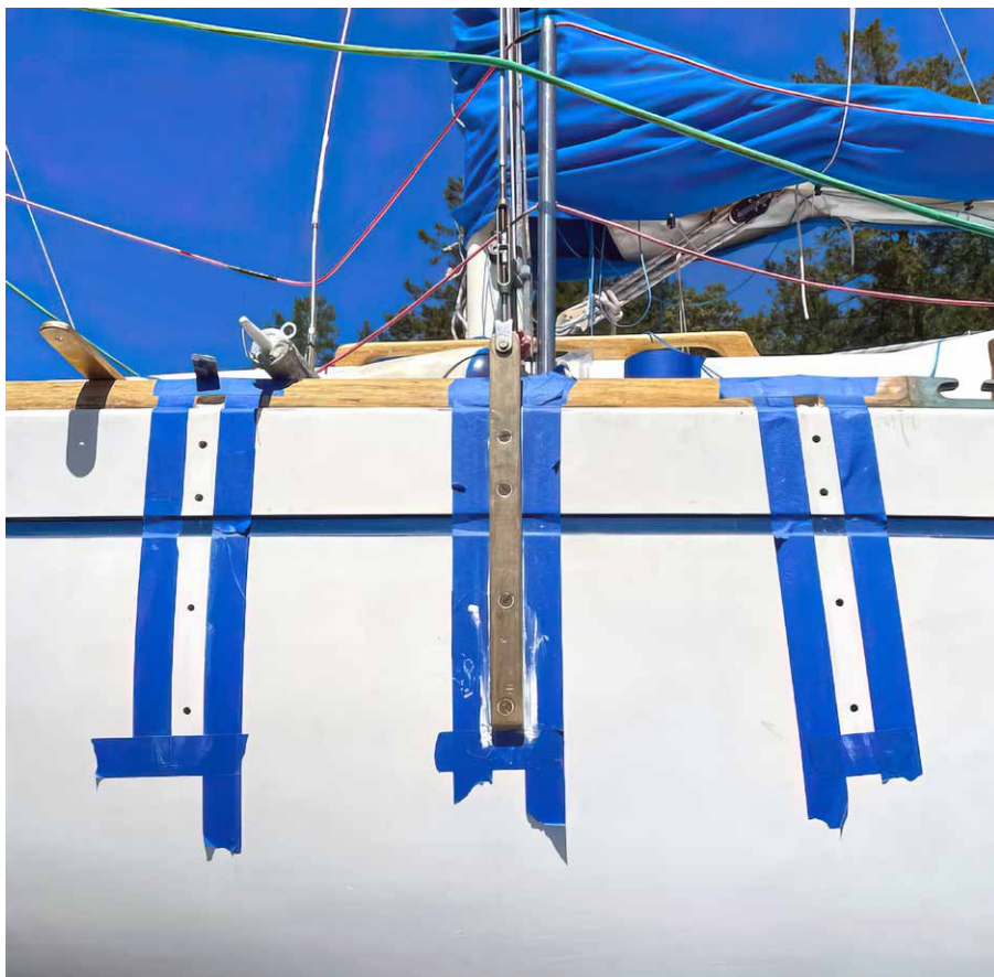
Left, installation day. The top shroud chainplate is fully installed and the lower shroud ones are almost ready to be glued.
