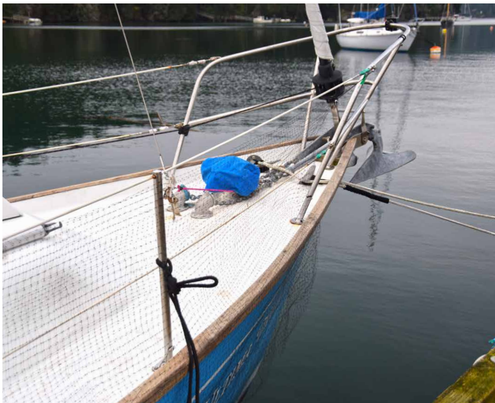
Essential sail handling and ground tackle gear are all accommodated at the bow. Note the termination of the inner forestay. Photo by Bert Vermeer.
