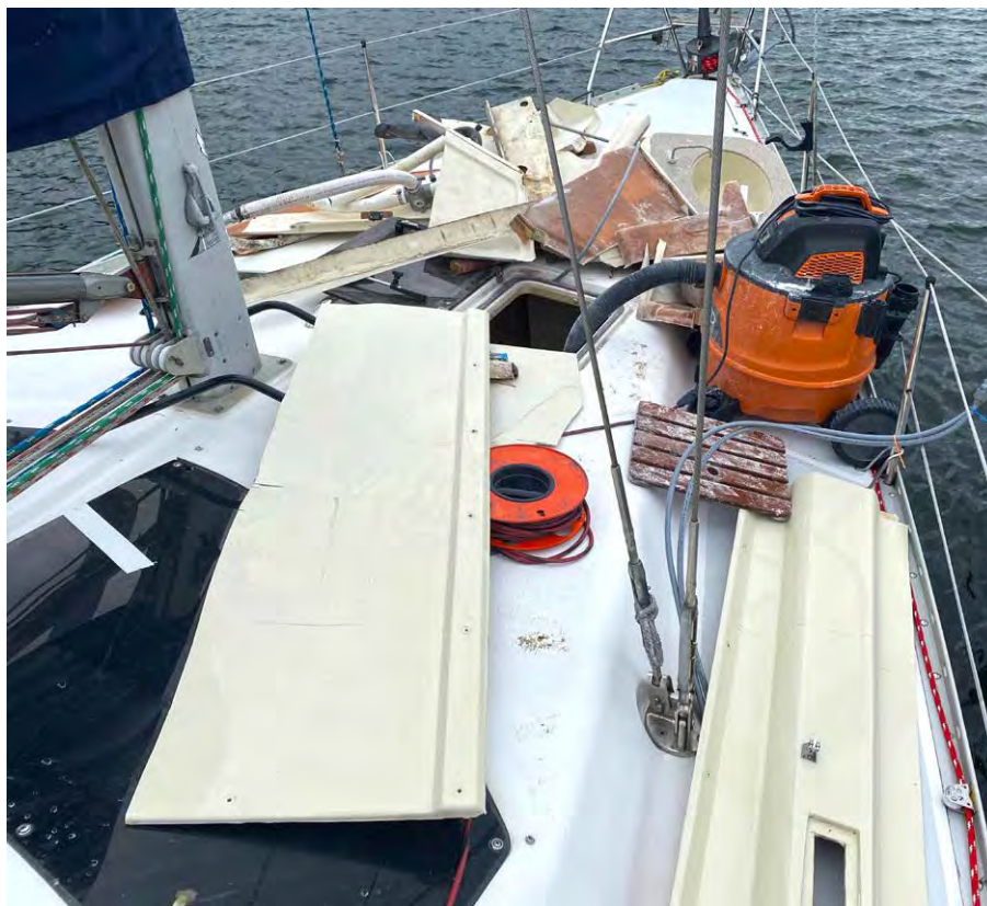
Bathroom remnants up on deck, with the vacuum hose hanging down through the hatch to minimize fiberglass dust.
