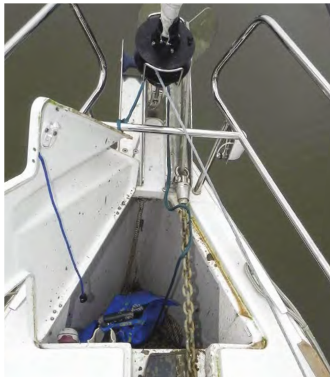
The bow area is configured for two anchor rollers, stowage, and a windlass concealed by the hatch cover — all very clean.
