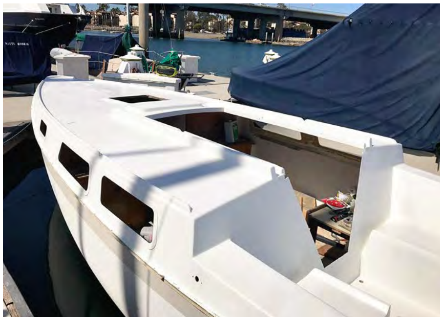
One More Time midway through the restoration, with the deck and cockpit repaired and repainted, still awaiting deck hardware, new portlights, and a new companionway slider, at right.
