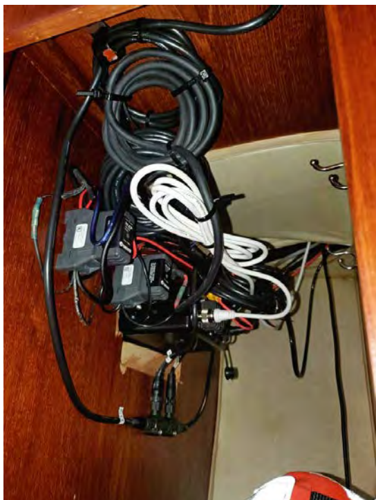
The two rectangular black devices are transient voltage surge suppressors (TVSS), which Drew installed in-line; they disconnect a circuit in the case of a sudden and large power surge.
