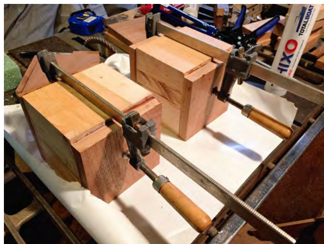
The two new pedestals glued and clamped together, above.
