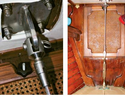
Below, Ed added a robust deck plate under the foredeck with an eye to accept a turnbuckle and wire (at left) that transfers the load to the foremost interior bulkhead, which is glassed to the hull. (at right).
