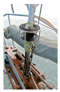
In the forward position, the stay is attached to a permanent toggle installed in the stemhead fitting's aft-most opening. The stay is just clear of the furling drum and allows for easy hoisting and lowering of sails.
