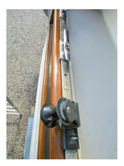
When not needed, the inner stay is attached to the starboard center stanchion, held securely by a small 1/4-inch turnbuckle. This allows enough tension to remove the slack so the stay does not flop around and can be reasonably secure if grabbed in a pinch, above left.
