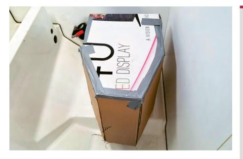
To ensure the optimum placement for the C-Head, Jerry first made and installed a cardboard mock-up.
