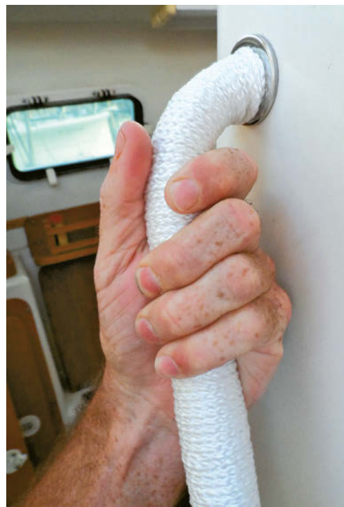
Wrapping a stainless steel handhold with thin line gives you much firmer grip, below.
