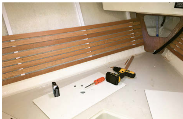
Starting at the bottom of the hull side and working his way up to the top, Bert attached 1¼ x ¼-inch oak strips, finished with satin varnish, to the cedar ribs using small wood screws and finishing (cup) washers.
