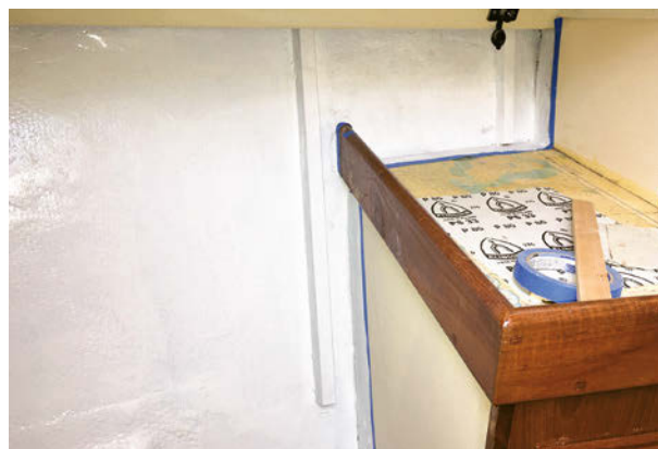
Once the cedar ribs were in place, everything got a coat of white primer to provide a clean background.
