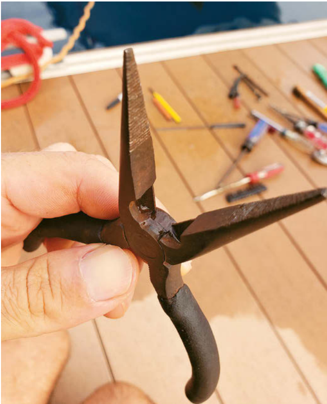
A dab of oil, followed by exercising the hinge, keeps these needle-nose pliers in good working order.
