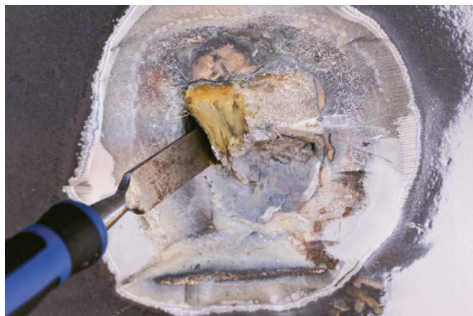
Chiseling out the filler, Robin had to be careful not to damage the bolt threads.
