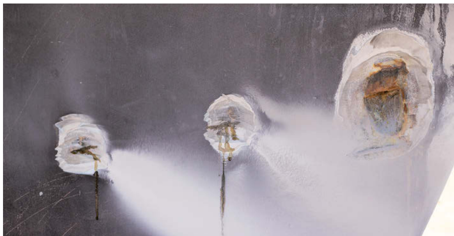
Telltale weeping on MonArk's keel (post grinding) illuminates the keel bolt problem.
