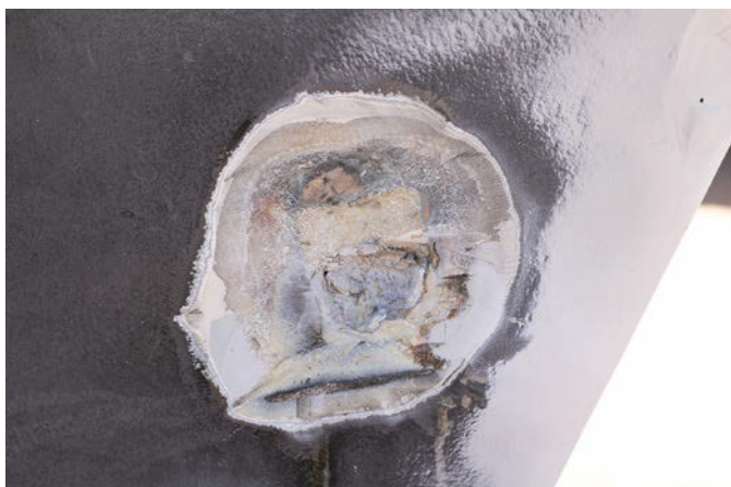
The keel pockets are exposed after being ground out.
