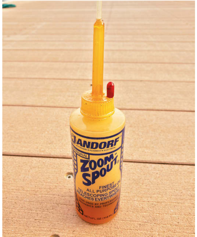
This handy container has a long, thin spout that lets Zachary apply just the right amount of oil to keep his tools limber and corrosion-free.
