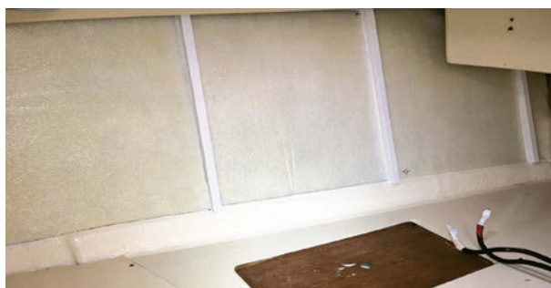
Bert glued in ½-inch sheets of closed-cell foam to prevent the hull sides from sweating in the damp Pacific Northwest climate.
