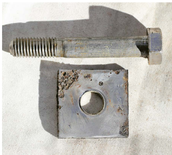
A keel bolt and old washer; note the pitted metal in the latter.
