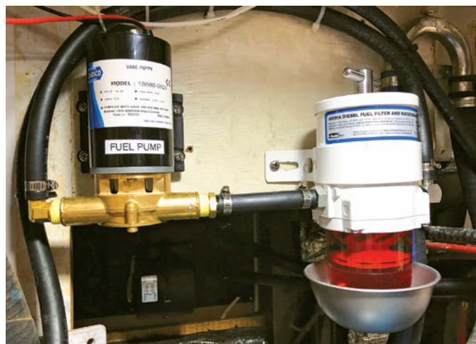
The Jabsco Vane Puppy pump (left) draws fuel through the primary fuel filter (right), which Gino opted to upgrade during this project to a Racor 500 with a 10-micron filter element.
