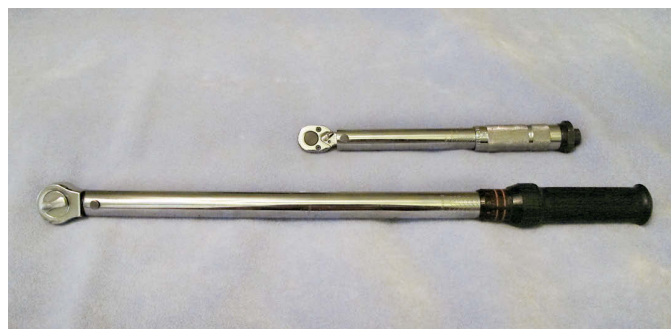
The click wrench is more accurate and reliable than the beam wrench. These two, above, are sized and calibrated for different ranges of torque, the smaller in inch-pounds and the larger in foot-pounds.
