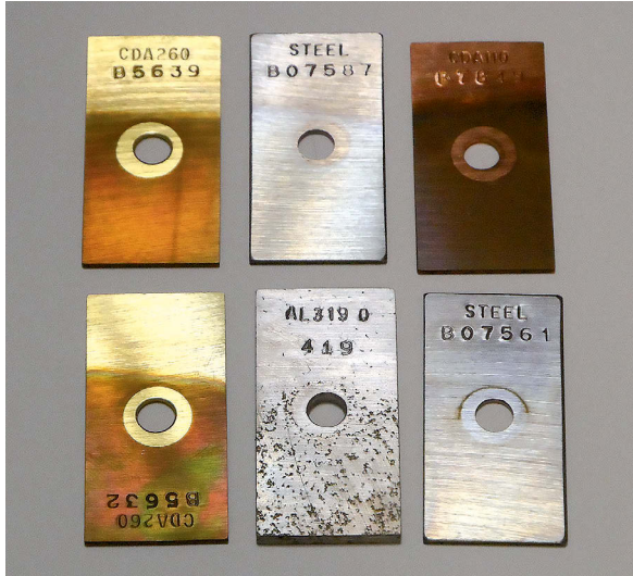
In another sample, there was corrosion on the coupons and the gasoline was visibly darkened by oxidation and sludge formation.
