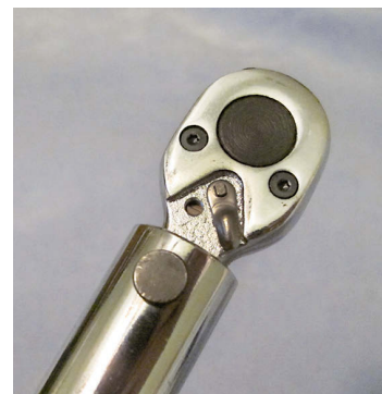
The click wrench is more accurate and reliable than the beam wrench. These two, above, are sized and calibrated for different ranges of torque, the smaller in inch-pounds and the larger in foot-pounds.
