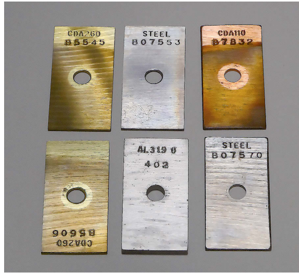
After 2 months, the best-performing anti-corrosion additive left the gasoline clear and the test coupons corrosion-free.
