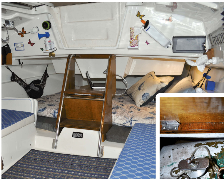
On the MacGregor 26, the water-ballast controls are under the companionway. The stainless steel handle is for the ballast entry and discharge valve and the bronze-colored handle is the vent plug.
