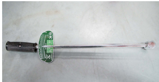
The beam wrench is not expensive, nor is it very accurate. Because the user must watch closely for the pointer to reach the desired torque on the scale, errors are possible.
