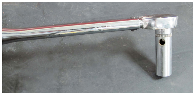
Crowfoots, extensions, and adapters, above upper, should be avoided, as they flex, twist, and slip, seriously reducing torque and compromising accuracy.
