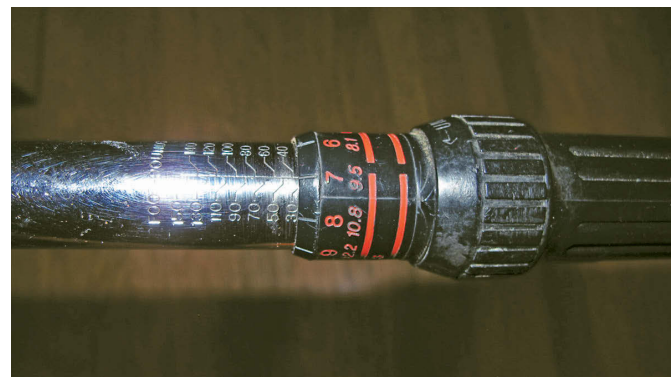
This wrench is set to 27 foot-pounds or the metric equivalent of 9.5 newton meters. A locking handle is important to prevent changes while tightening.
