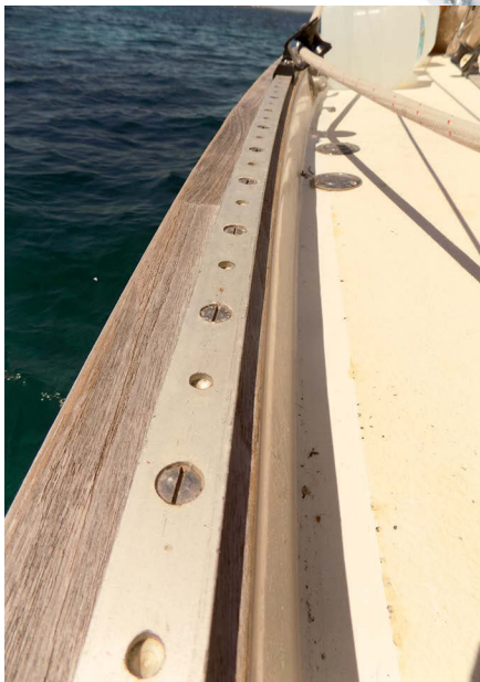
Trouble awaits should the slotted screws securing this genoa track need removing.
