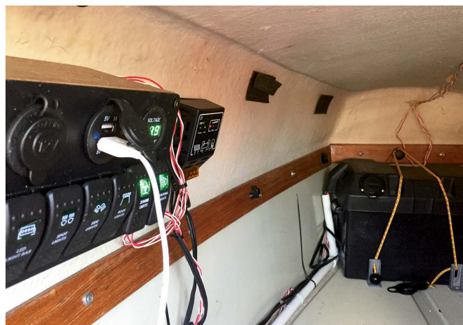
Robert usually daysails his Harpoon 5.2 on a lake, so he had to make some modifications before taking on the Texas 200. They included building a platform for his bed, at left, and installing an electrical system, at right, for navigation lights and chargers for digital devices.
