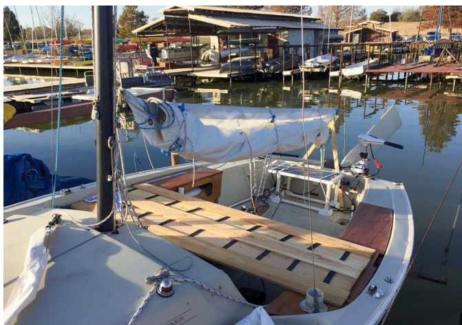
Robert usually daysails his Harpoon 5.2 on a lake, so he had to make some modifications before taking on the Texas 200. They included building a platform for his bed, at left, and installing an electrical system, at right, for navigation lights and chargers for digital devices.
