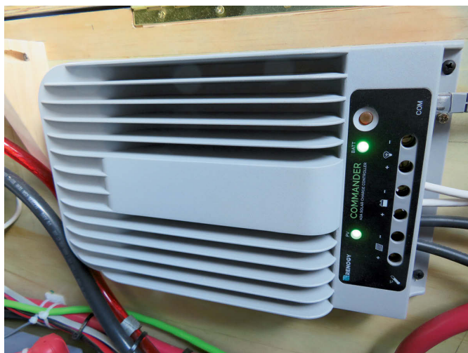
When David installed a solar battery charging system in the land yacht they now cruise in, he chose a Renogy MPPT controller, at left, to manage and monitor the charging process. The tracer meter, at right, allows him to set charge parameters and perform other functions.
