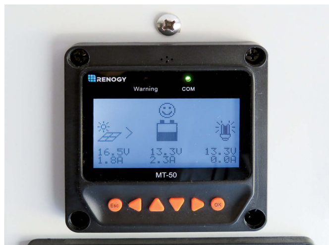
When David installed a solar battery charging system in the land yacht they now cruise in, he chose a Renogy MPPT controller, at left, to manage and monitor the charging process. The tracer meter, at right, allows him to set charge parameters and perform other functions.
