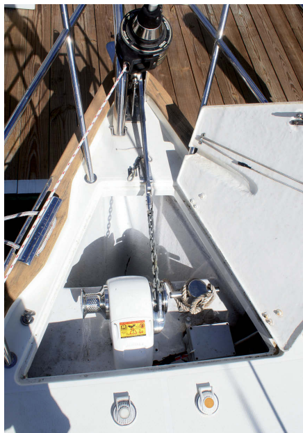
The foredeck on the Southerly 115 is furnished with heavy stainless steel cleats atop the bulwarks port and starboard, and a windlass and substantial Samson post inside the anchor locker.
