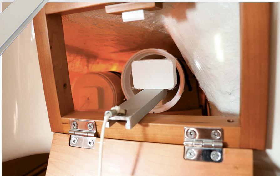
Joe's car is a length of aluminum extrusion with a block fastened to one end and a retrieval cord on the other. It slides along a track made of StarBoard.
