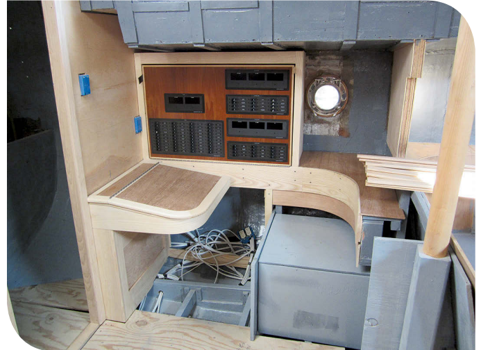
With a temporary cabin sole in place, at left, work began on the furniture. Dan contributed clever touches with his joinerwork, at right.
