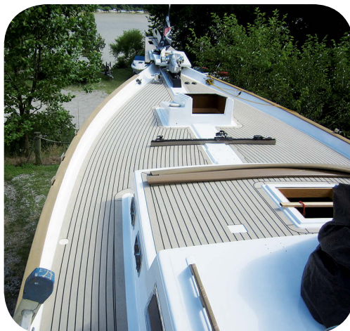
Cutting day for the bow-thruster housing brought on a case of nerves for Jim, at left. A ketch rig uses a lot of chainplates, at right. Pre-measured and precut synthetic teak decking was the solution to what could have been a major undertaking, below.
