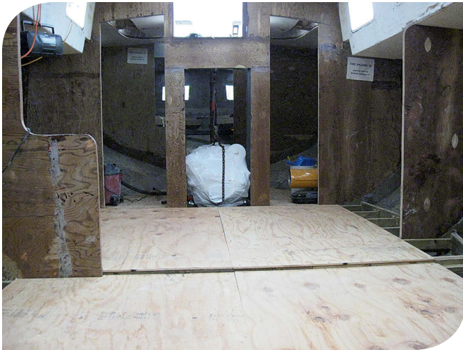
With a temporary cabin sole in place, at left, work began on the furniture. Dan contributed clever touches with his joinerwork, at right.
