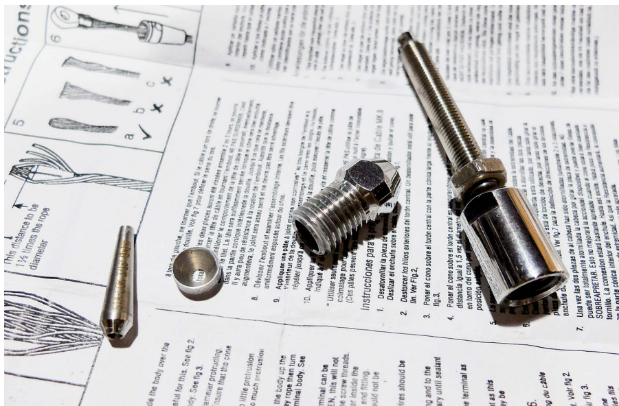
A Sta-Lok swageless compression fitting has four parts, the cone, the cap, the base, and the body, and it pays to read the assembly instructions.
