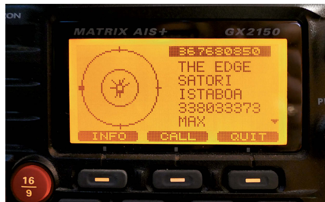
The red DSC distress button is under a hinged cover so it won't be pressed by accident, upper left. Selecting "Test" on the DSC menu tests the distress function, upper right. Selecting "Individual" from the menu allows the operator to call a vessel using its MMSI number, above left. This VHF set has AIS built in, so it can show nearby vessels with their positions, MMSIs, and other information, above right.
