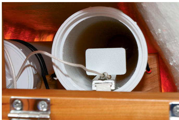
The tubes under the V-berth, at top, are hung fore-and-aft in 1-inch nylon webbing that is fed up through 3/4-inch holes cut into the bunk platform and fastened down with screws. The tubes in the cockpit coaming, above left, are bungeed onto cradle blocks set in place on the headliner with 3M 5200. Joe made a handsome access door to properly finish the job, above right.
