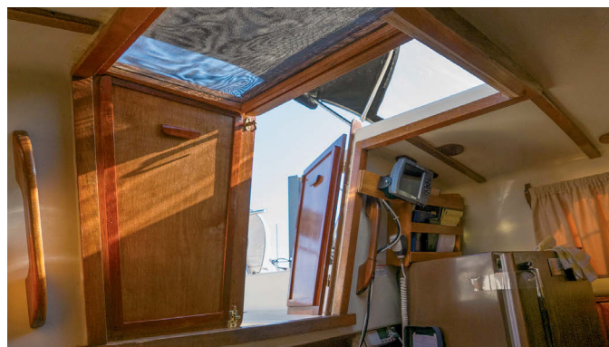
The complete assembly: Jim can still get ventilation without bugs while not exposing the boat's interior to the view of passersby in the marina, at left. The top screens are made so the port side can be opened to allow passage into and out of the cabin, at right.
