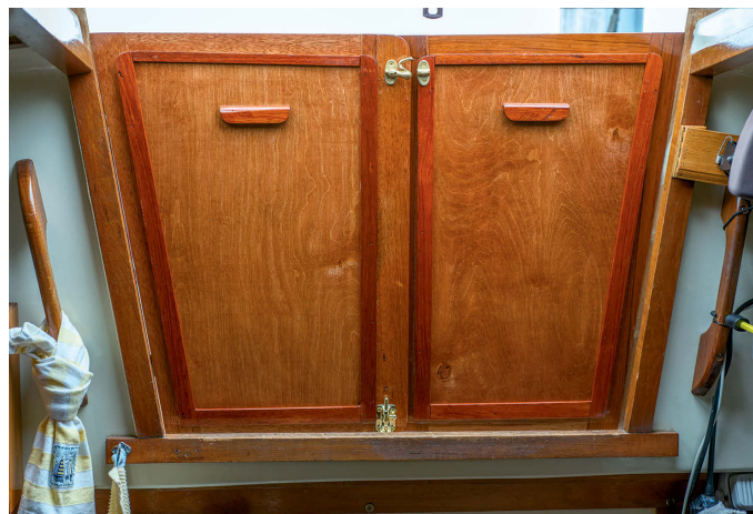
Jim made removable solid panels to fit into channels on the inside of each door, at left. He can slip them into place when he wants to close up the boat, at right, or remove them in fine weather when he wants some ventilation.
