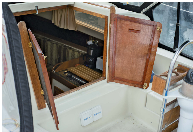
Jim made removable solid panels to fit into channels on the inside of each door, at left. He can slip them into place when he wants to close up the boat, at right, or remove them in fine weather when he wants some ventilation.
