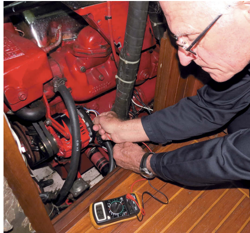
For his test equipment, David used, far left clockwise from top: a digital multimeter, laser tachometer, infrared thermometer, and a multimeter with a clamp. To simplify installing the Balmar AT-SF-200 alternator for testing, at left, he chose the model with mounts that matched those of Nine of Cups' alternator.
