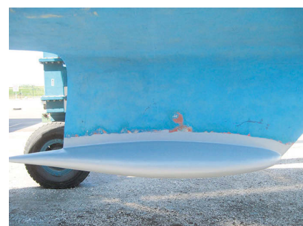
During the test fit, the keel began to take on its future appearance, at left. The bulb halves were then removed, for the keel surface to be ground to bare lead, then bolted back on with epoxy in the joint, center. The faired bulb and adjacent keel surface await paint, at right.
