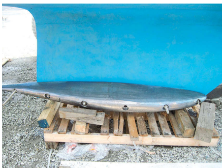
During the test fit, the keel began to take on its future appearance, at left. The bulb halves were then removed, for the keel surface to be ground to bare lead, then bolted back on with epoxy in the joint, center. The faired bulb and adjacent keel surface await paint, at right.
