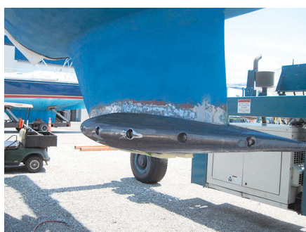
During the test fit, the keel began to take on its future appearance, at left. The bulb halves were then removed, for the keel surface to be ground to bare lead, then bolted back on with epoxy in the joint, center. The faired bulb and adjacent keel surface await paint, at right.
