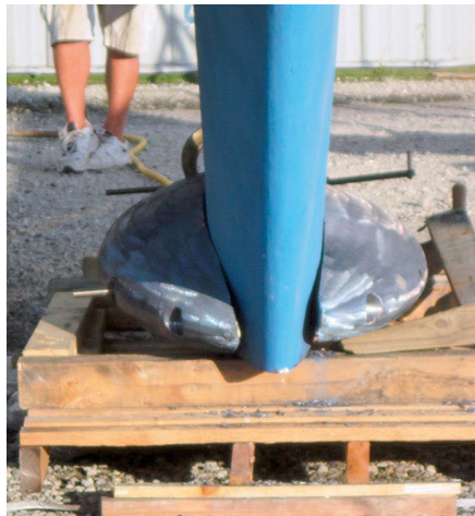
Lead is soft enough to cut with a saw, far left. After making the cut, the boatyard staff test-fit the bulb halves and drilled the holes for bolting them to the keel, at left.
