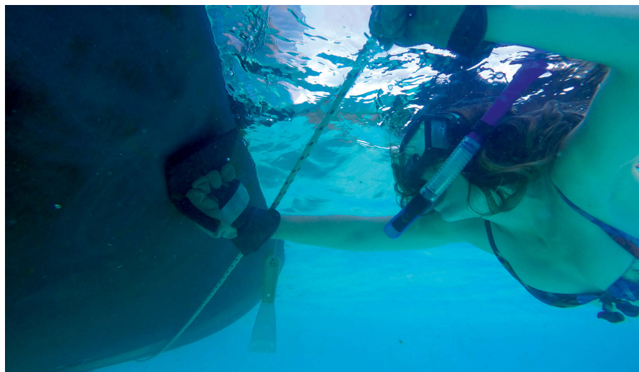
A line run from the bow, above, close to the intersection of the hull and keel, and to the opposite stern quarter, is a very helpful handhold.
