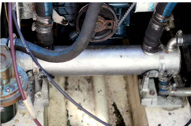
Either side of the heat exchanger, above left, can become blocked. The coolant side was clean and an acid bath removed calcification in the raw-water side. The thermostat, upper right, opened and closed on cue, and Robin replaced the coolant pump, above right.
