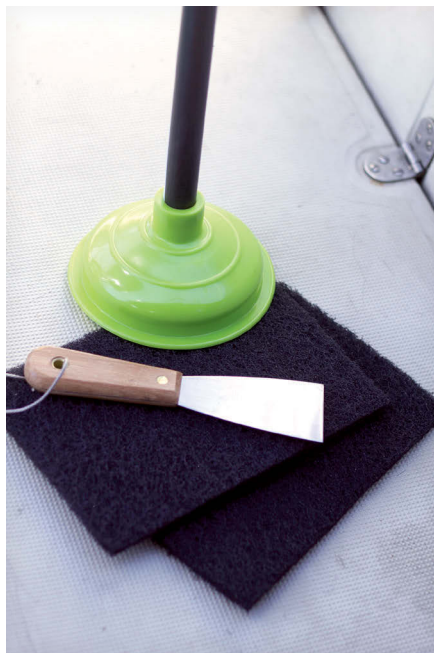
Key tools are toilet plunger, a putty knife for unprotected metal, and scrub pads.
