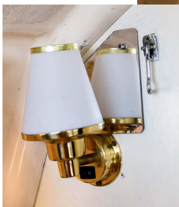
A mirror behind a cabin light is attractive in daylight, at left, and softens the light when it's lit, above.
