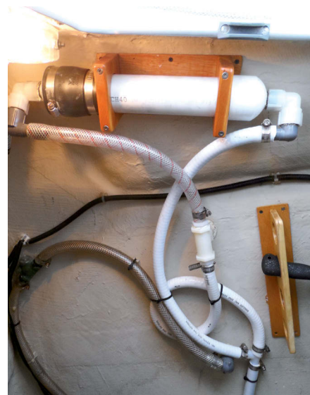
A filter (white cylinder) will freshen vented air but needs a bypass for protection.
