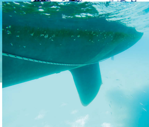
A line run from the bow, above, close to the intersection of the hull and keel, and to the opposite stern quarter, is a very helpful handhold.
