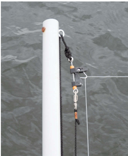
Drew's outriggers are electrical conduit with outrigger clips at the tips, upper left, and held in PVC pipe lashed to the pulpits, lower left. A fine striper caught on a yo-yo, below.
