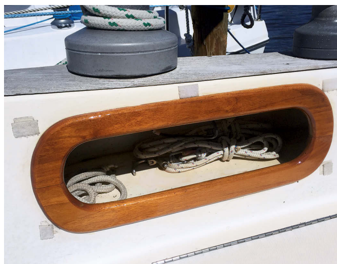
John says the grabrail on the cabintop is about 3 years old, at left, and has been recoated once, but the eyebrow on the cabin side is due another coat. The trim around the cockpit cubby, at right, is the same age as the grabrail. The Velcro tabs secure its protective cover.
