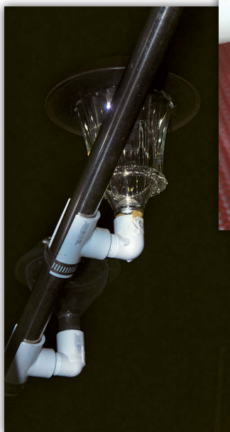
After cutting the stem of the light to a stub, he applied hot-melt glue and stuck it into the PVC elbow, above. The saddle tees clip onto any 1-inch rail, at left. If the boat's motion might cause them to rotate, he secures them with hose clamps.
