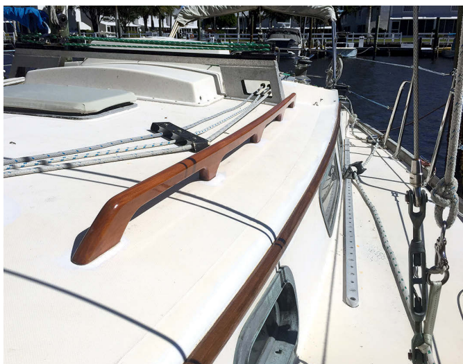
John says the grabrail on the cabintop is about 3 years old, at left, and has been recoated once, but the eyebrow on the cabin side is due another coat. The trim around the cockpit cubby, at right, is the same age as the grabrail. The Velcro tabs secure its protective cover.
