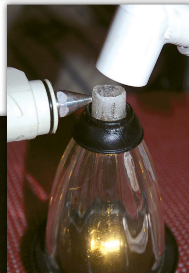
After cutting the stem of the light to a stub, he applied hot-melt glue and stuck it into the PVC elbow, above. The saddle tees clip onto any 1-inch rail, at left. If the boat's motion might cause them to rotate, he secures them with hose clamps.
