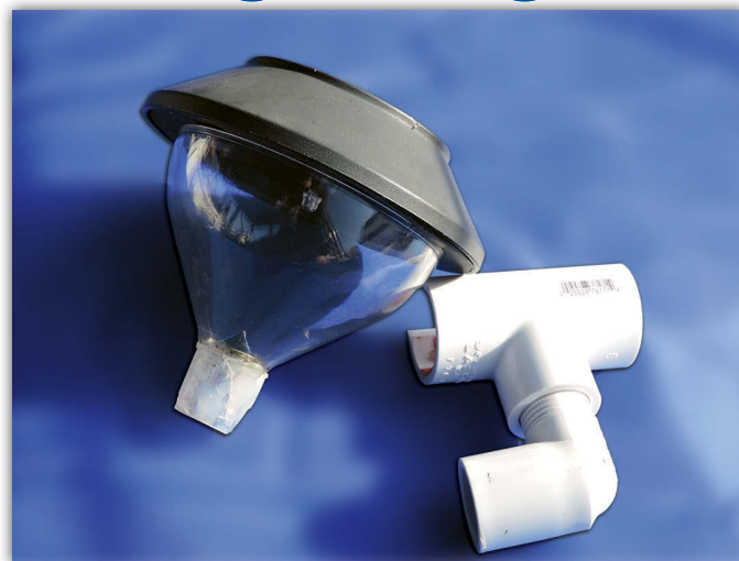
Gary made his $5 light from a high-intensity solar yard light, a PVC saddle tee, and a PVC elbow with a threaded end, above.
