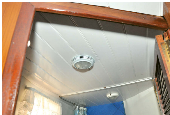
The heads are also much improved. When Roger removed the old vinyl liner, he also took down the overhead lights. Reinstalled, they help hold the boards in place.
