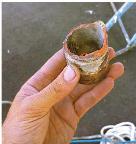
MonArk's bronze stern tube had corroded and become brittle, and it broke when Robin tried to fit a new stuffing box on it.
