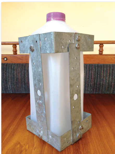
Milk is kept cold and accessible in this metal cage fashioned from galvanized tie straps and stainless-steel screws and nuts.
