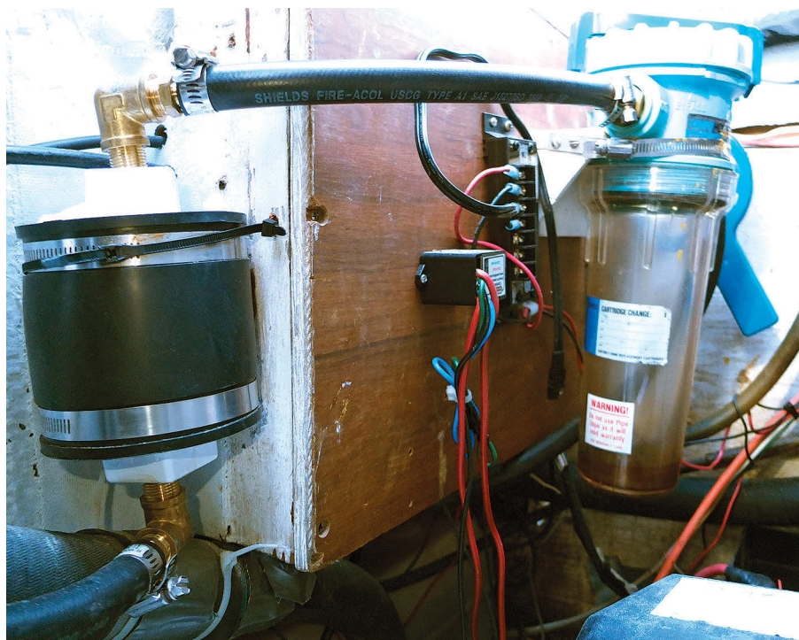
Cliff's burp catcher, at the right in the photo, has been doing its job of trapping diesel fuel. The dryer, at the left, is between the burp catcher and the vent in the transom.
