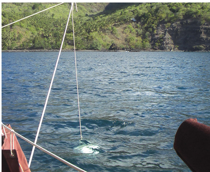
The pole needs a topping lift, a foreguy, and an after guy, at top. The flopper stopper is suspended from the trim line, which leads via a snatch block to the deck where it is adjusted and made fast.
