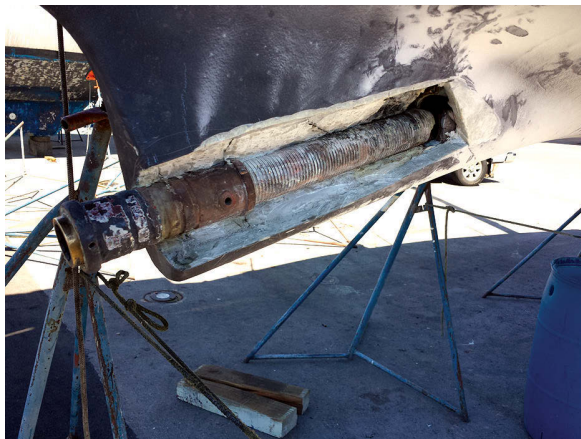
To extract the stern tube, Robin first ground off the bottom paint and gelcoat, above left. He cut a grid pattern to make chiseling away the fiberglass a little easier, above right. The tube, once exposed, below, was not difficult to remove, at bottom.
