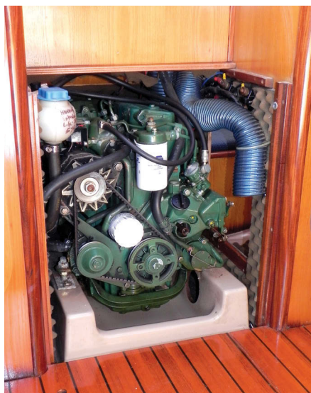
The engine is under the cockpit but access to it is good from the sides and when the companionway ladder is removed.
