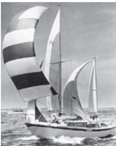
Charley Morgan's first boat, Brisote . Demonstrating considerable resourcefulness, she had a Star Boat keel and rudder, a Thistle mainsail, and a modified Penguin sail for a mizzen.
