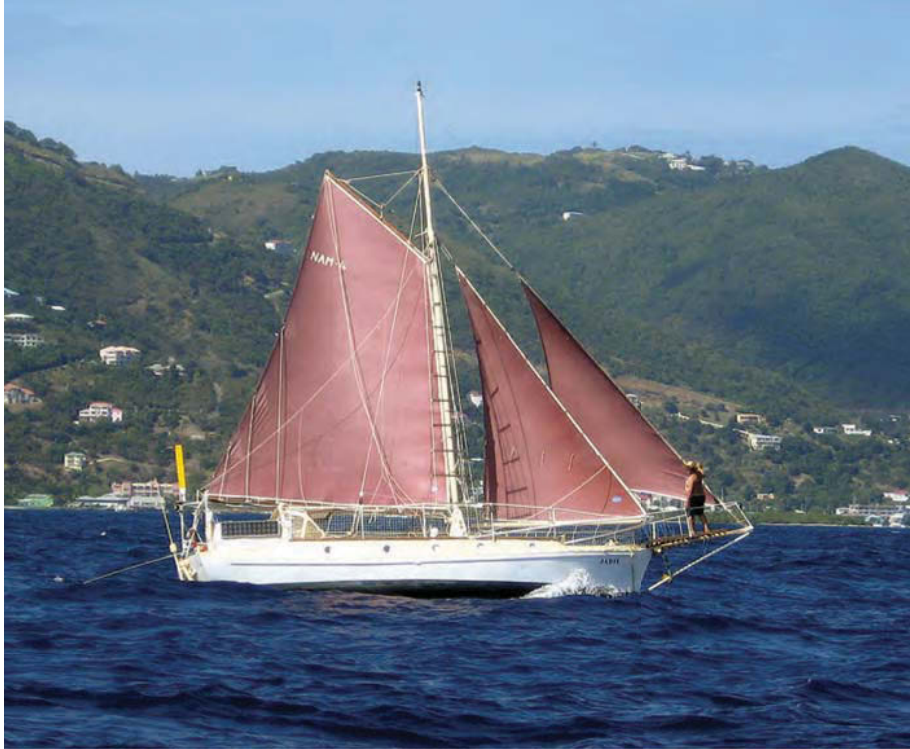
Jadie is a steel gaff-rigged cutter built by Martin and Leslie Klein in Namibia. She has sailed Caribbean waters since the late 1990s. She has no roller furling and sets a variety of small sails, all easily handled by even the smallest crewmembers.
