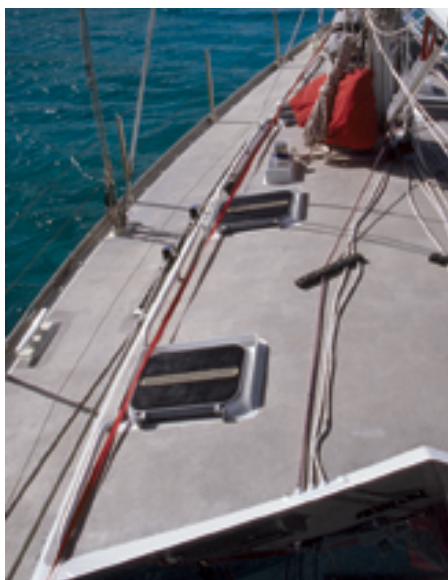
These jacklines, consisting of a ¼-inch Spectra line threaded through the red webbing, are strong but won't roll underfoot.
