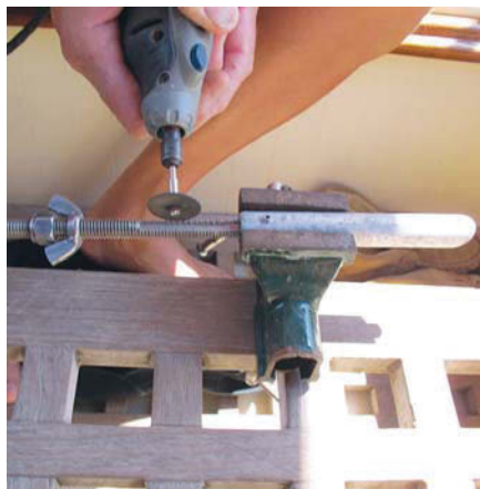
With the support strut released, the seat folds down for quick stowage, at left. Grinding the groove in the support rod takes patience, center, and safety glasses are essential. A Dremel tool and sanding drums can be used instead of a router to trim the edges of the hatchboard, at right.
