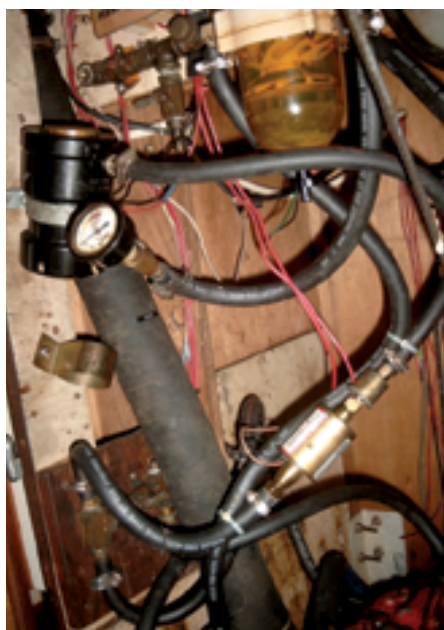
Clean fuel is essential to a diesel engine's reliability. A grit filter helps keep it clean and a vacuum gauge monitors the condition of the filter.
