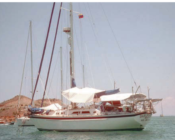
The light blue Bimini lining reduces heat, top photo. The top photo also shows aft bows attached to the stern pulpit, the outboard motor lock, and other safety gear. Next photo shows the Bimini with side wings. The rain hood, in third photo, also made a big difference by allowing for ventilation during rainstorms at anchor. Dahlfin stays as cool as is possible in Grenada with all the suncovers employed, bottom photo.
