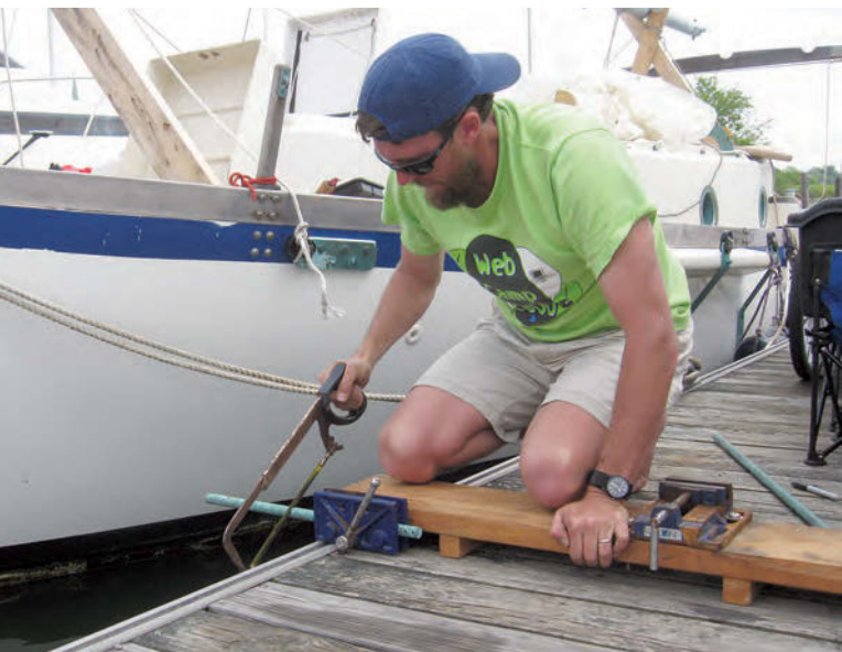
Ben fitted a woodworking vise and a drill-press vise to his portable workbench, at left. The two wooden feet underneath fit securely into Ganymede's foc's'le hatch coamings when Ben has a project he can work on when on board. Ben sharpens a long drill bit on his hand-powered grinder, at right. This one is made by the Prairie Tool company and costs about $15. It attaches to the table with a screw clamp. A big wooden clamp holds the boom jaws to the fiberglass boom, below, until they can be glassed firmly in place.
