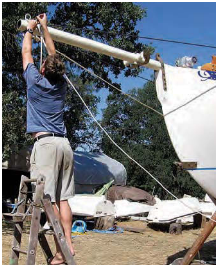
Ben fits whisker stays to Ganymede's fiberglass bowsprit shortly after he'd installed it, at left. Ganymede's 8-horsepower Yamaha outboard engine and its bracket were still looking good in Cartagena, Colombia, after 5,000 miles of exposure, abuse, and a passage through the Panama Canal, at right.
