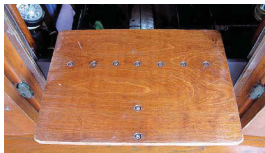
Ed hinged the seat off-center to leave room forward of it for standing on the ladder, top left. To ensure the seat was smooth, Ed countersunk all the nuts and cut the bolts flush with the nuts, left center. The support-rod assembly is made up of a threaded rod, compression tube, stopper nut, and a tensioning wingnut, bottom left. With the support rod in place and the limiting strap taut, the seat is ready for use, top right.
