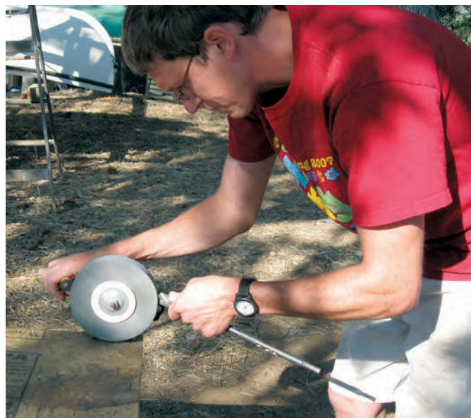
Ben fitted a woodworking vise and a drill-press vise to his portable workbench, at left. The two wooden feet underneath fit securely into Ganymede's foc's'le hatch coamings when Ben has a project he can work on when on board. Ben sharpens a long drill bit on his hand-powered grinder, at right. This one is made by the Prairie Tool company and costs about $15. It attaches to the table with a screw clamp. A big wooden clamp holds the boom jaws to the fiberglass boom, below, until they can be glassed firmly in place.
