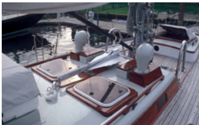
Anchors like the Fortress and Danforth stow well in chocks on the coachroof or pulpit.
