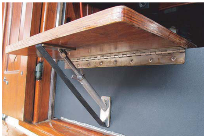
Ed hinged the seat off-center to leave room forward of it for standing on the ladder, top left. To ensure the seat was smooth, Ed countersunk all the nuts and cut the bolts flush with the nuts, left center. The support-rod assembly is made up of a threaded rod, compression tube, stopper nut, and a tensioning wingnut, bottom left. With the support rod in place and the limiting strap taut, the seat is ready for use, top right.
