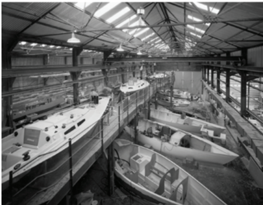
In 1979, Camper & Nicholson's "B" shed had several models of production fiberglass sailboats under construction. From the foreground looking back is a Nicholson 33 hull, two 35s, a 32, and a 31. To the left is a deck for the 33 and behind it two decks for 35s.
