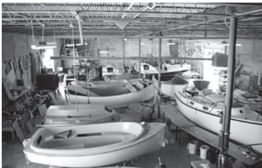
A worker at the Hutchins yard puts finishing touches on an Eclipse, at left. The company subcontracts the construction of the hulls, liners, and decks. The final assembly and all finishing work, such as deck fittings and cabinetwork, is done at the Hutchins facility in Clearwater, Florida, shown above.
