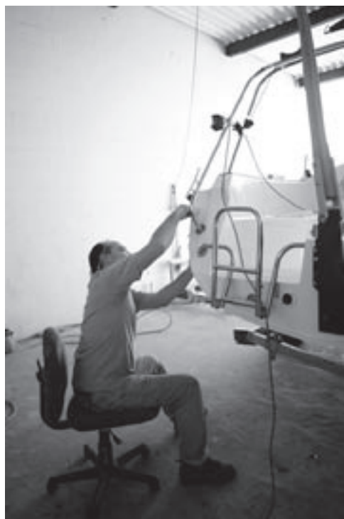
A worker at the Hutchins yard puts finishing touches on an Eclipse, at left. The company subcontracts the construction of the hulls, liners, and decks. The final assembly and all finishing work, such as deck fittings and cabinetwork, is done at the Hutchins facility in Clearwater, Florida, shown above.
