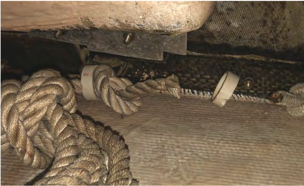
Above and below, the rings are attached to overhead bolts at the deck edge and used to hang fender lines and docklines.
