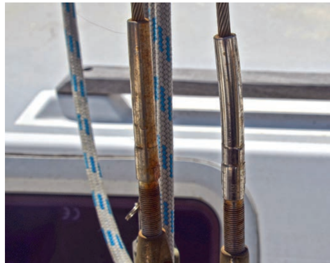
Banana swage, causing misaligned wire with uneven loading across the 19 strands.
