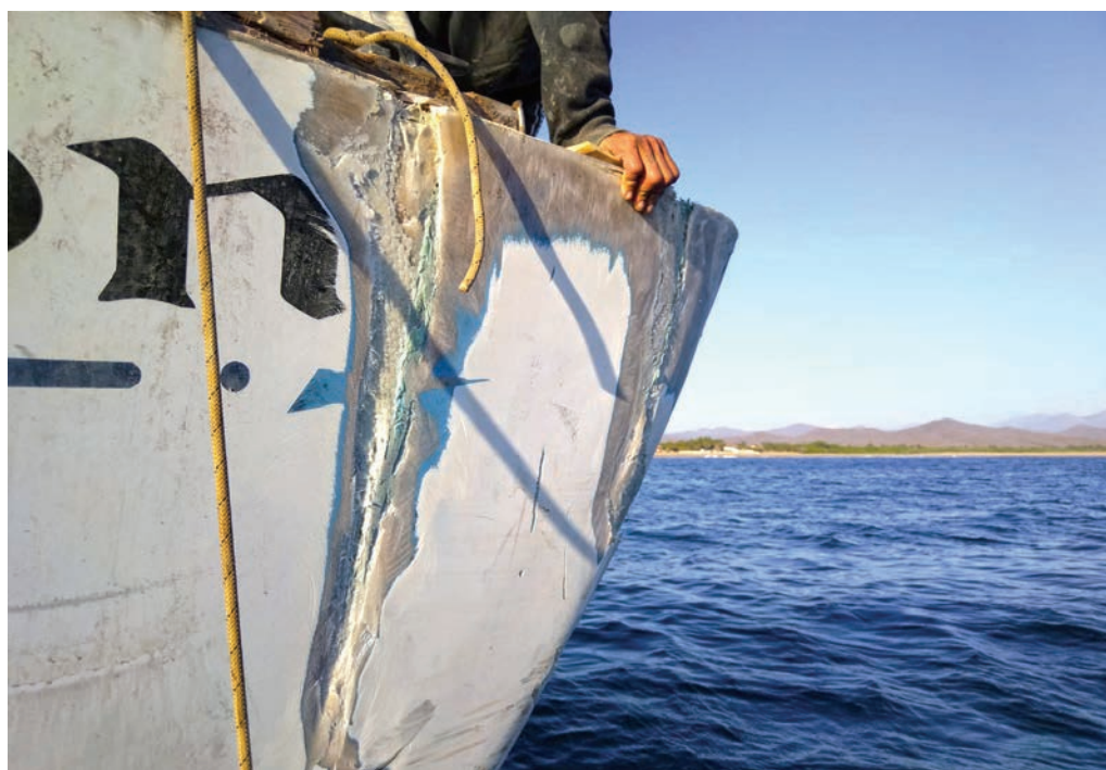
Repairs begin on Falcon's damaged bow while on a stern anchor.
