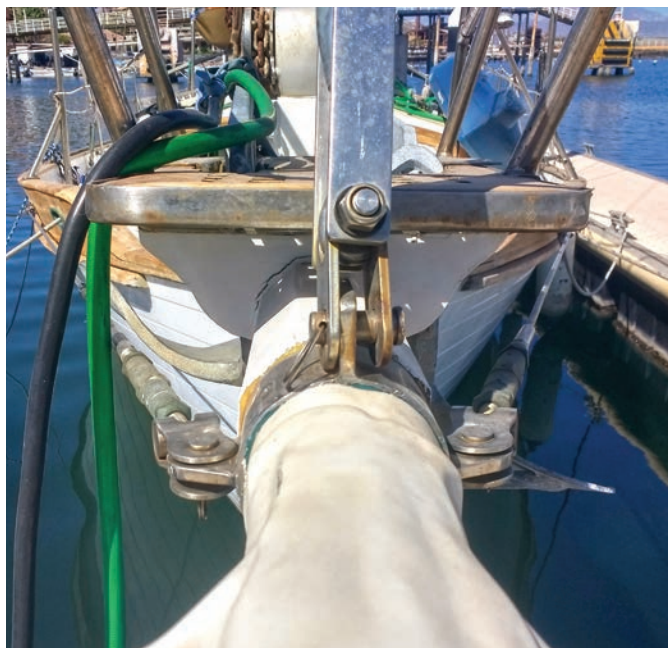
Headstay toggle shifted to one side, with dark rust from failing stainless steel.
