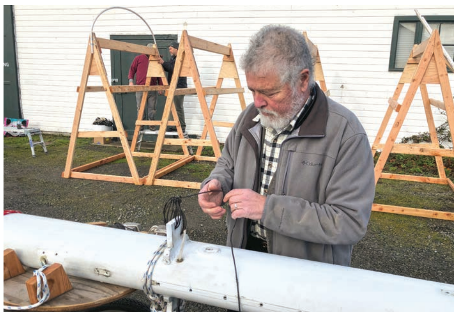
Rigger Brion Toss ties one of the loops that will be used to suspend the mast over the next several months.
