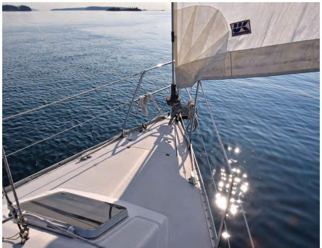
The bow is clean, with ground tackle stowed in a locker and cleats mounted quite far aft and near the rails.
