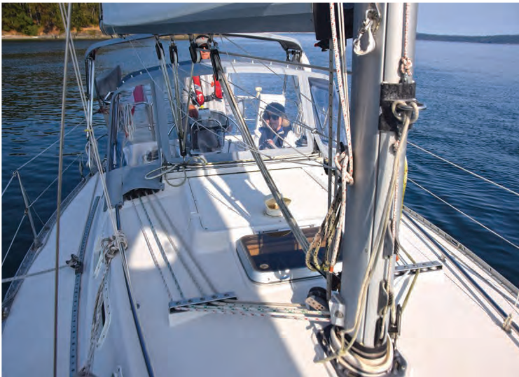
Halyards are led aft from the mast base through turning blocks.
