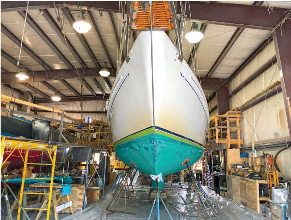
Andiamo with her old peeling ablative bottom ready to be soda-blasted.
