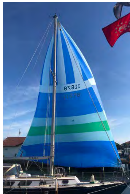
Above, the recut spinnaker now has a better shape for reaching, and is lighter and easier to handle.
