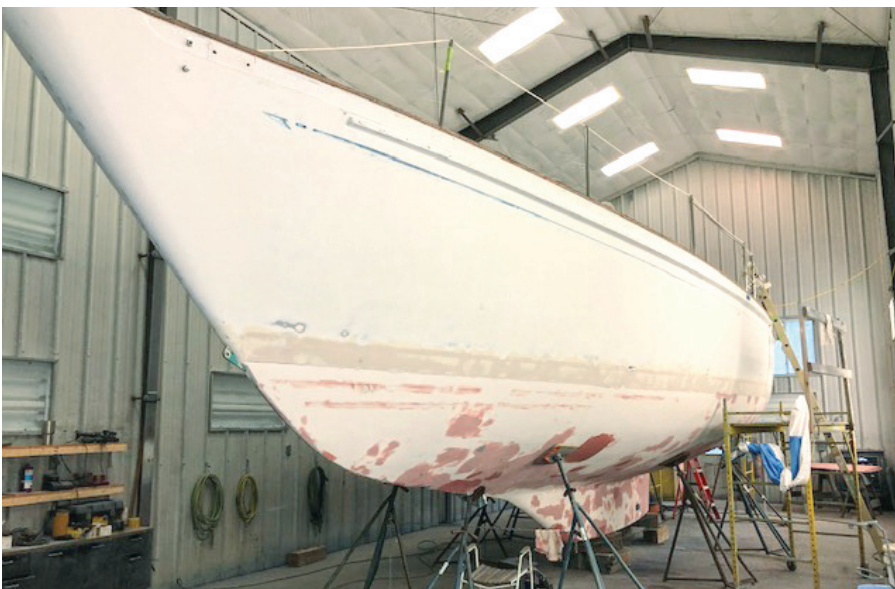
The bottom after being soda-blasted to remove 30 years of old bottom paint.
