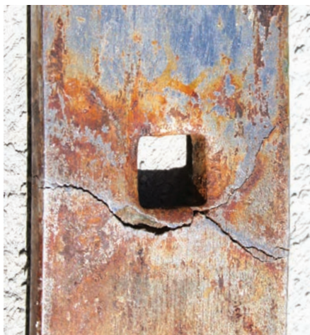
A closeup of the cracked chainplate shows some normal corrosion and abrasion. But what's lurking beneath the surface?
