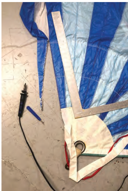
On left, in the radial head area of the sail, John used a hot knife to remove multiple layers of reinforcing, with the seam acting as a guide.
