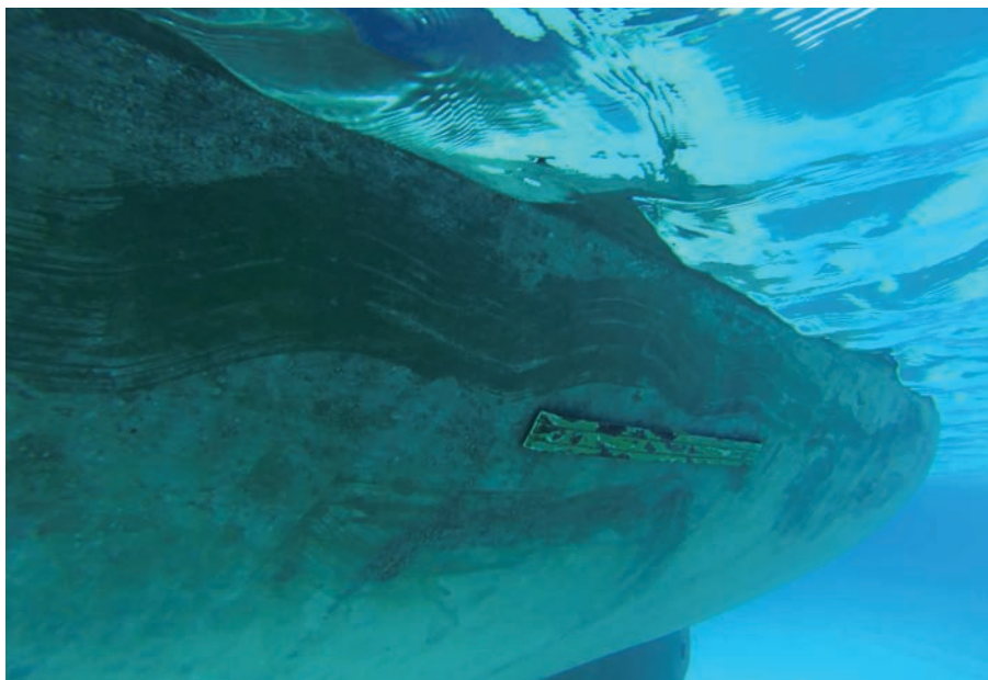
Andiamo's bottom after about six months with Coppercoat. A light layer of slime is visible.
