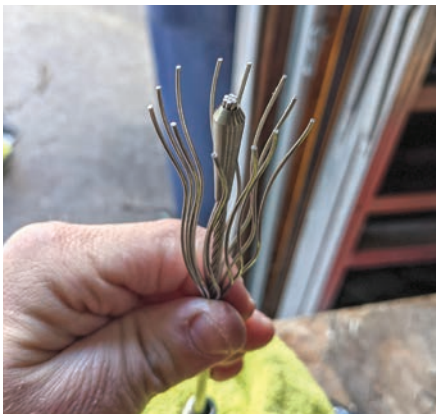
Top left, unwrapping the outer wires and inserting the Sta-Lok wedge.
