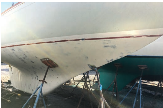
On left, Constance's hull looking smooth after wet-sanding.
