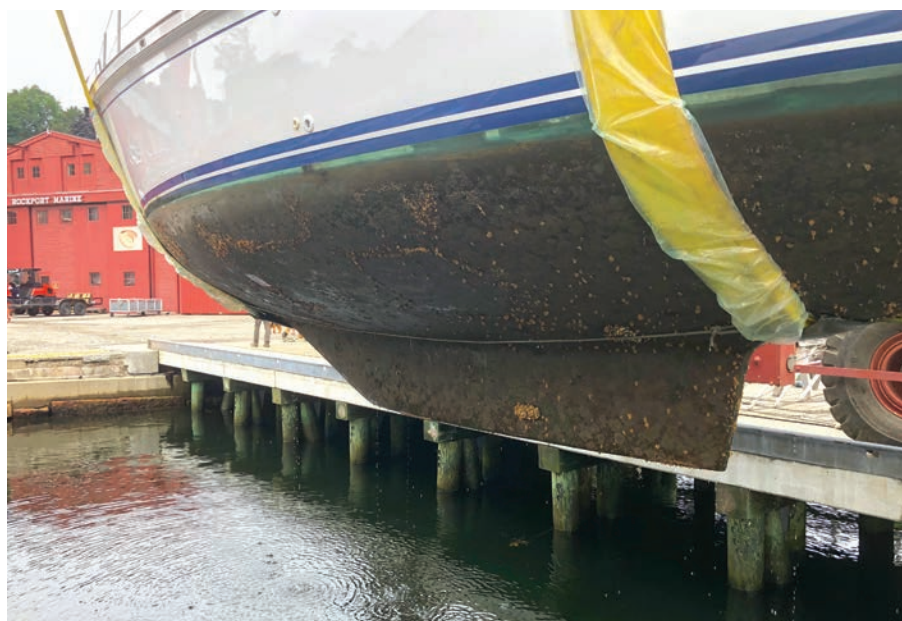
The boat bottom after a year of cruising with Coppercoat. The slime and a small number of barnacles were easily removed with a powerwash.
