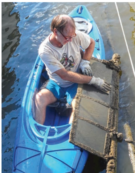
Drew Frye cleans a four-panel paint testing board.
