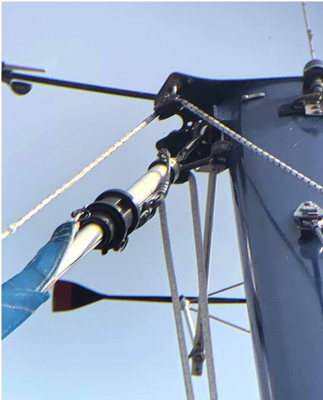
Above, the top of Juniper's mast showing the halyard wrap.
