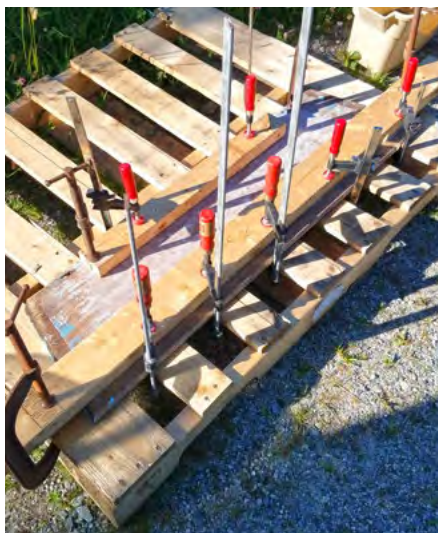
Chi's aft thwart was badly curled. After soaking in wet cloths and bags, it was clamped until it flattened out.
