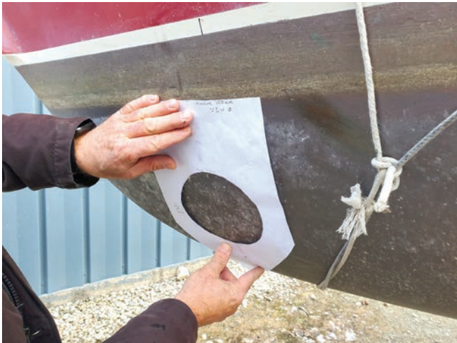
Bill and David used a template to determine the height of the bow thruster, based on the waterline and bottom of the hull.
