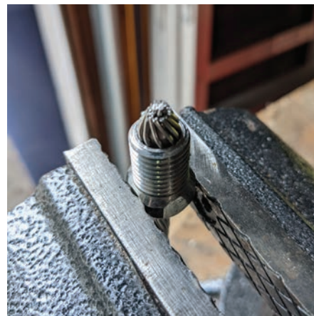
Below, opening a terminal to double-check that everything came together correctly before rerigging the boat.
