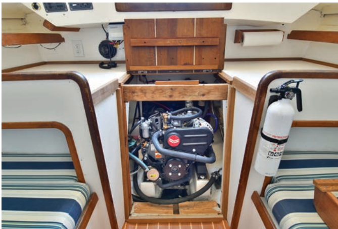
Engine access is from the front and above and makes servicing reasonably easy.
