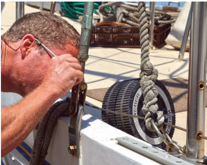
Inspecting a shroud with 10X loupe to sleuth out possible metal faults.
