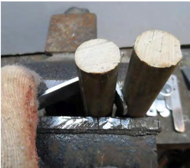
On left, step-by-step fabrication of the hooks, which are bent slowly, using cut broom handle pieces held by a vice.
