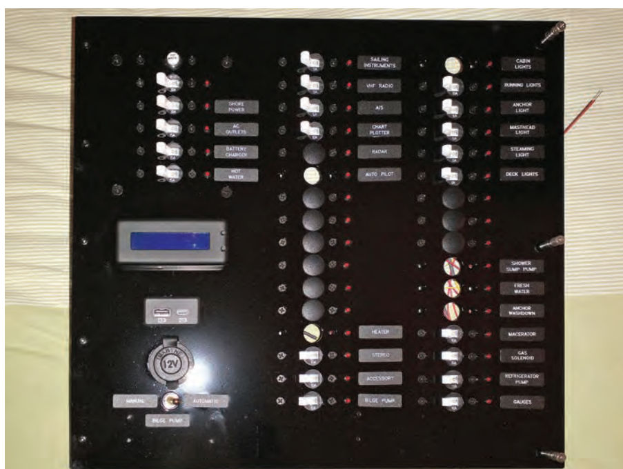
Front view of the wired panel, ready for installation.
