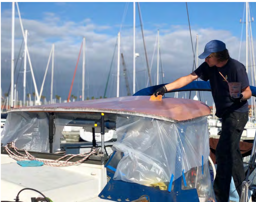
Applying fairing compound to the new hardtop, top left. Note the supports beneath, which Chris added when the new core material developed some dips as glass and fairing were added.
