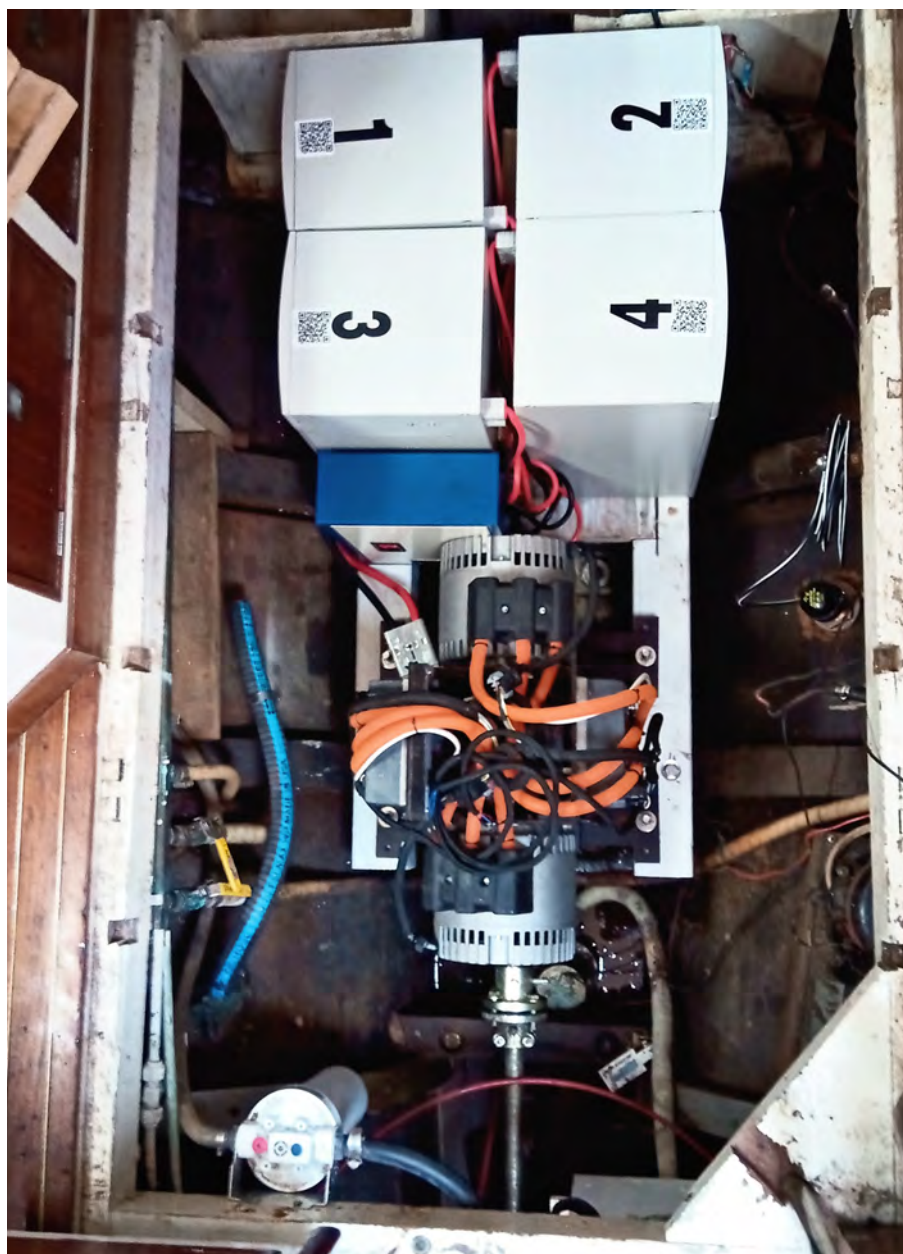
The new system, including batteries, fits neatly into the space that once held the Perkins 4-108.
