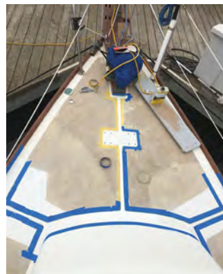
(Above and below) The foredeck in mid-repair, and after completion, coated with new KiwiGrip non-skid.
