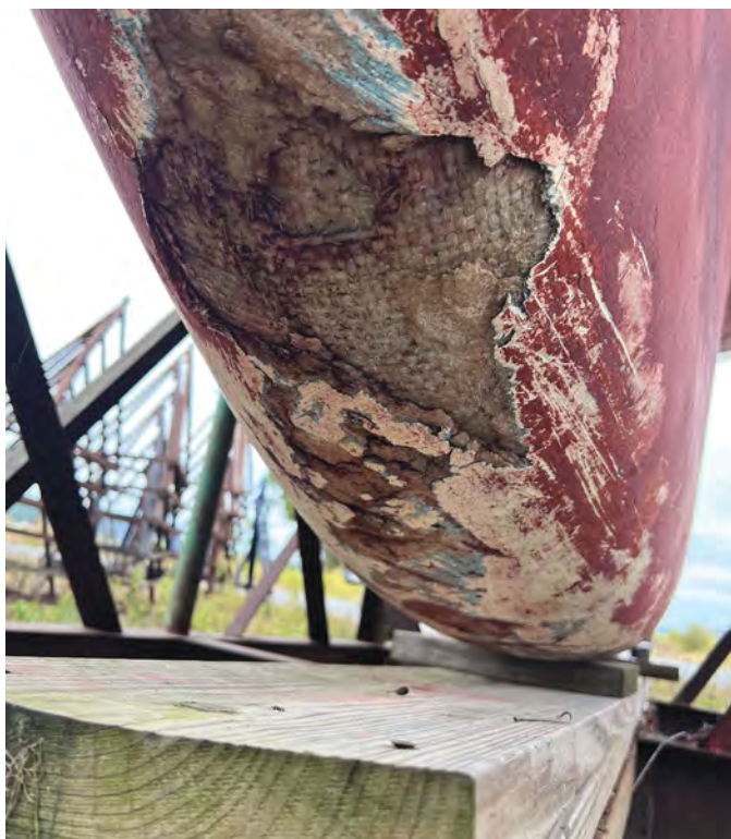
After the cruise was over, Tom finally saw the nasty results of two close encounters with the submerged rock known as Hen and Chickens off the mouth of the Connecticut River.
