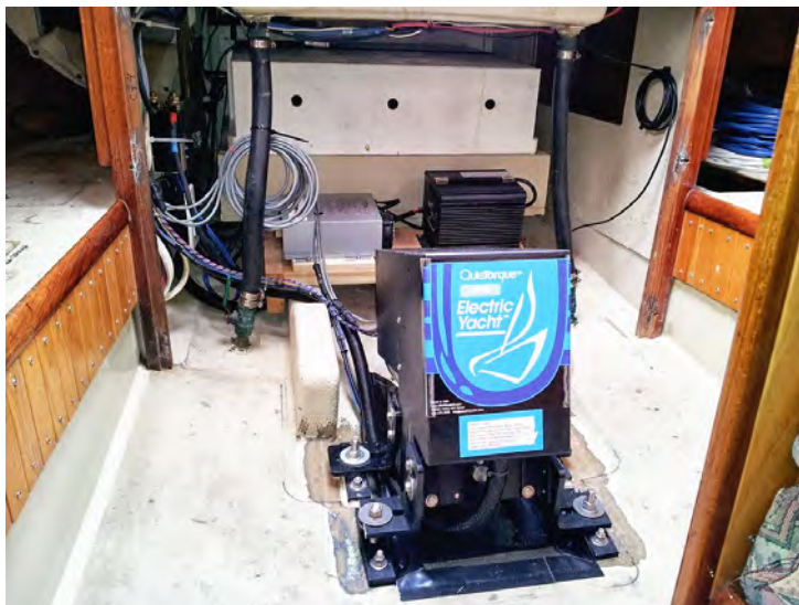
A clean install of an Electric Yacht QuietTorque 180iBL on the 1975 Cal 2-34 Footloose. Photo by Kirk Grier.
