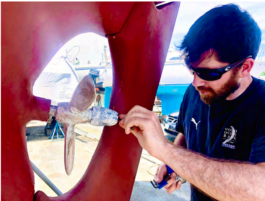
Adam performs some annual maintenance on the propeller, replacing the zinc and applying a new coating of PropSpeed.
