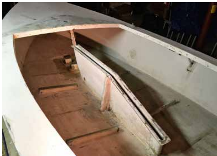
The deck undergoing filling and fairing. Fiberglass work included filling in all old holes, at top.
