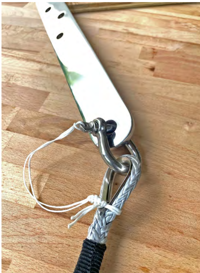
A mock-up of a JSD bridle leg attached to the chainplate, which would be installed on the aftmost hull, just below the toerail and extending slightly off the transom.
