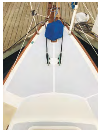
(Above and below) The foredeck in mid-repair, and after completion, coated with new KiwiGrip non-skid.
