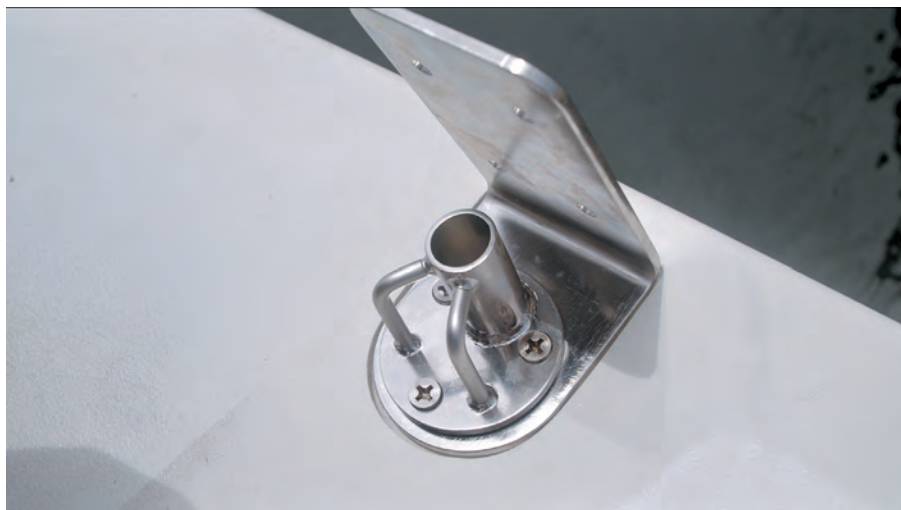
An L-bracket and stanchion base fully installed for the new bulwark configuration.
