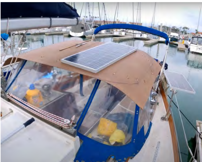
Chris and Marissa used the old dodger as the template to shape the new one. Here, the new material is laid on top of the old dodger and a solar panel placed in approximate position for sizing.
