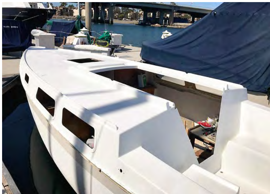
One More Time midway through the restoration, with the deck and cockpit repaired and repainted, still awaiting deck hardware, new portlights, and a new companionway slider, at right.
