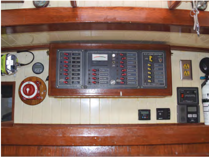
The well-equipped electrical panel is located behind the companionway steps, clearly visible and accessible with no chance of accidental contact, above.
