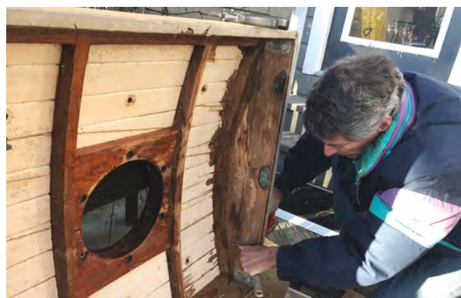
Jeremy starts to dismantle the original hatch.
