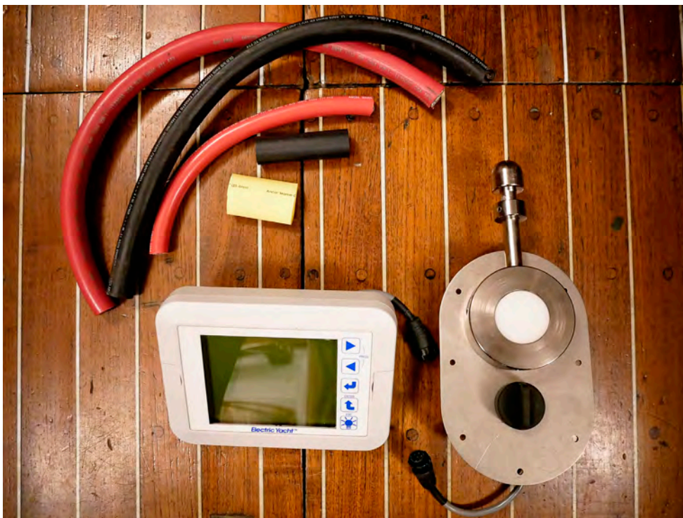
Some of the components of the motor, before installation, include the display, throttle lever with key switch, and two sizes of wire used for the custom lengths that Larry had to make for his installation.
