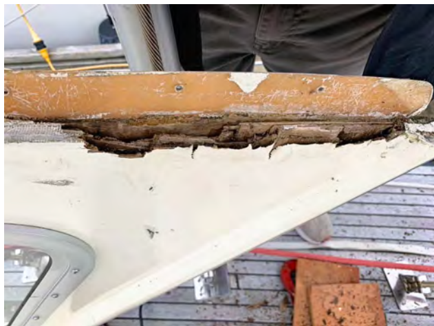
The exposed rotten wood on the dodger's base (top) and the repaired area after "Git"-Rot application and fairing (below).
