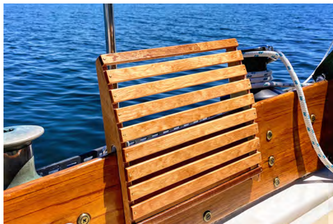
One of the coaming board extensions installed and ready for use, above.
