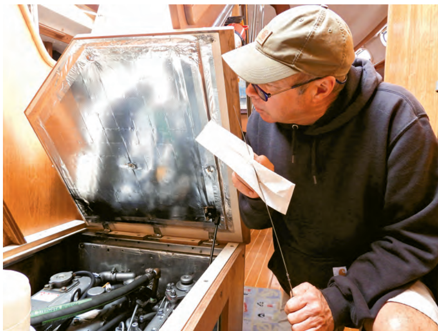
Giving the engine oil a sniff is a good way to detect for internal engine issues, such as a bad fuel injector or worn rings, above.
