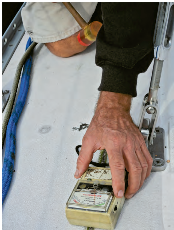
Using a moisture meter, Tarn checks the deck around the chainplates of a Catalina 46.
