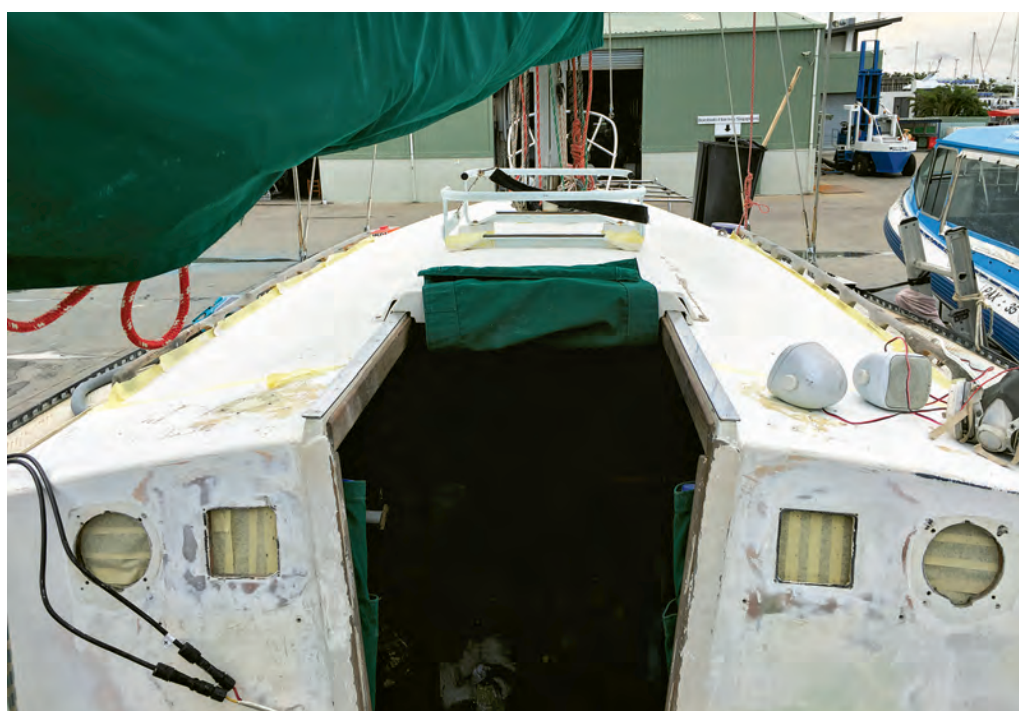
In mid-refit, the deck is stripped and prepped for new line organizers and rearranged deck hardware to improve shorthanded sailhandling, below.
