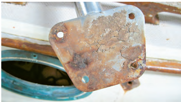
Bedding compound gone bad after years under a stanchion base, at top left.
