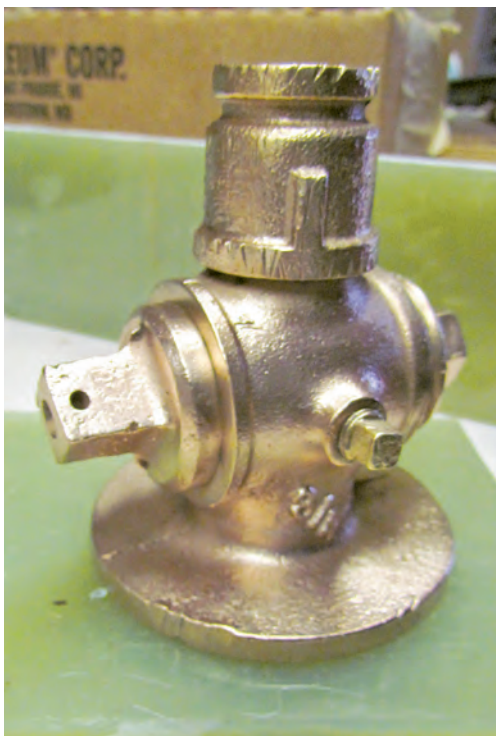
The metal refit began with one of the boat's seacocks, shown here before and after refurbishment.
