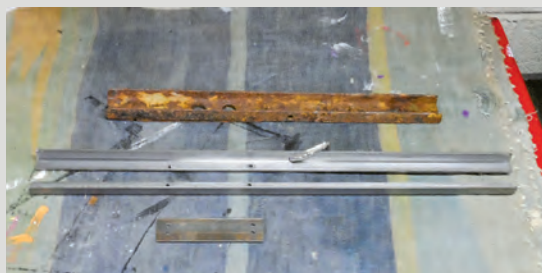
Drew's old cross stock, and the parts for the new cross stock, ready for paint and assembly.
