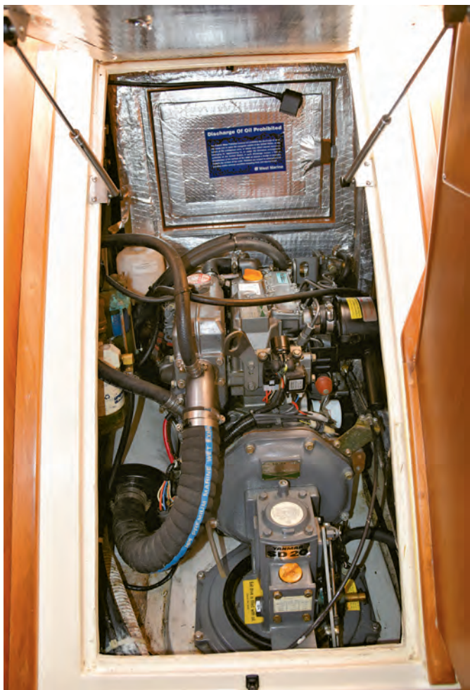
Lifting the gas-assisted companionway steps, one finds the aft end of the engine and top of the saildrive. Access to the front of the Yanmar is through another access door in the aft cabin.
