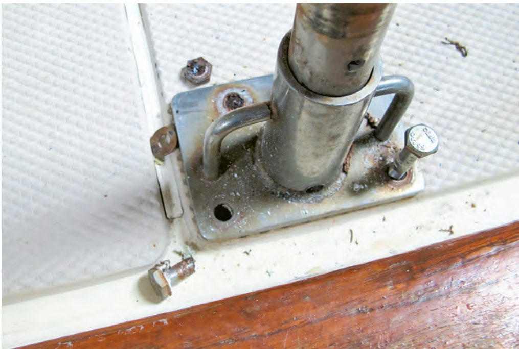
Stanchion bases were especially susceptible to corrosion.
