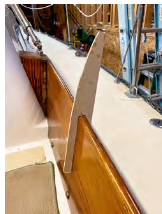
One of the coaming board extensions installed and ready for use, above.
