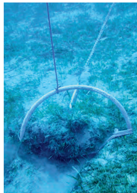
This anchor is showing how the sod-cutter effect can result in a bad set when weeds hold the shank and rode above the root mat, preventing the anchor from digging deeper.
