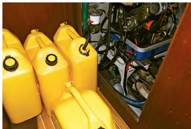
David pulled fuel from the tank through the water separator/filter and into clean jerry cans where it stayed until the tank was clean.
