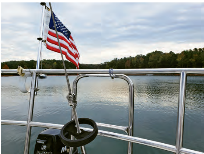
Before the modification, the solid stern pulpit meant climbing over the 30-inch-tall top rail to use the stern ladder.
