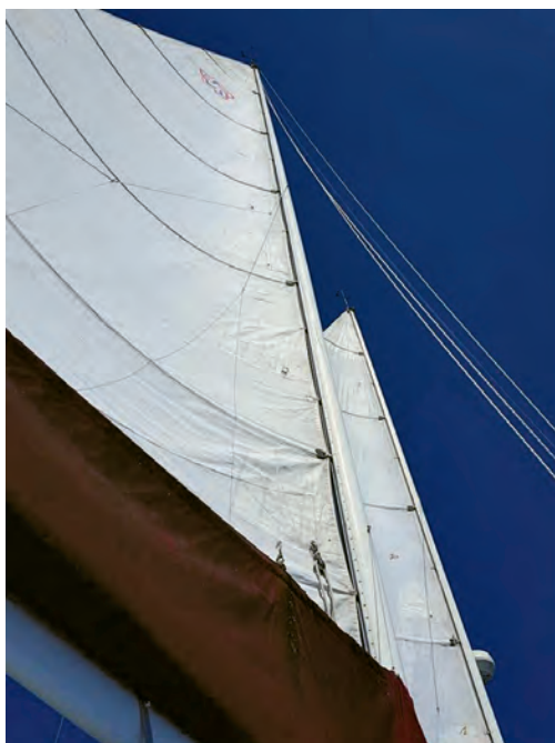
Goodwind, a 1984 Freedom 39 Pilothouse Schooner, features the original Freedom Cat Ketch rig as it evolved with full length battens and conventional booms and vangs. Photo courtesy Greg Cantori.
