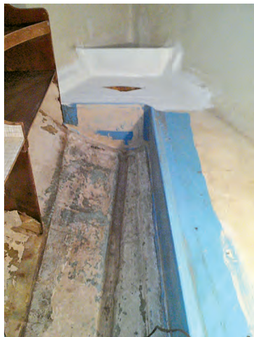
After scrubbing and bleaching the boat's entire interior and priming it with Dulux Exterior Latex Primer, Lee applied two coats of Interlux BilgeKote to create a sparkling white space down below.
