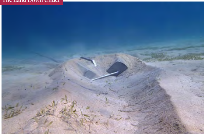
This Delta anchor is clearly making no progress in setting. It should be retrieved and checked for debris. Finding none, the captain should consider a different anchor in the same location, or a different location with this anchor.
