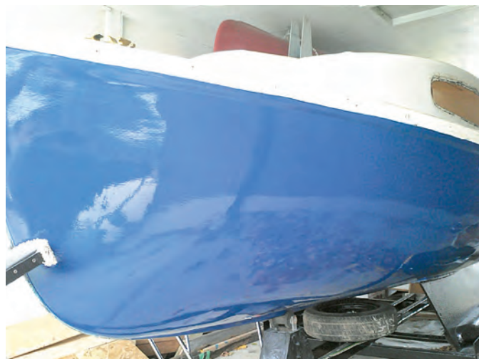
The thick fiberglass hull was in good shape, despite years of neglect, and required just a little sanding and fairing to prep her for a new paint job, which Lee accomplished using the roll-and-tip method.
