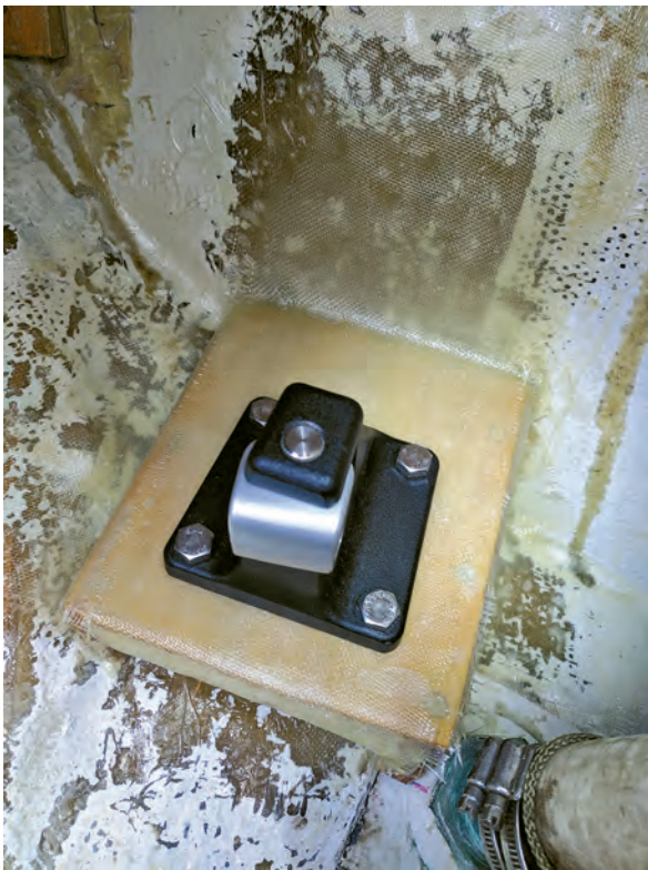
The new shelf glassed in with the mechanical linear drive mounting foot installed.
