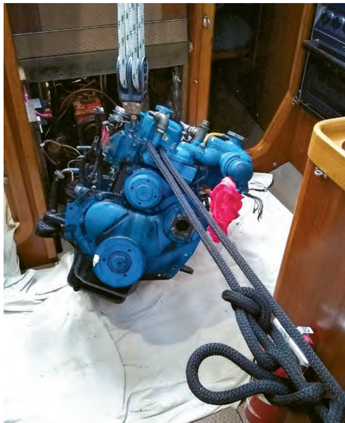
The oily mess of the old engine is pulled up and forward as it's extracted from the engine compartment.
