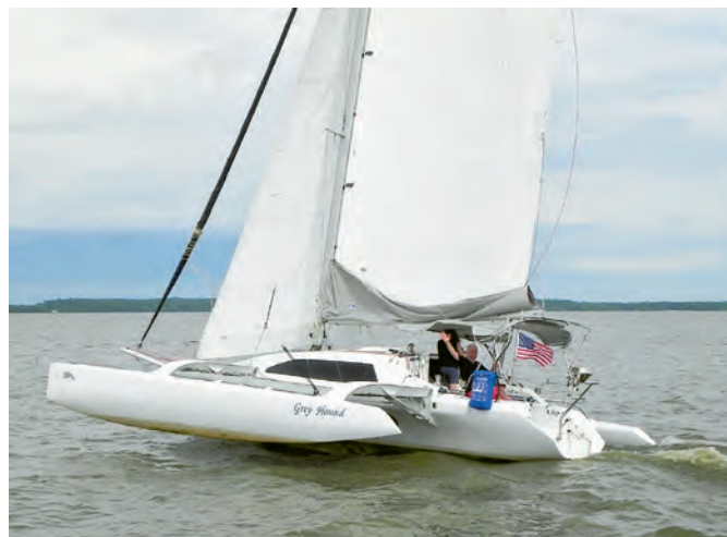
Flying a hull, Grey Hound remains steady and easy to handle. Even at speeds of 18 to 20 knots, the F-33 feels stable, as apparent wind moves well forward, and the boat changes speed with changes in wind velocity.
