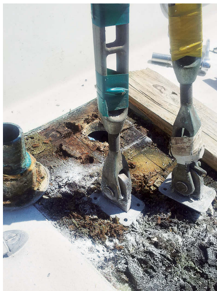
Other areas where the core was rotten were the coachroof, at left, and around the chainplates, center, the latter caused by a poorly sealed fuel fill. Sighting along the stern tube solved the shaft-alignment puzzle — the tube had a bend in it, at right.
