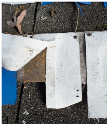
Polyurethane adhesives remained well-adhered to the bottom surface, but peeled cleanly off the UV-exposed side.
