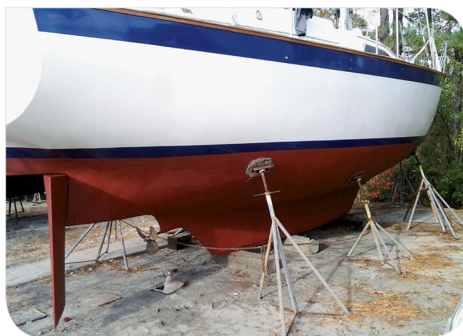
Removing years of marine growth left the bottom looking rough, at left, so the bottom, and the topsides, received fresh coats of paint.
