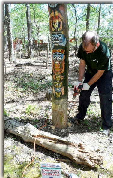
Drew tested his borax preservative on a totem pole. The pole lying in the foreground is from the same tree, and the same age, but has not been treated.
