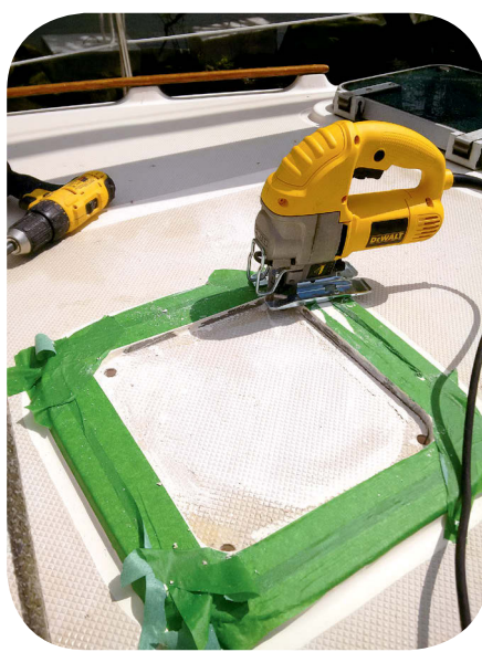
Once he was sure he had all the details right, Matt epoxied the hatch base in place, at left. He applied and faired the gelcoat before cutting the hole, then masked it for protection before making the cut, center. After cleanup, the base was ready to receive the new hatch, at right.
