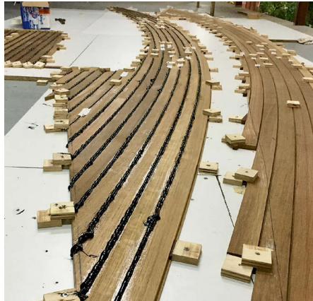
A worker used his hands and feet to fit the teak strips together, at left. The assembled deck panels are glued together with caulk, below.
