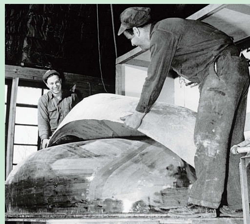
Workers in Ray Greene's shop pull a cured dinghy hull off a male mold, above, circa 1947-49. The exterior had to be sanded and painted.
