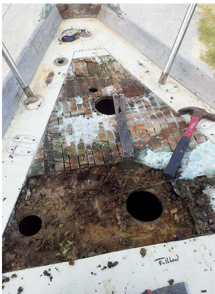
Before recoring the foredeck, Jon took measurements of the hardware locations, far left. He cut out a section of the top skin and chipped away the old core, at left, cleaned up the area, then laid the new core and the first layer of fiberglass, above.
