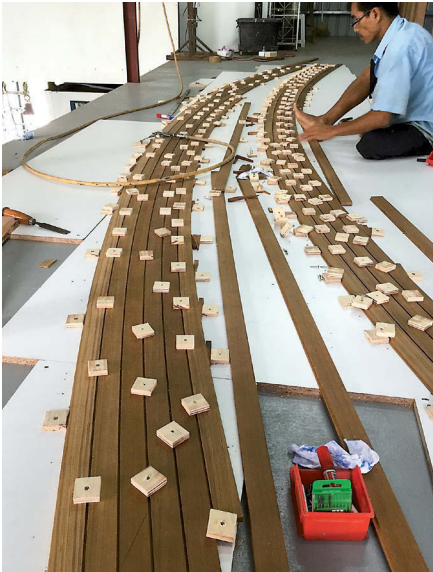
A worker used his hands and feet to fit the teak strips together, at left. The assembled deck panels are glued together with caulk, below.
