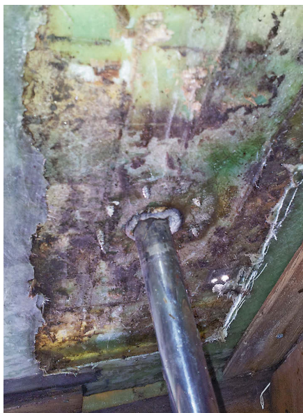
Other areas where the core was rotten were the coachroof, at left, and around the chainplates, center, the latter caused by a poorly sealed fuel fill. Sighting along the stern tube solved the shaft-alignment puzzle — the tube had a bend in it, at right.
