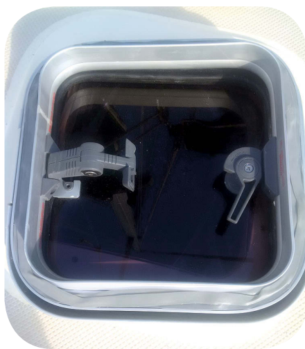
Matt applied butyl tape as the sealant between the hatch flange and the base.
