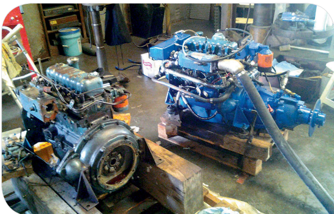
The new Perkins engine was a short block, and Clay completed it with parts scavenged from the old engine.
