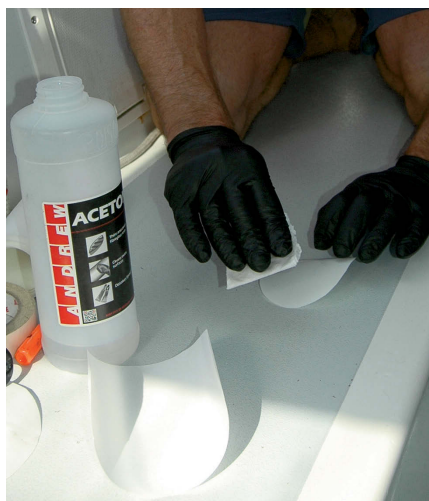
Chafe damage, at top of page, is a good candidate for a 5200 repair. Cut a patch to overlap the damaged area and wipe it and the sail with acetone, at left. Apply the 5200, at right.
