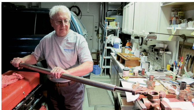
Never again! During the latest refit of Entr'acte , Ed replaced the one ball-valve seacock with the original tapered-cone seacock.
