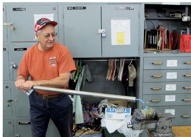
Ed tried ever-longer levers in his attempts to open the ball-valve seacock, but to no avail. He had to disassemble it.
