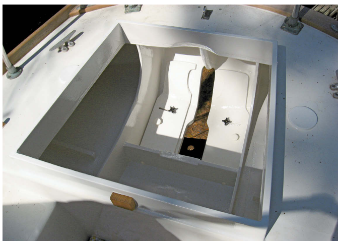
On another Alberg 30, James cut a narrower slot in the hull and transom, at left, for the smaller 6-horsepower motor, at right. The hatch was slightly smaller, so its lid did not require a raised center, and the original traveler was retained.
