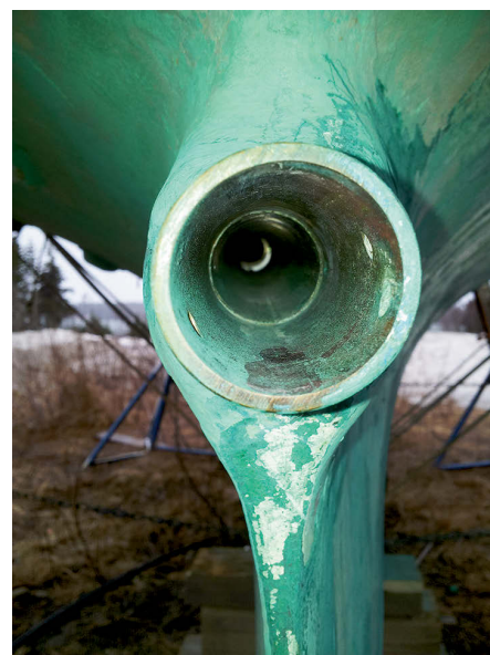
Other areas where the core was rotten were the coachroof, at left, and around the chainplates, center, the latter caused by a poorly sealed fuel fill. Sighting along the stern tube solved the shaft-alignment puzzle — the tube had a bend in it, at right.
