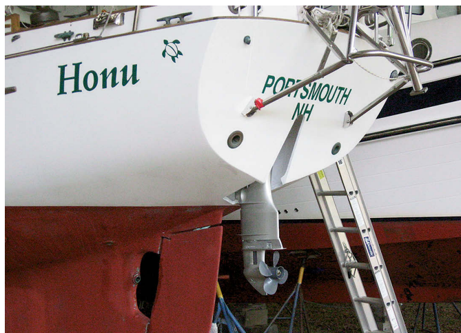
James fitted this Able 32 with a motor well with a 15-horsepower motor. The aperture for the original prop was later filled.
