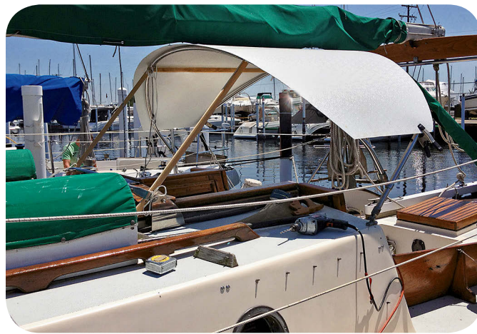
Charles cut the FRP sheet a little over size, at left, so he could play with the height of the dodger and the width of the hardtop. He also adjusted the height of the frame, at right, to balance the sight lines forward with ease of access into the companionway.
