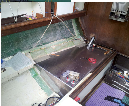
Jon hauled his recently acquired Tartan 34C to replace a seacock, at left, but he discovered other problems that needed his urgent attention. One task was to install a new fuel tank, below.
