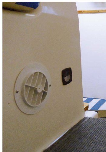
Drew's AC unit was a tight fit under the saloon seat, far left, but there is room to pull it out through the next seat. He mounted this rotatable outlet where it can direct air into the starboard hull or into the saloon, at left.
