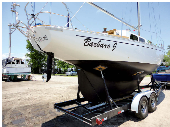
The 9.8-horsepower extra-long-shaft Nissan fits neatly in the completed well, at left. The new mainsheet tackle and 10-inch mooring cleats are also visible. The outboard motor's prop is nearly as low in the water as the original inboard engine's prop, at right. The aperture for the original prop has been filled to reduce drag and improve the efficiency of the rudder.
