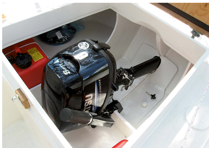
On another Alberg 30, James cut a narrower slot in the hull and transom, at left, for the smaller 6-horsepower motor, at right. The hatch was slightly smaller, so its lid did not require a raised center, and the original traveler was retained.
