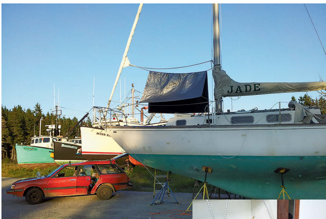
Jon hauled his recently acquired Tartan 34C to replace a seacock, at left, but he discovered other problems that needed his urgent attention. One task was to install a new fuel tank, below.
