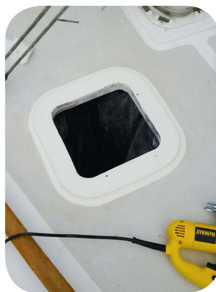
Once he was sure he had all the details right, Matt epoxied the hatch base in place, at left. He applied and faired the gelcoat before cutting the hole, then masked it for protection before making the cut, center. After cleanup, the base was ready to receive the new hatch, at right.
