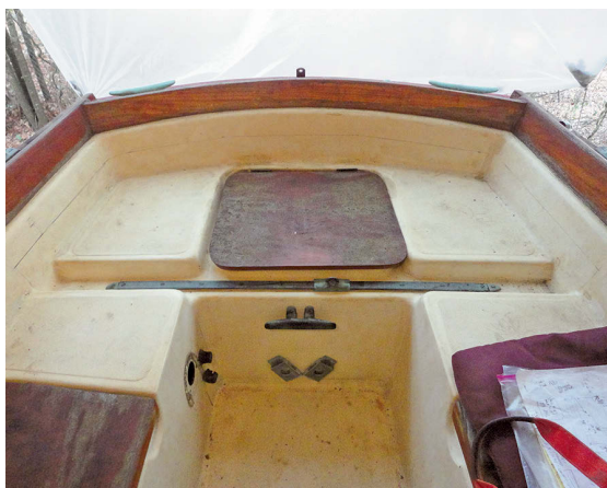
Fitting an outboard well in a Tripp 29 lazarette, top left, required extensive modifications to the cockpit seating and the lazarette area, second left. The finished outboard well, third left, is tidy, includes storage space for gas cans, and takes advantage of the ample transom overhang of the Tripp 29, bottom.
