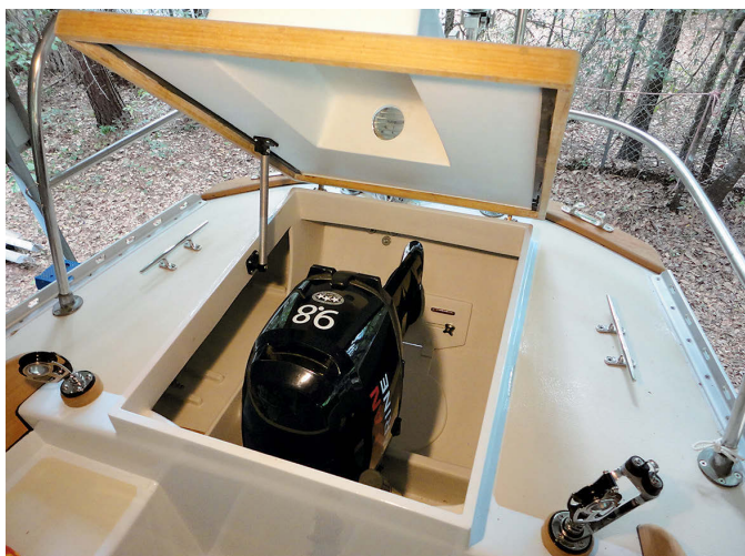
The 9.8-horsepower extra-long-shaft Nissan fits neatly in the completed well, at left. The new mainsheet tackle and 10-inch mooring cleats are also visible. The outboard motor's prop is nearly as low in the water as the original inboard engine's prop, at right. The aperture for the original prop has been filled to reduce drag and improve the efficiency of the rudder.
