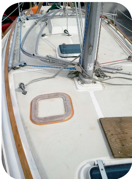
Once he was sure he had all the details right, Matt epoxied the hatch base in place, at left. He applied and faired the gelcoat before cutting the hole, then masked it for protection before making the cut, center. After cleanup, the base was ready to receive the new hatch, at right.
