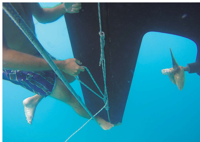
Before dropping the rudder, Robin and his helpers ran a lifting line under it to take the weight, at left. They then wrapped a safety line around the rudder, at right, so they could maneuver it out of the boat and to one side for hoisting it aboard.
