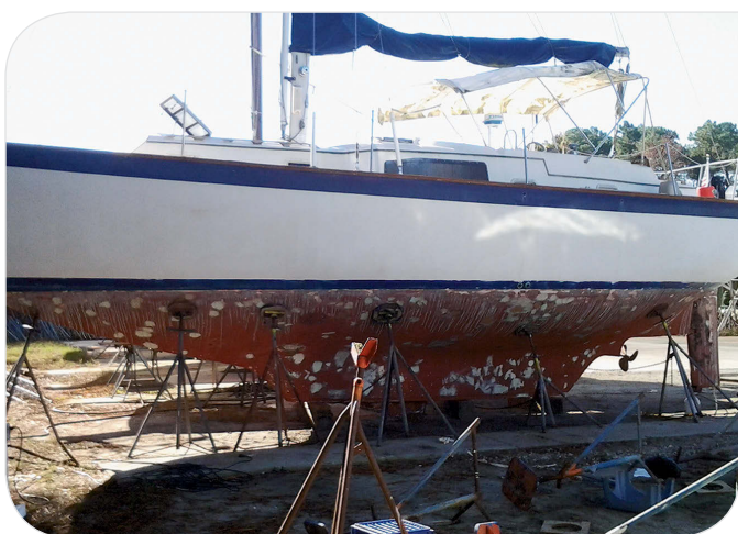
Removing years of marine growth left the bottom looking rough, at left, so the bottom, and the topsides, received fresh coats of paint.
