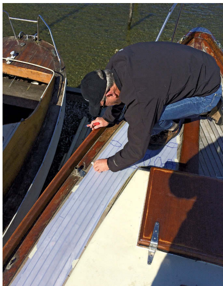
Shipwright Peter Taprell traced the deck edge onto Mylar, at left. The Mylar doesn't have to be an exact fit because tracing around the "fish" establishes the perimeter of the deck with precision, center. The finished tracing of the aft starboard deck has lots of marks, at right.
