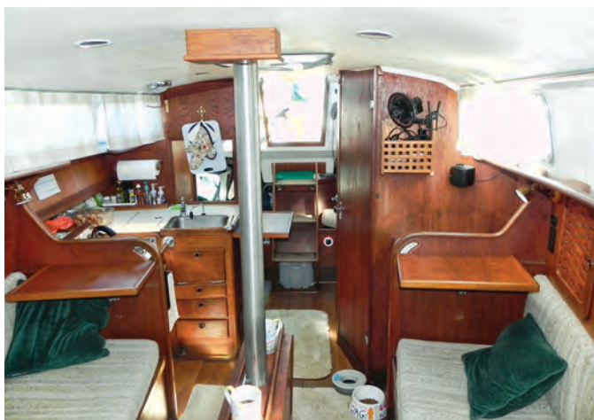
The head is aft of the saloon, on the port side, at left. Two countertops hinged on bulkheads provide extra counter space for the galley, which lacks it. The saloon has classic symmetry, at right, and passage is relatively easy on either side of the centerline drop-leaf table. The numerous storage bins, compartments, and drawers are a mark of a boat of above-average quality.
