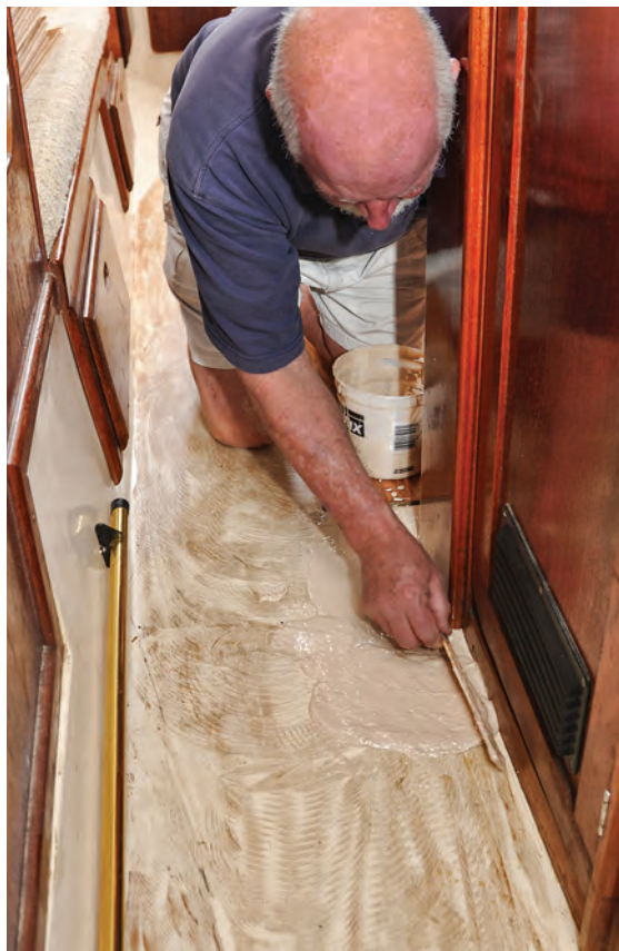
Working in tight quarters, Bill prepares to lay the sole next to the head compartment, at left. Bricks weigh down the boards while the epoxy sets, at right. Genie marks the boards after Bill has cut them to fit, below left. Bill applies epoxy to a board prior to setting it in place, below right.
