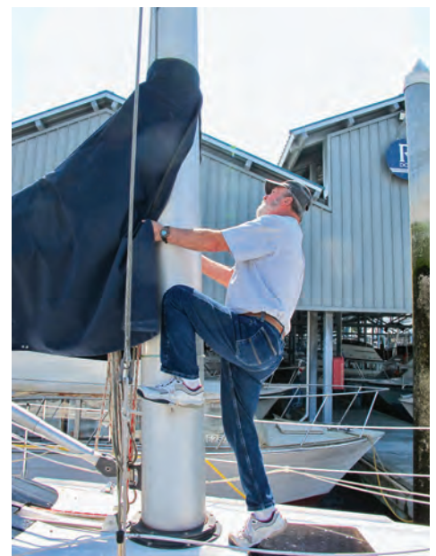
Two steps are fitted on the mast to allow crew to reach the mainsail's halyard shackle and work with the sailcover.
