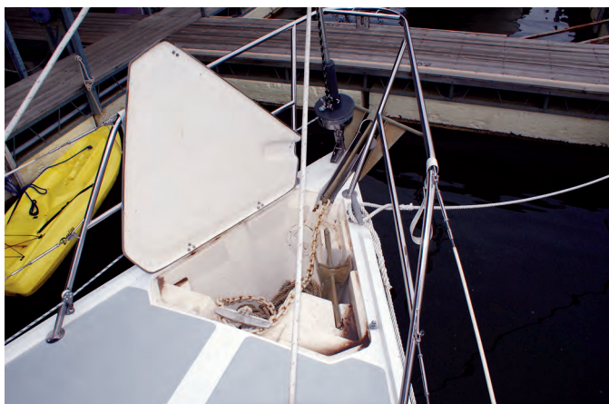
The anchor locker, at left, holds a second anchor and rode but makes fitting a windlass difficult. The T-shaped cockpit, at right, allows easy movement around the pedestal. Note the rudder head under the helm seat where it's accessible if there is a need to fit an emergency tiller.
