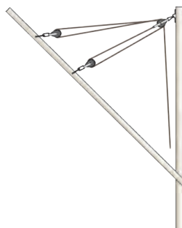
Sometimes, instead of using a bridle, the peak halyard is fastened directly to the gaff. This peak halyard has a 4:1 mechanical advantage.
