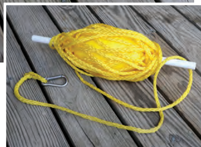
Polypropylene line, a small float, and a length of PVC pipe make an adjustable-depth anchor marker.
