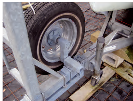
A steel sleeve attached to the trailer's hitch beam, at left, accommodates a 9-foot hitch extension. The Z-shaped mounting arm, at right, allows the spare wheel to double as a hitch jack, and a much more robust one than the standard equipment.
