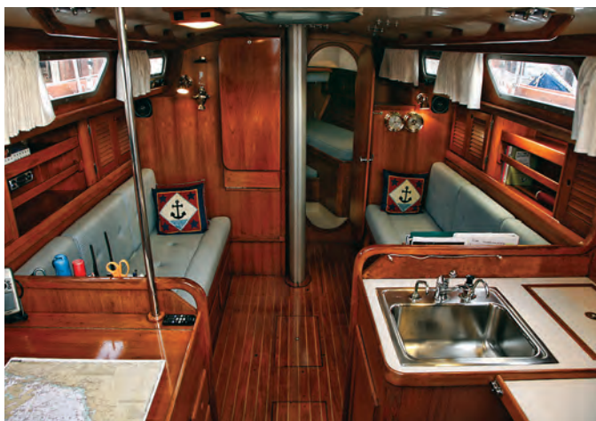
Bristol Yachts finished the interior of the 35.5 in teak and did not stint on cabinetry. Note that the centerboard trunk is entirely beneath the cabin sole, at left. Fixed portlights and the Browns' custom companionway let in plenty of light, at right.
