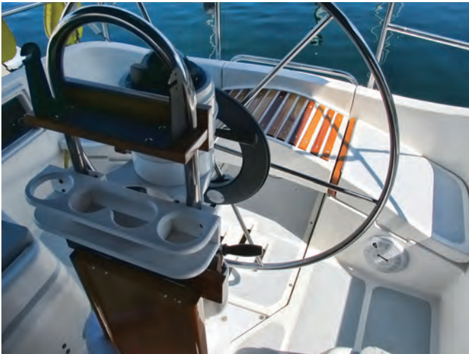
The arched helm seat, at left, provides support for the helmsman when the boat is heeled and lifts up to provide access to the transom-mounted swim ladder. The T-shaped cockpit allows easy movement around the steering wheel, at right, but the seats are too short to lie down on.
