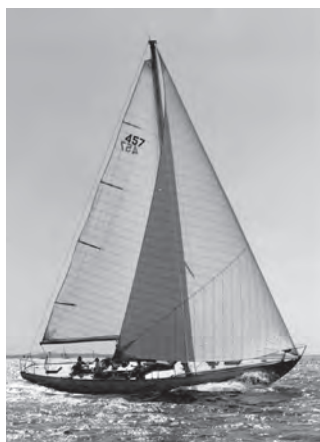
Touché , at left, designed by Bill Tripp Jr., shows the long bow overhang and squat sail plan encouraged by the CCA rule. Even when reefed, The NE 38 , also designed by Tripp, carries a big overlapping genoa, at right. The famous Finisterre , below, gets a big push from her "free" mizzen staysail.
