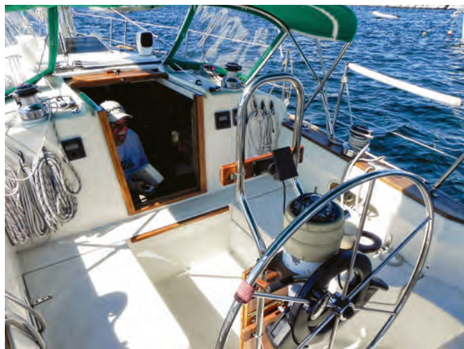
The cockpit is spacious enough and has high comfortable backrests, but Trilogy's aft-cabin arrangement comes at the expense of cockpit length, so the seats are not long enough to nap on.
