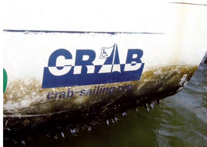
Not pretty, but pretty impressive. St. Brendan's deck and fittings show the effects of 10 months at sea, at left. Inch-long barnacles and a slimy waterline, at right, are the natural accumulation on St. Brendan's hull during her long voyage.
