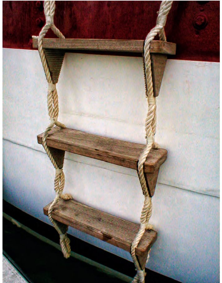
Sigfrid's boarding ladder looks salty, is easy to climb, and its rope risers don't clunk on the hull or abrade the paint.
