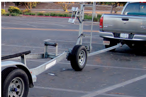
With the spare wheel taking the weight of boat and trailer, above, the hitch extension (which nets at about 9 feet) keeps the tow vehicle away from the water. The extension is equipped with its own 1 7/8-inch hitch/ball arrangement and stores snugly next to the trailer's outside frame and trailer-bunk uprights, at right.
