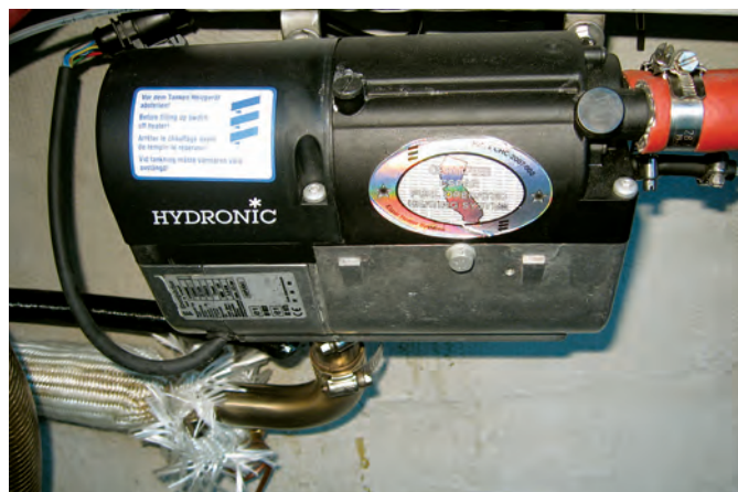
The larger radiator warms the saloon, at left. It's under the aft leg of the U-shaped settee and draws air from the galley. The Espar heater, above, is installed aft under the cockpit. It draws combustion air from the cockpit locker and the exhaust exit is in the transom.
