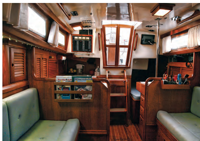
Bristol Yachts finished the interior of the 35.5 in teak and did not stint on cabinetry. Note that the centerboard trunk is entirely beneath the cabin sole, at left. Fixed portlights and the Browns' custom companionway let in plenty of light, at right.
