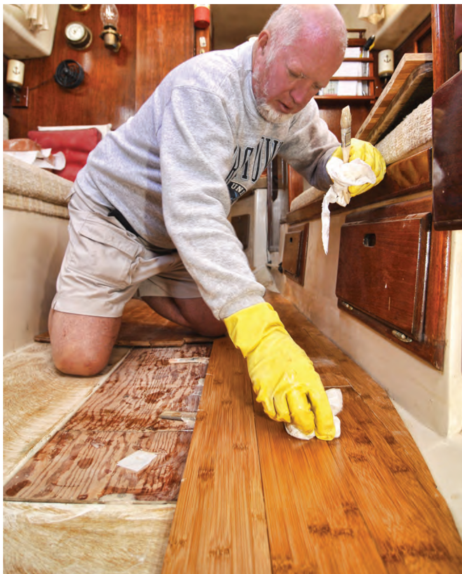
Once the tongue-and-groove pieces of flooring are in place, a tap with a hammer ensures a tight fit, above. Bill wipes up errant epoxy with vinegar, below.
