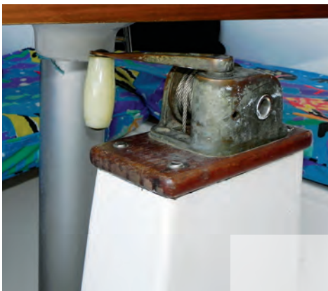
The swing keel's winch is easier to operate with the table removed, above, but Steve raises and lowers the keel with the table in place. A quarter berth is to starboard, near right, and the bulkhead gives the V-berth privacy, far right.
