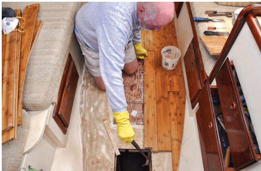
Once the tongue-and-groove pieces of flooring are in place, a tap with a hammer ensures a tight fit, above. Bill wipes up errant epoxy with vinegar, below.
