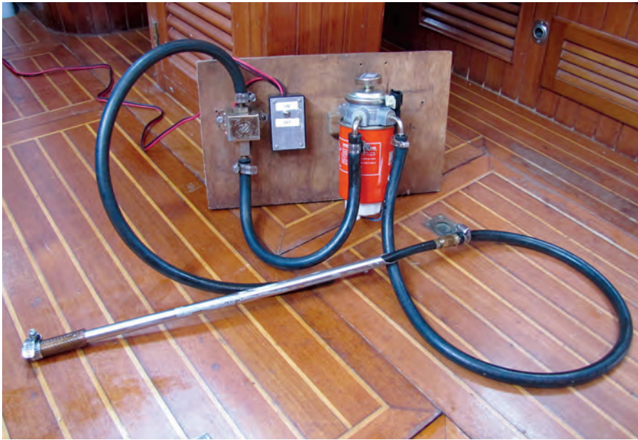
David's fuel-polishing system, shown at left with the Kia fuel filter and below with the Racor filter, is portable, making it more versatile than a hard-plumbed system.
