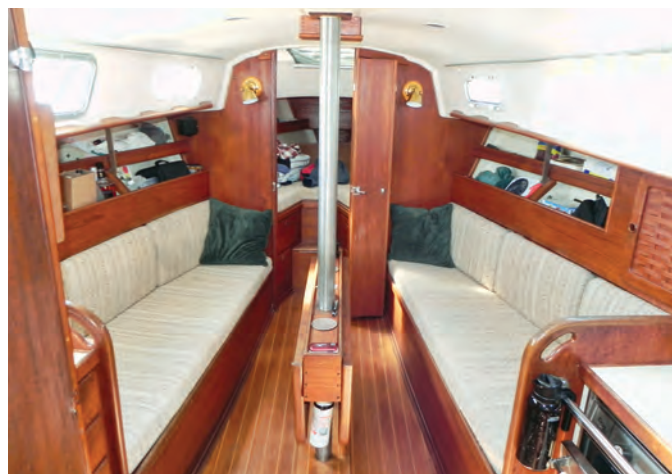
The head is aft of the saloon, on the port side, at left. Two countertops hinged on bulkheads provide extra counter space for the galley, which lacks it. The saloon has classic symmetry, at right, and passage is relatively easy on either side of the centerline drop-leaf table. The numerous storage bins, compartments, and drawers are a mark of a boat of above-average quality.
