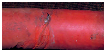
The raw-water supply hose to the engine was chafed almost through where it passed through the bulkhead.
