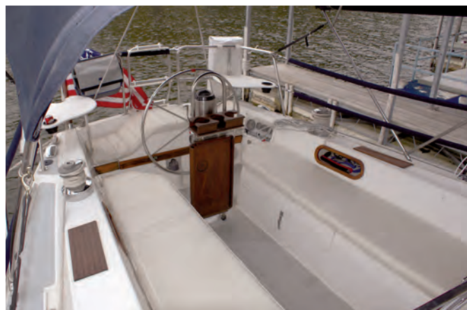
The anchor locker, at left, holds a second anchor and rode but makes fitting a windlass difficult. The T-shaped cockpit, at right, allows easy movement around the pedestal. Note the rudder head under the helm seat where it's accessible if there is a need to fit an emergency tiller.
