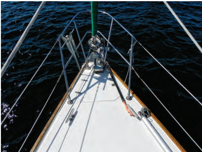
The foredeck is relatively clean, at left, with twin cleats for docklines and ground tackle, a bow roller for the plow anchor, and a small anchor locker. Fred installed the windlass, just forward of the locker. The twin lazarette hatches provide storage space for deck gear such as fenders and docklines, at right. The engine control panel is under the starboard hatch.
