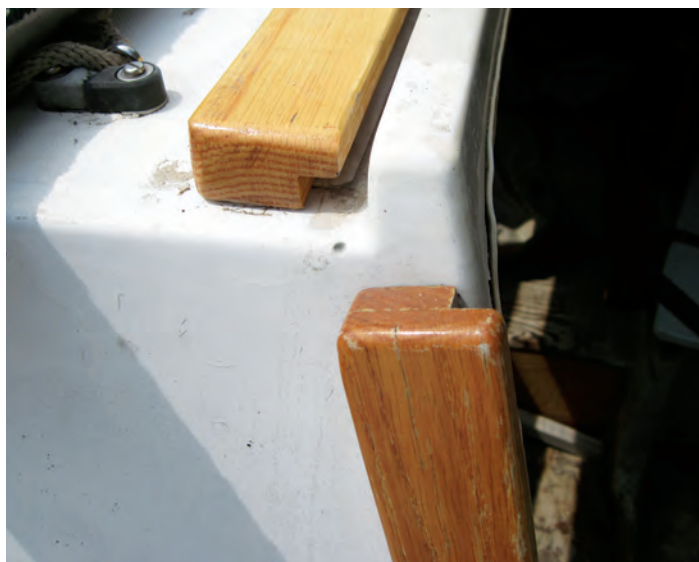
The hatch guide on the cabintop is made from a single piece of wood. The hatchboard guides are two pieces glued together.
