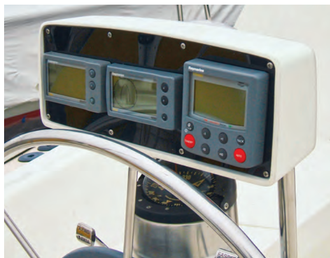
... to accommodate his autopilot control and sailing instruments.
