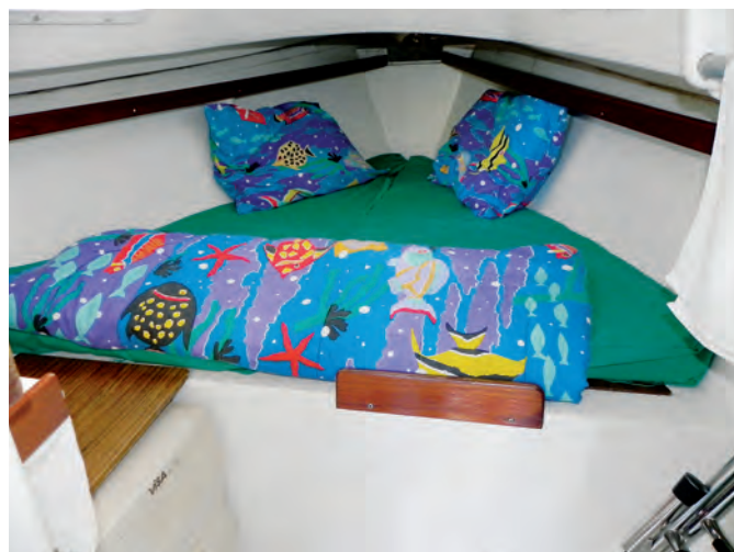
Teak trim and laminates soften the cold whiteness of the molded fiberglass pan and headliner, at left. The trunk for the swing keel is easily visible but it's not as intrusive as it might seem. A portable toilet can be fitted between the main bulkhead and the V-berth, at right.
