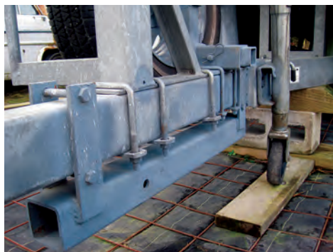
A steel sleeve attached to the trailer's hitch beam, at left, accommodates a 9-foot hitch extension. The Z-shaped mounting arm, at right, allows the spare wheel to double as a hitch jack, and a much more robust one than the standard equipment.
