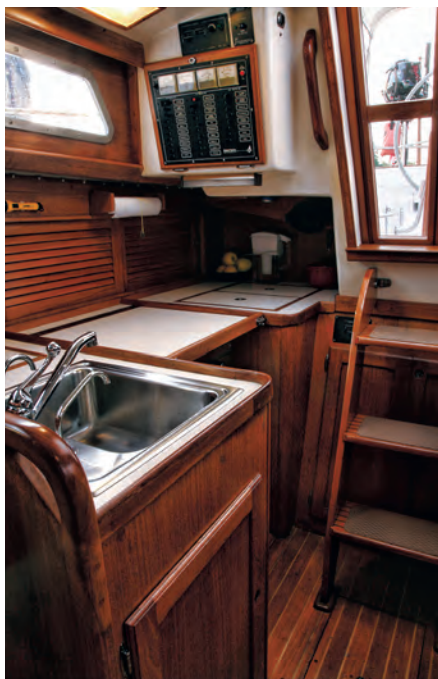
The interior layout is standard for a boat of the era and functional, with the galley to starboard of the companionway, at left, and the head, at right, forward of the saloon.
