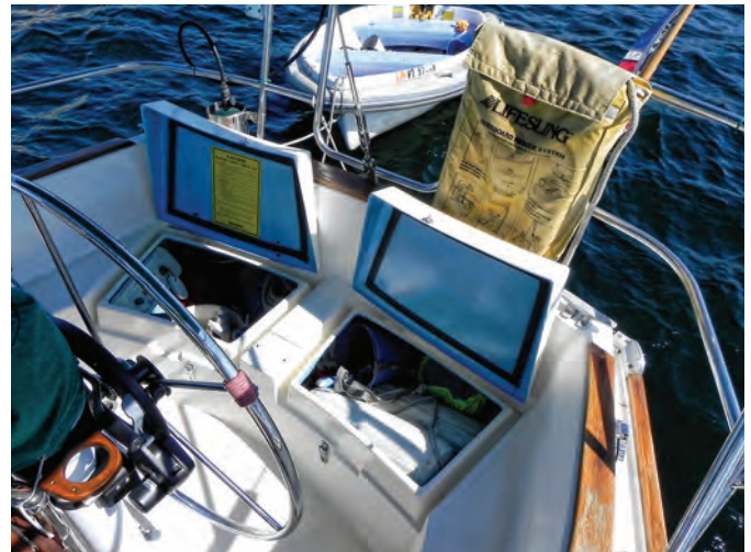
The foredeck is relatively clean, at left, with twin cleats for docklines and ground tackle, a bow roller for the plow anchor, and a small anchor locker. Fred installed the windlass, just forward of the locker. The twin lazarette hatches provide storage space for deck gear such as fenders and docklines, at right. The engine control panel is under the starboard hatch.
