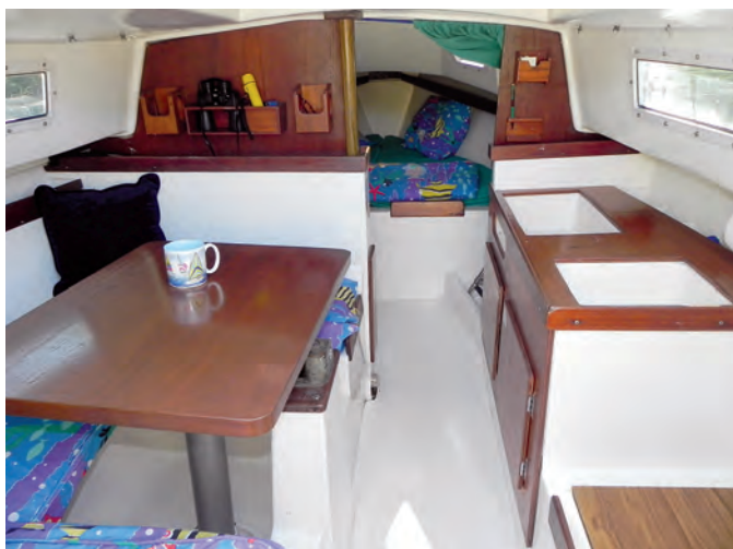
Teak trim and laminates soften the cold whiteness of the molded fiberglass pan and headliner, at left. The trunk for the swing keel is easily visible but it's not as intrusive as it might seem. A portable toilet can be fitted between the main bulkhead and the V-berth, at right.
