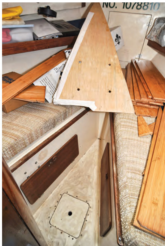
Bamboo flooring made for homes might not have a traditional “yachty” appearance but it looks great just the same, on facing page. The pattern for the sole in the V-berth cabin was the only piece small enough for Bill to conveniently make at home, at left. After a trial fit, at right, he was ready to cut the bamboo boards.
