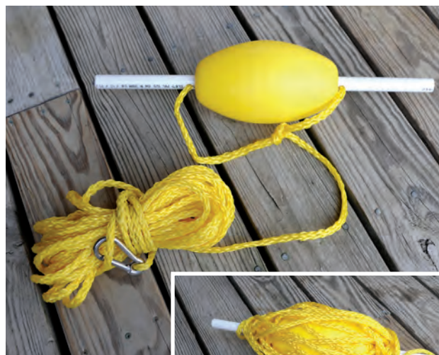
Polypropylene line, a small float, and a length of PVC pipe make an adjustable-depth anchor marker.
