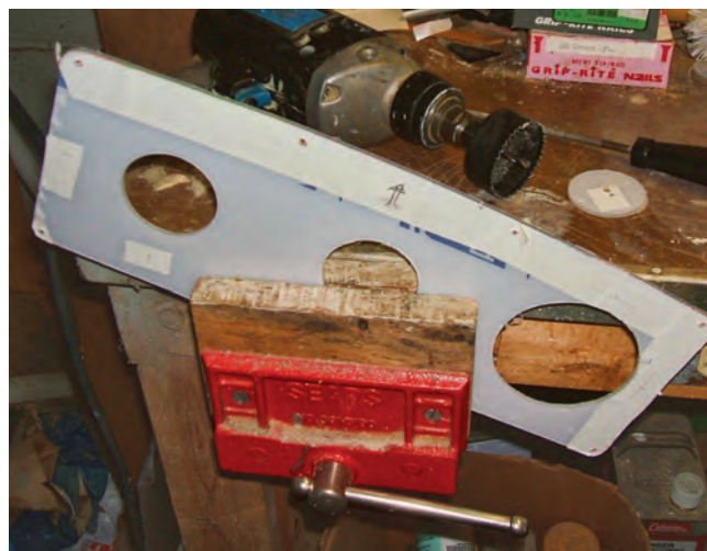
... so he made a new faceplate out of clear polycarbonate ...
