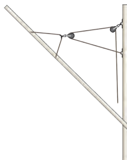
As the gaff is raised into a more vertical position the peak halyard changes its position on the gaff bridle. This is often accomplished by using a gaff bridle saddle.
