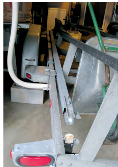
With the spare wheel taking the weight of boat and trailer, above, the hitch extension (which nets at about 9 feet) keeps the tow vehicle away from the water. The extension is equipped with its own 1 7/8-inch hitch/ball arrangement and stores snugly next to the trailer's outside frame and trailer-bunk uprights, at right.
