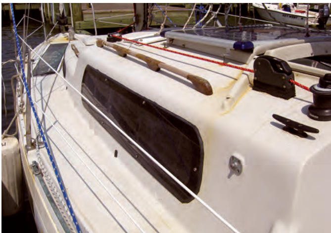
Large deadlights like those in the Vega's cabin trunk, at left, are sometimes vulnerable in bad sea conditions, so Matt and the CRAB crew fitted them with Lexan storm covers. The perpetually damp atmosphere belowdecks caused anything metal to corrode, at right.
