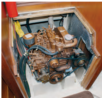
The Universal diesel is easily serviced from the space just beneath the companionway stairs.
