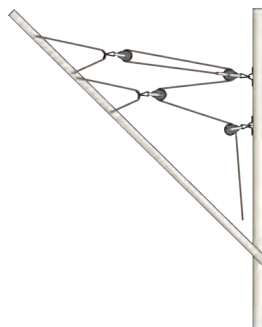
The peak halyard of this heavier gaff is attached using two bridles and has a 4:1 mechanical advantage.
