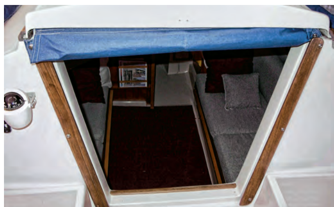
Dan's soft "hatchboard" provides privacy, keeps out rain, and is a lot easier to manhandle than a wooden board.
