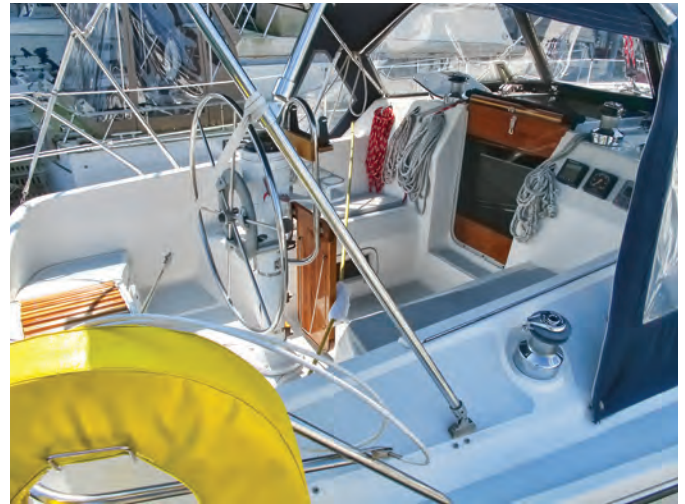
The arched helm seat, at left, provides support for the helmsman when the boat is heeled and lifts up to provide access to the transom-mounted swim ladder. The T-shaped cockpit allows easy movement around the steering wheel, at right, but the seats are too short to lie down on.
