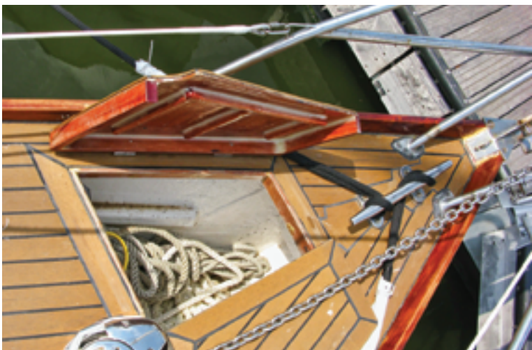
Among the many additions Stephen made to the Vera May was the anchor locker, at left. He also installed the windlass. He went his own way with the lifelines, at right, making them of high-tech synthetic fibers instead of the traditional stainless-steel wire cable.
