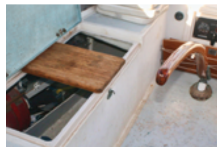
In the unused space above the galley storage, Bruce fitted a fiddled shelf, at left, that hinges down to give access to its contents, center. His cutting board fits over the galley sink and doubles as a seat that lets him face forward while steering, at right
