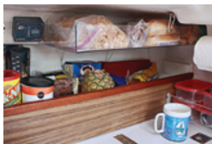
In the unused space above the galley storage, Bruce fitted a fiddled shelf, at left, that hinges down to give access to its contents, center. His cutting board fits over the galley sink and doubles as a seat that lets him face forward while steering, at right
