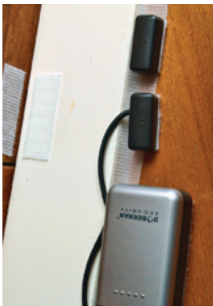
A magnetic-switch alarm that connects the switch to the alarm unit with a wire, at left and center, allows some flexibility with the installation as the alarm can be mounted out of the way of the entrance. This model is operated by a remote control, at right.
