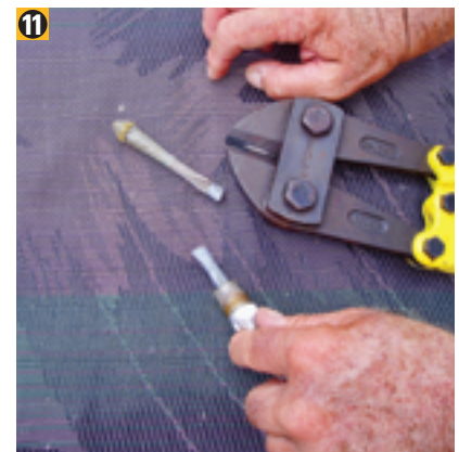
11 To remove the terminal socket from the old stay, cut the wire.
