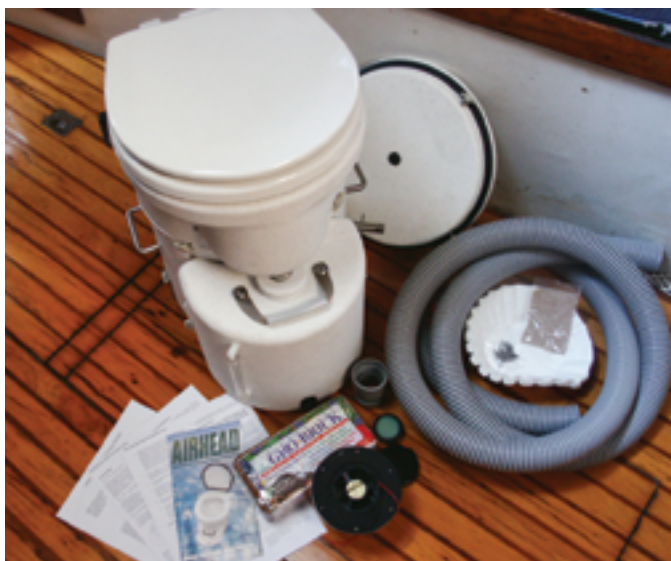
One Air Head kit complete, some assembly required, above left. It included the vent hose, various fittings and consumables, and the cover for transporting the compost tank. The inverted bowl component, above right, shows the liquids conduit, at the left, and the trapdoor (its lever is at the lower right). Venting is aided by a 12-volt fan in a shroud, which Dave mounted beneath a Dorade, bottom of page.
