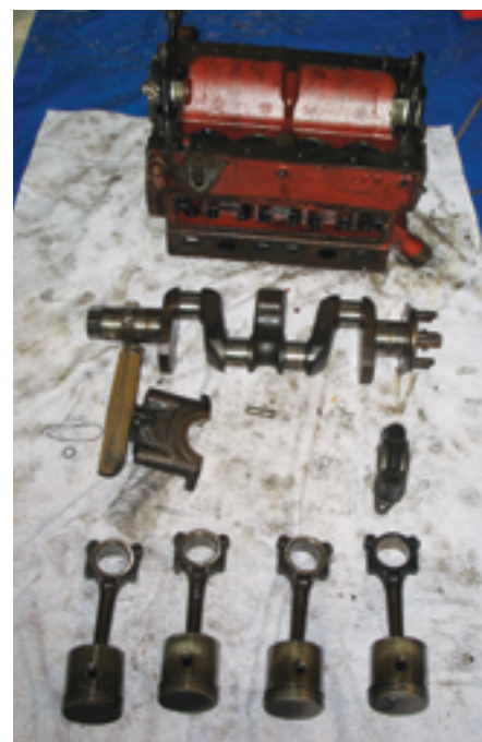
New pistons and the crankshaft with its freshly machined journals await assembly into the refurbished engine block.
