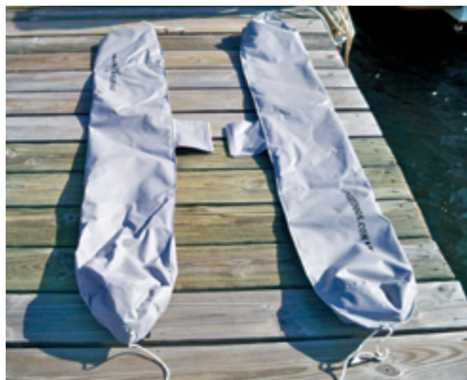
Dinghy Dogs are separate tubes that fit on each side of a dinghy's hull to provide additional buoyancy.
