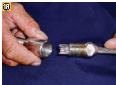
Thread the female terminal end onto the socket and draw it up hand tight.
