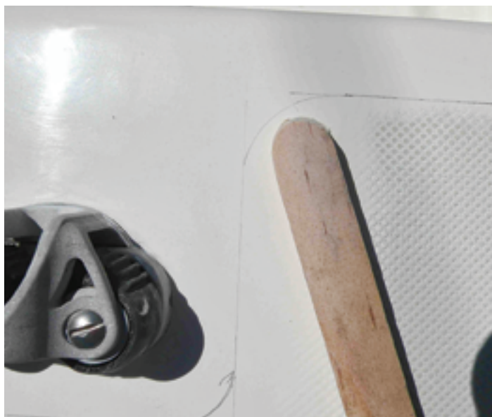
Stephen made special sanding blocks so he could work right up against hardware items that stayed in place, above. Another sanding block let him sand down the old non-skid up to the pencil lines, below.
