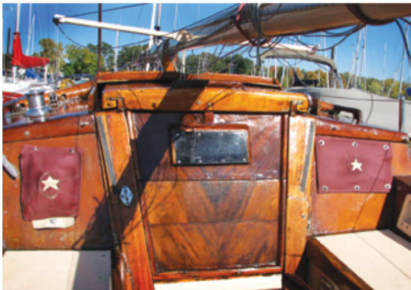
The covers match up on both sides of the companionway. A set of twist-lock fasteners atop the cabin allows the cloths to be unbuttoned at the bottom and folded up to reveal the instruments when they are needed.
