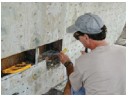
To prevent water from lingering in the bilge, Randy chiseled out a small sump to hold a pair of bilge pumps, at left. The rebuild began with fiberglass laid from the inside against a form, at right.
