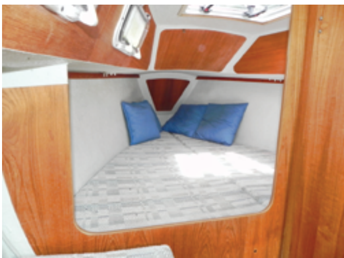
Despite the 2023's short length, the V-berth is a generous 82 inches long x 72 inches wide, at left. Interior joinery is built with teak-veneer plywood, nicely oiled for an attractive appearance. The number of opening portlights varied by boat, at right.
