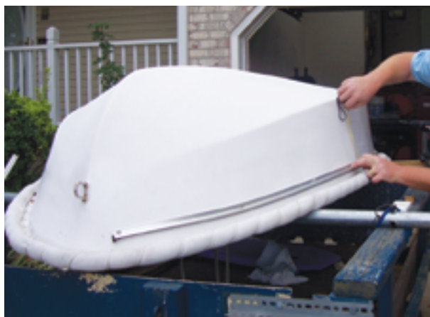
To accommodate the fuller bow of the Dyer knockoff, Frank had to bend the aluminum mounting tracks.
