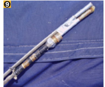
9 Tape the old wire, with the wedge still in place, to the new wire.
