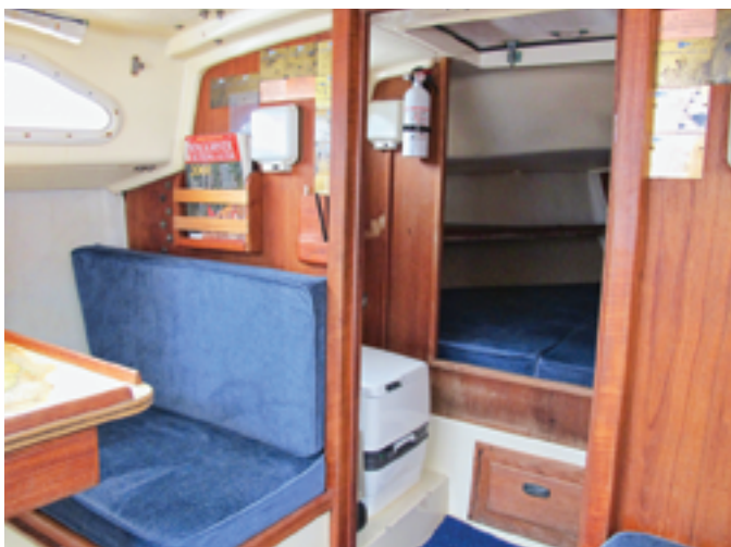
Bandit's racing honors, garnered under several owners, adorn the main bulkhead, at left. Forward is the small head compartment and spacious (for this size boat) V-berth. The dinette in the saloon, at right, is well lit by the fixed ports in the cabin trunk and converts to a double berth.
