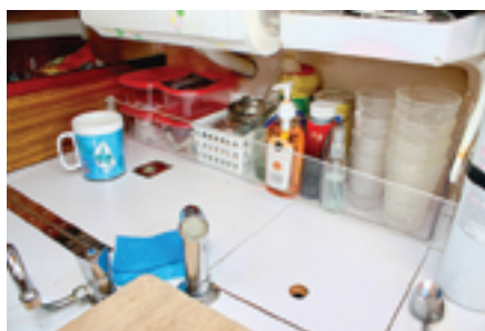
On both sides of the galley, Bruce fenced off counter space to hold items he uses often, by the stove, at left, and near the sink, center. A removable fiddle extension, at right, keeps utensils from jumping out when the boat is sailing hard.
