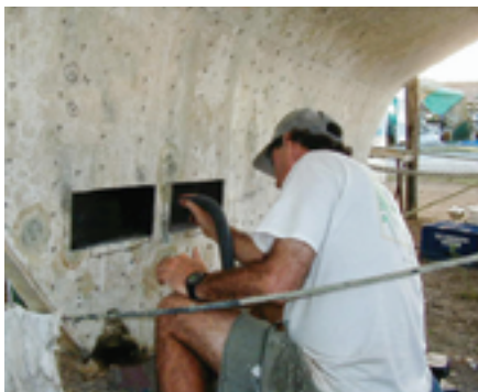
Cutting into it from outside the hull revealed the black truth that was the inside of the bilge, at left. Before going any further, Randy and Cheryl had to clean it out, at right.
