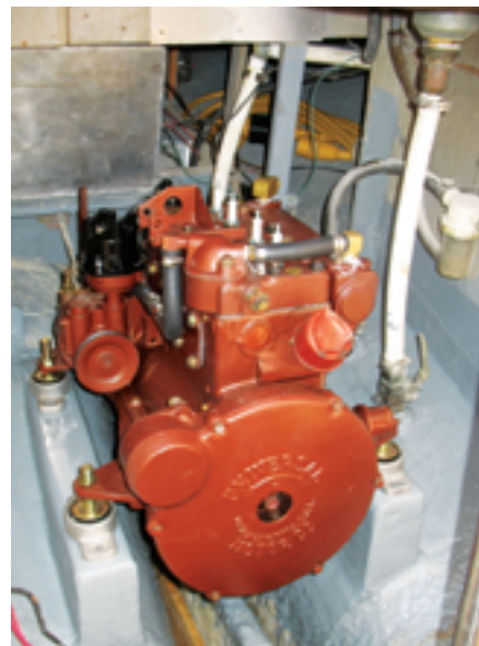
Lifted by the boom once more, at left, the rebuilt engine made the return journey to its home under the cockpit, where it joined the new aluminum fuel tank and cockpit-drain seacocks, at right. Trillium looks ready to put another 39 years on her engine, below.
