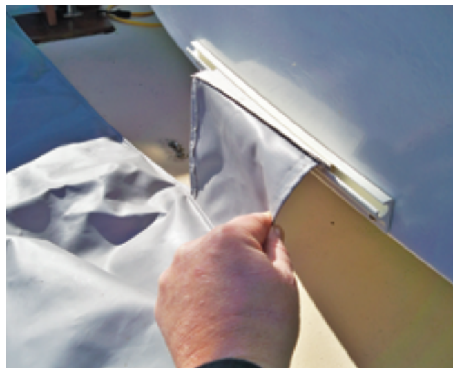
Dinghy Dogs attach to cleats at the bow and stern of the dinghy and are held down by a short tab in a track.
