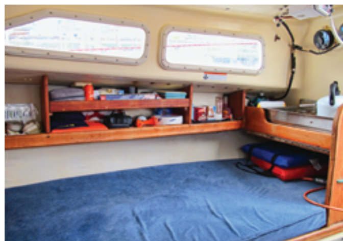
The galley in the Ranger 26 is quite minimal. The small sink is hard against the aft bulkhead on the port side, at left, and the stove is opposite on the starboard side, at right. The starboard settee extends under the stove, and shelves above it provide storage for sundry items.
