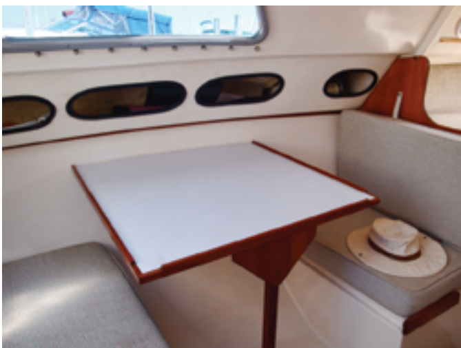
The dinette, on the port side of the saloon, at left above, converts to a double berth. Oval storage compartments above it have a shippy look while saving construction weight. The compact galley, at right above, is an example of how the Clark Boat Co. employed advanced manufacturing techniques. Aft of the galley is a quarter berth, below. A portable toilet is kept behind the companionway step.
