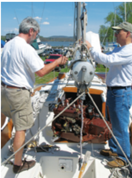
Lifted by the boom once more, at left, the rebuilt engine made the return journey to its home under the cockpit, where it joined the new aluminum fuel tank and cockpit-drain seacocks, at right. Trillium looks ready to put another 39 years on her engine, below.
