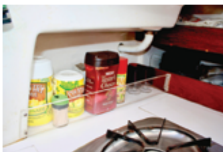
On both sides of the galley, Bruce fenced off counter space to hold items he uses often, by the stove, at left, and near the sink, center. A removable fiddle extension, at right, keeps utensils from jumping out when the boat is sailing hard.
