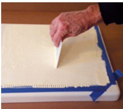
Still using the spreader, Stephen covered the entire surface with an even coating.
