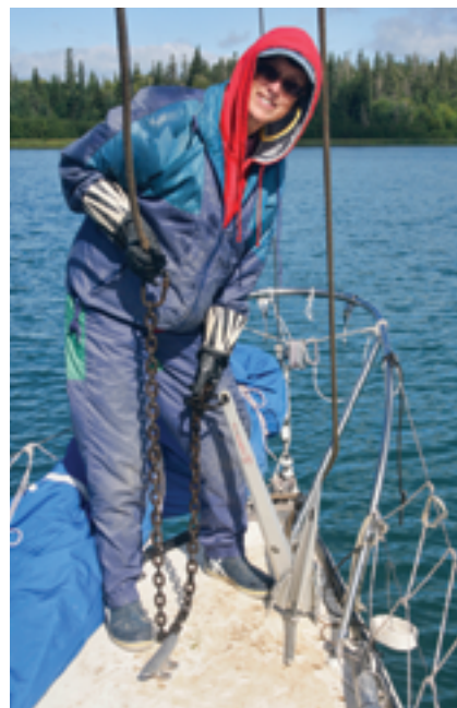
Once the anchor is under the bow, the ascender is attached to the rode and clipped to a halyard, at left. While Jerry (off camera) hoists away on the halyard, Karen, at center, guides the anchor rode until she has the anchor and chain (and a little mud) on deck, at right.
