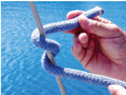
To tie a rolling hitch onto a stay, take two turns around the stay in the direction the load will be applied, at left, cross the end over the standing part, and take another turn, tucking the end under, center and right. Long link plates, bottom right, allow access to the forestay turnbuckle.
