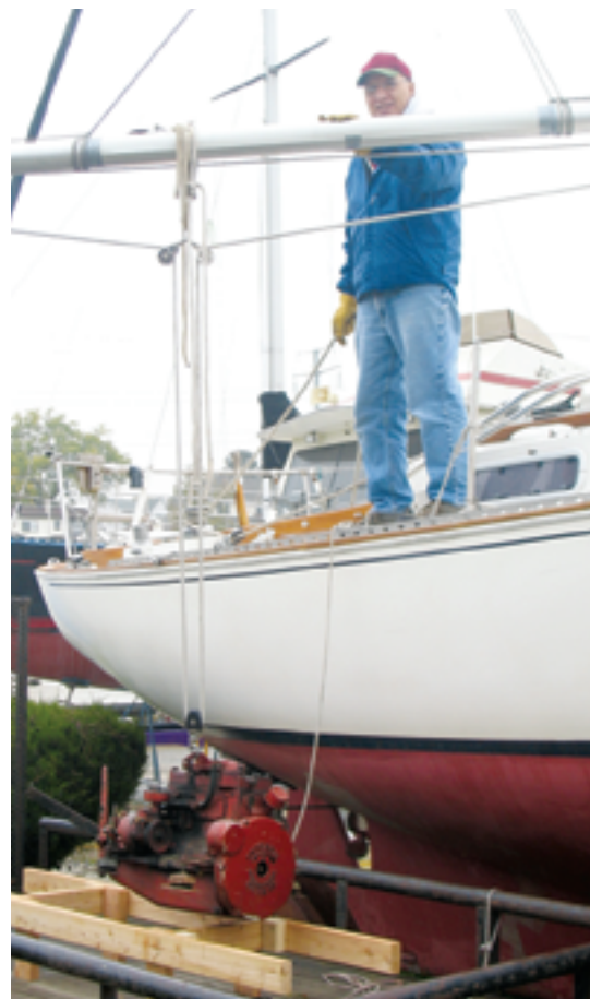
Rob used the boom to lift the engine out of the cabin and lower it to the trailer.
