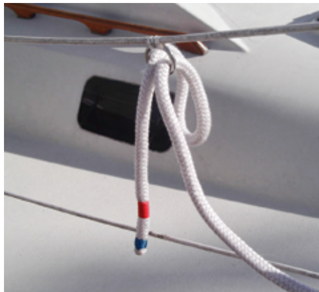
With one end made fast on the boat and the other tucked into a ring on the lifeline, Michael's dockline is set up so a helper on the dock can easily grab it and take it to a dock cleat.
