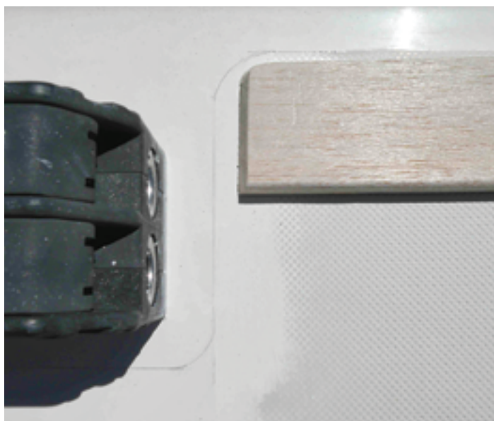
Stephen made special sanding blocks so he could work right up against hardware items that stayed in place, above. Another sanding block let him sand down the old non-skid up to the pencil lines, below.
