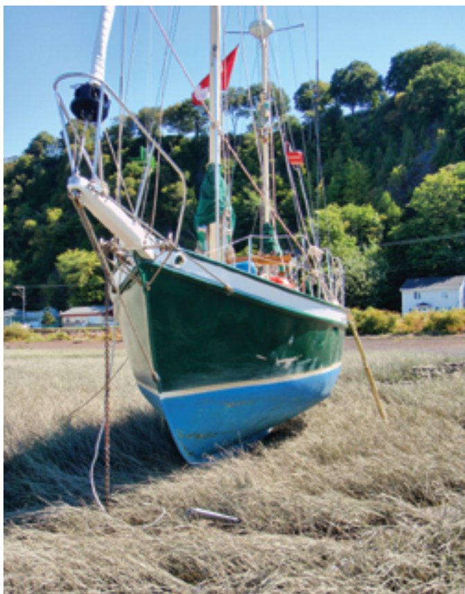
Kuan Yin is a Tahitiana 32, and her long full keel allows her to take the ground very easily, at left. Dennison had the sheer legs aboard, so he was equipped to prop her up. At low tide, the bay looks like a meadow, but at high tide, the grass is completely covered to a depth of five feet, at right.
