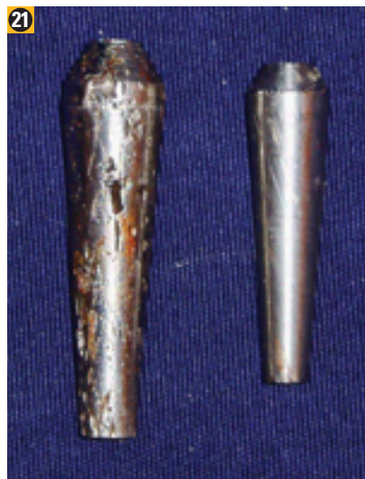
The corroded wedge (left) indicates water ingress into a terminal.
