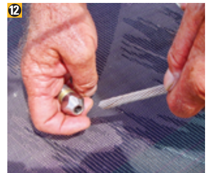
12 Slide the terminal socket off the cut end of the old wire.
