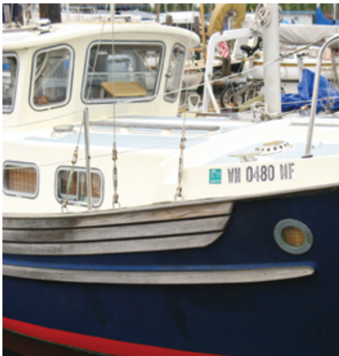
Weathered or bright, with a little care, teak will last for years, as on this 84-year-old San Francisco Bird, above. Bare teak rubbing strakes, below, look shippy, but peeling varnish, below right, suggests neglect.
