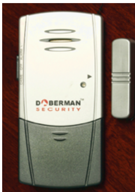
In a typical window alarm, a magnetic switch is held open by an external magnet, at left. When the alarm and magnet are attached to adjacent companionway dropboards, above, the alarm will go off when the upper dropboard is removed.
