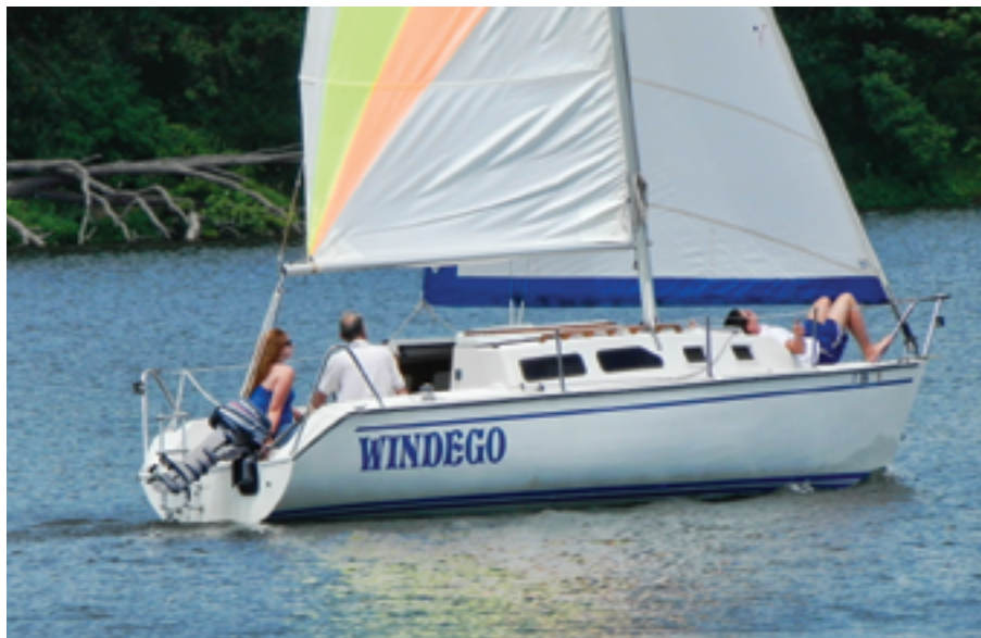
Lest anyone accuse Alex Krinickas of poor sail trim, the luff boltrope on Windego's mainsail has stretched and cannot be properly tensioned.
