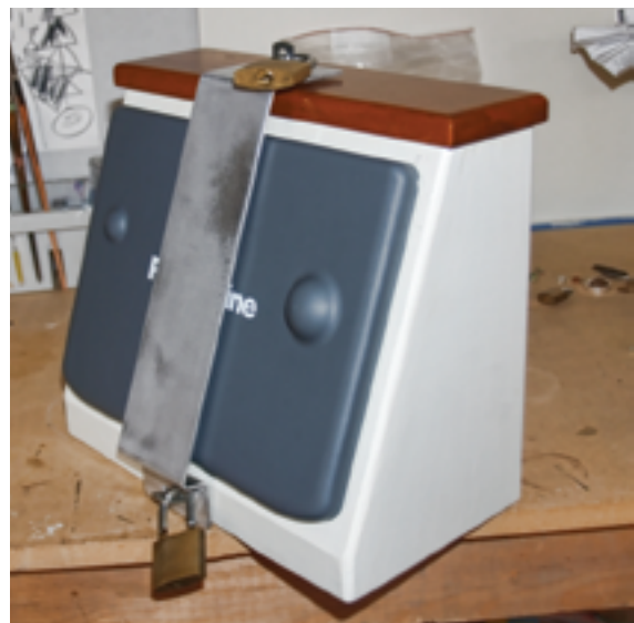
The curved extension, at left, houses the cable plugs. The metal bar and locks, at right, are to deter theft.
