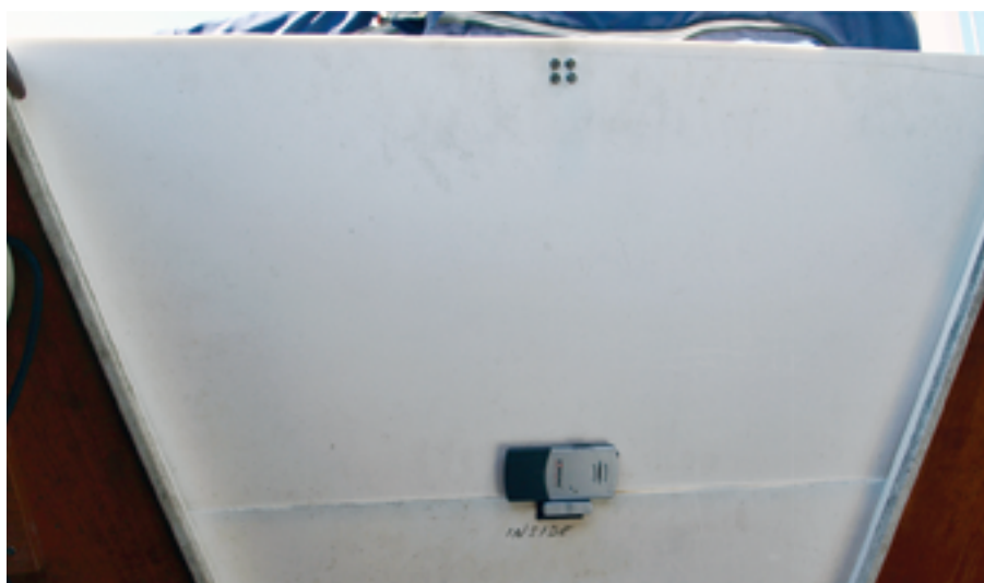
In a typical window alarm, a magnetic switch is held open by an external magnet, at left. When the alarm and magnet are attached to adjacent companionway dropboards, above, the alarm will go off when the upper dropboard is removed.
