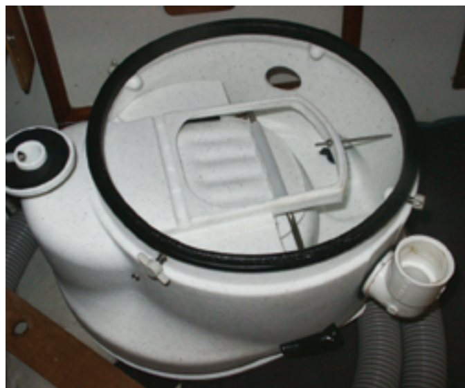
One Air Head kit complete, some assembly required, above left. It included the vent hose, various fittings and consumables, and the cover for transporting the compost tank. The inverted bowl component, above right, shows the liquids conduit, at the left, and the trapdoor (its lever is at the lower right). Venting is aided by a 12-volt fan in a shroud, which Dave mounted beneath a Dorade, bottom of page.
