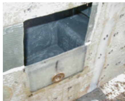
Before closing the hole, Randy lined the inside of the bilge with glass cloth and epoxy, at left. The closure then proceeded in stages, at right. Note the little sump and the drain plug.
