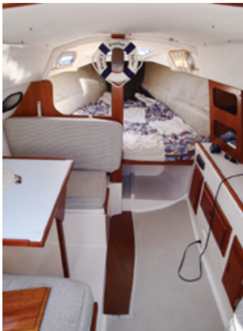
The absence of a full main bulkhead opens up the interior to light and good ventilation.
