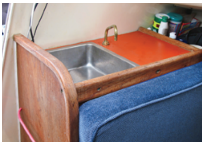
The galley in the Ranger 26 is quite minimal. The small sink is hard against the aft bulkhead on the port side, at left, and the stove is opposite on the starboard side, at right. The starboard settee extends under the stove, and shelves above it provide storage for sundry items.
