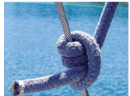
To tie a rolling hitch onto a stay, take two turns around the stay in the direction the load will be applied, at left, cross the end over the standing part, and take another turn, tucking the end under, center and right. Long link plates, bottom right, allow access to the forestay turnbuckle.
