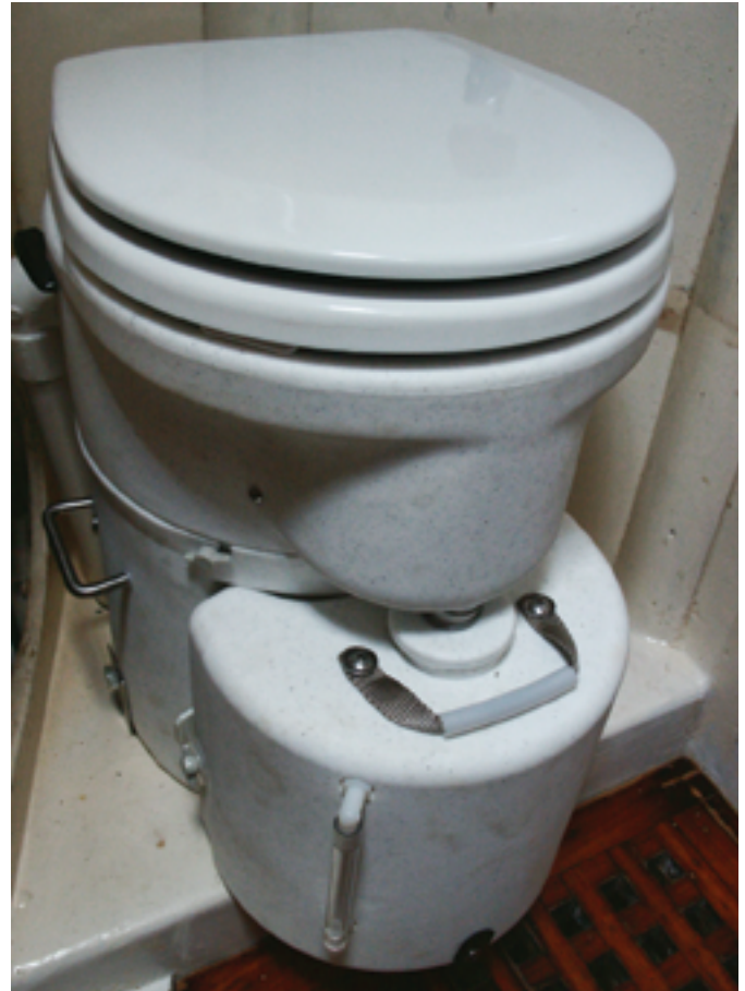
The Air Head is bulkier than a standard marine toilet and a close fit in Eurisko , but it eliminates the need for a holding tank.
