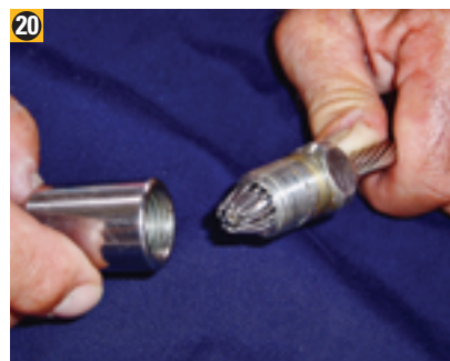
Make the final assembly with sealant and thread-locking compound.
