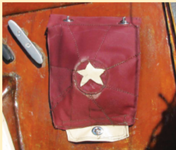
The tanbark-colored compass cover is made of leftover Sunbrella. The star decoration is cream-colored leather scavenged from an old office chair. The eyelet in the leather tab at the bottom can be secured to a twist-lock on the cabintop to expose the compass.
