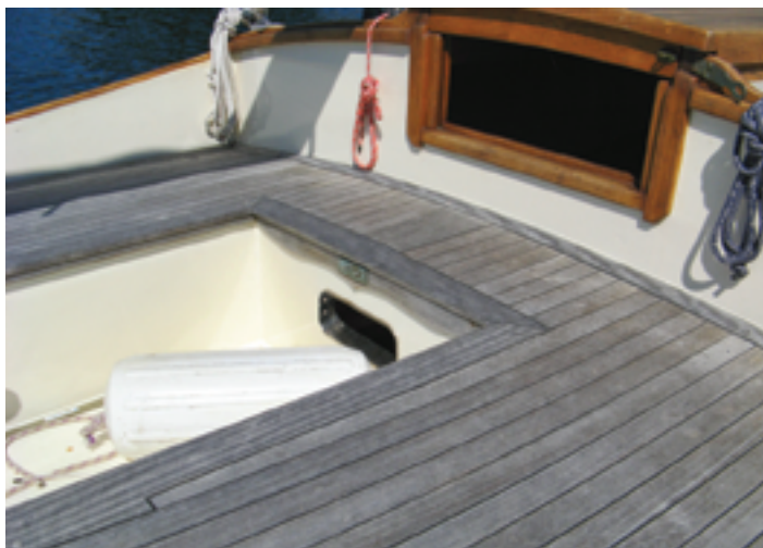
Weathered or bright, with a little care, teak will last for years, as on this 84-year-old San Francisco Bird, above. Bare teak rubbing strakes, below, look shippy, but peeling varnish, below right, suggests neglect.
