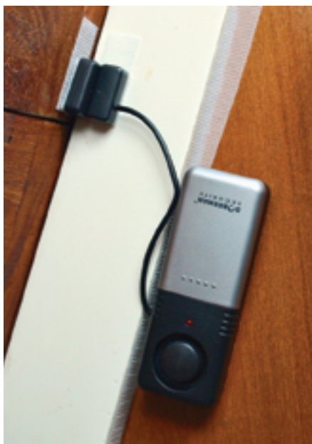
A magnetic-switch alarm that connects the switch to the alarm unit with a wire, at left and center, allows some flexibility with the installation as the alarm can be mounted out of the way of the entrance. This model is operated by a remote control, at right.
