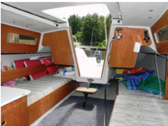
The companionway opening is quite large and, with the low step down, allows easy passage between the cabin and the cockpit, at left. A sliding drawer under the galley counter is designed to hold a small portable ice chest, at right.
