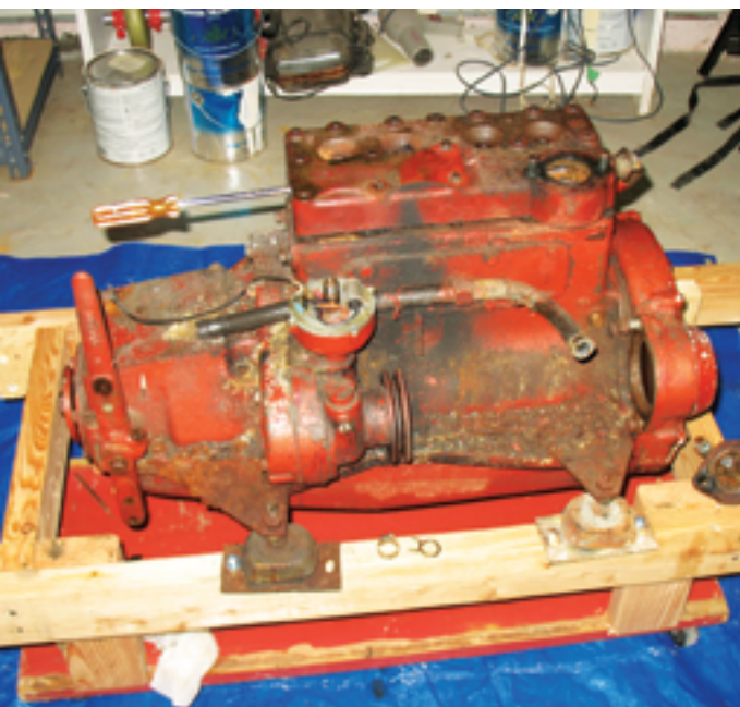
Disassembly of the engine began in the fall with the removal of the cylinder head, at left, and the re-machined head went back on the refurbished block in the spring, at right.
