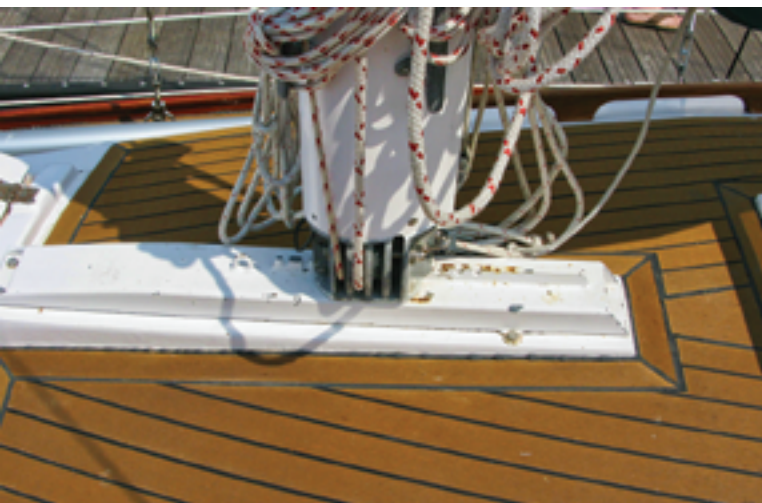
The Mistral's mast is stepped on deck on a raised stiffener that spans two bulkheads, at left. Stephen surfaced the deck with TekDek. Stephen placed mounting pads for a multi-directional fan, at right, throughout Vera May's cabin. The wooden deck beams are structural, not decorative.
