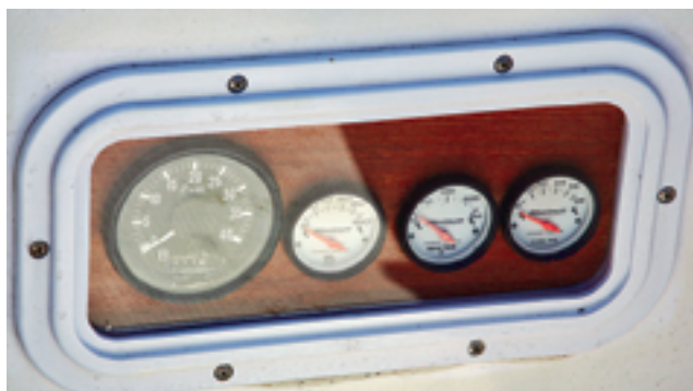
The engine instruments are protected behind a Beckson fixed port mounted in the face of the bridge deck where they are clearly visible from the helm.
