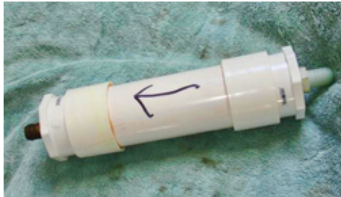
Assembling the filter is easy. The arrow points to the top bushing, which can be removed for recharging the filter.
