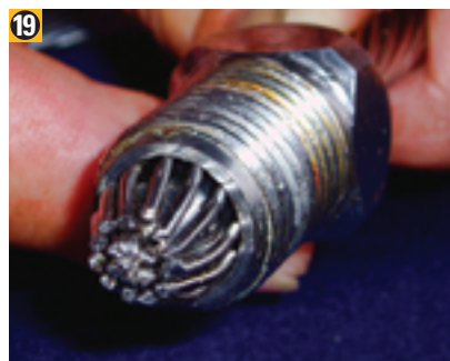
Unscrew the terminal end and examine the assembly for uniformity.
