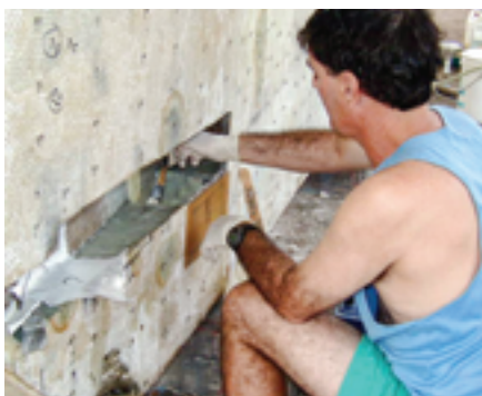
Before closing the hole, Randy lined the inside of the bilge with glass cloth and epoxy, at left. The closure then proceeded in stages, at right. Note the little sump and the drain plug.
