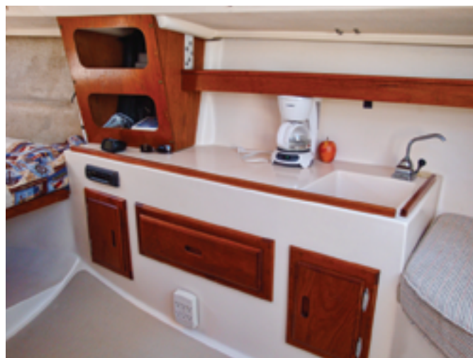
The dinette, on the port side of the saloon, at left above, converts to a double berth. Oval storage compartments above it have a shippy look while saving construction weight. The compact galley, at right above, is an example of how the Clark Boat Co. employed advanced manufacturing techniques. Aft of the galley is a quarter berth, below. A portable toilet is kept behind the companionway step.
