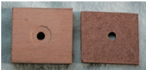
Plywood crushes under pressure but Masonite doesn't, at left. Masonite sandwiched between two layers of plywood makes a sturdy backing plate with cosmetic appeal, at right.
