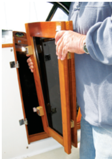
Gary fits the bi-fold doors onto the pintles that serve as hinges, at left. This view from the inside shows the brass hinges and the turn buttons that hold the inserts in place, at right.
