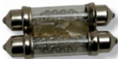
The red and green festoon bulbs are glued together.
