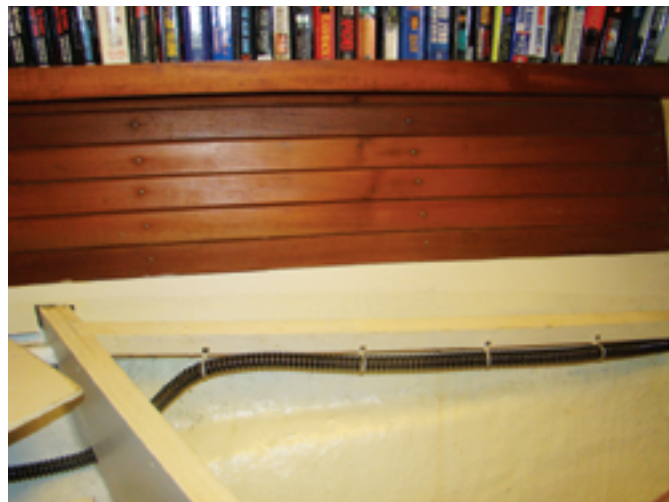
From the head intake, the wash-down supply hose passes through the bulkhead into the forward cabin, to a strainer, then to the pump, at left. The hose continues forward under the berth, at right, and into the chain locker, where it connects to the on-deck hose bib via a pipe extension, below.
