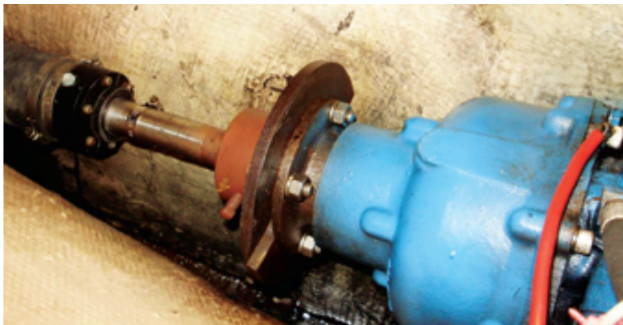
The two halves of the shaft coupling are secured together with four bolts. Use a feeler gauge to check the space between the two halves at 90, 180, 270, and 360 degrees.
