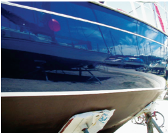
Caribee's reflection in a neighbor boat, which Randy helped paint, shows that a high-gloss finish highlights imperfections of all magnitudes in the surface it covers, from dust specks to unfairnesses bequeathed by the original hull mold, at left above. By repairing nicks, dings, and scratches, though, it's possible to get a finish at least as good as the one that emerged from the factory, at right above.
