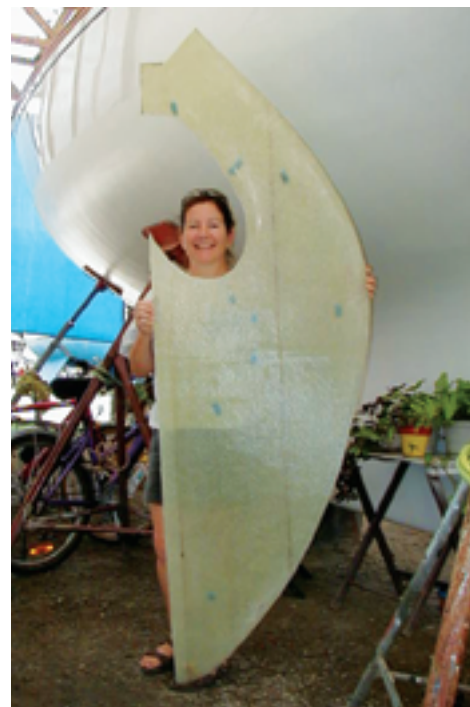
The rudder's backbone is a fiberglass sheet, above left, that is bigger than Cheryl, above right.
