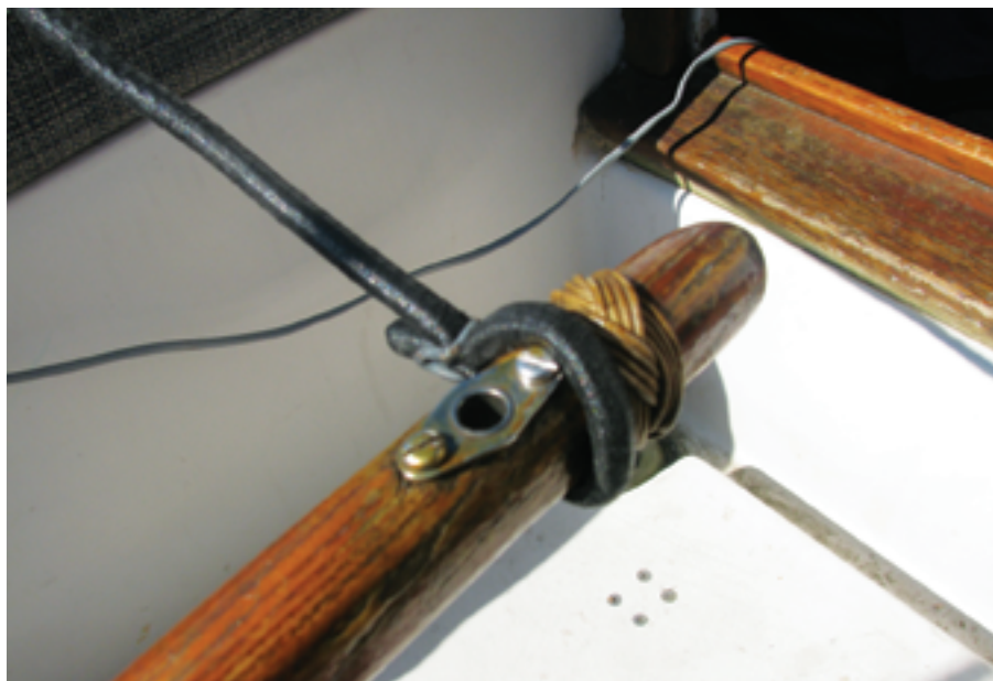
A length of shock cord and a scrap of wood make up a low-budget adjustable steering control, at left and below. A pair of these devices can handle varied conditions, at bottom.
