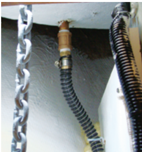
From the head intake, the wash-down supply hose passes through the bulkhead into the forward cabin, to a strainer, then to the pump, at left. The hose continues forward under the berth, at right, and into the chain locker, where it connects to the on-deck hose bib via a pipe extension, below.
