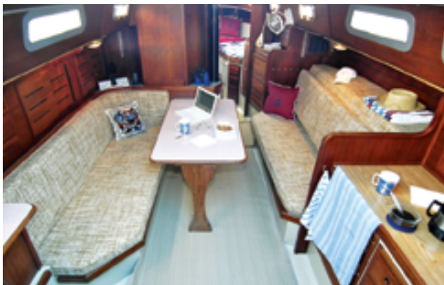
The layout of the Islander 36 broke the mold for sailboat interiors, using a disappearing table and low partitions to create an openness imitated in many designs to this day. Its designer, Joe Artese, also employed angled partitions and bulkheads to make the spaces more interesting.
