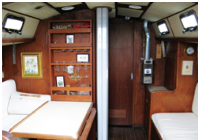
The view from the saloon looking aft, at left, shows a conventional arrangement with the chart table, quarter berth, and wet locker next to the companionway to starboard and the tight U-shaped galley to port. Forward, Duane installed a wood-burning stove to cheer up the already cozy cabin when cruising in the cool Pacific Northwest autumn, at right. The plywood bulkheads are bonded to the hull and deck for strength and stiffness.
