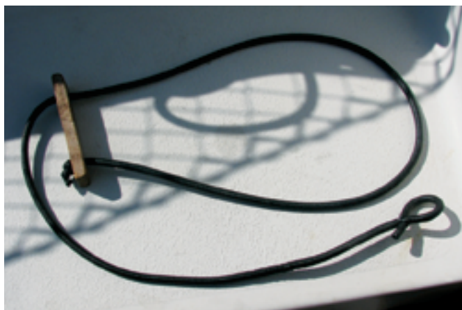
A length of shock cord and a scrap of wood make up a low-budget adjustable steering control, at left and below. A pair of these devices can handle varied conditions, at bottom.
