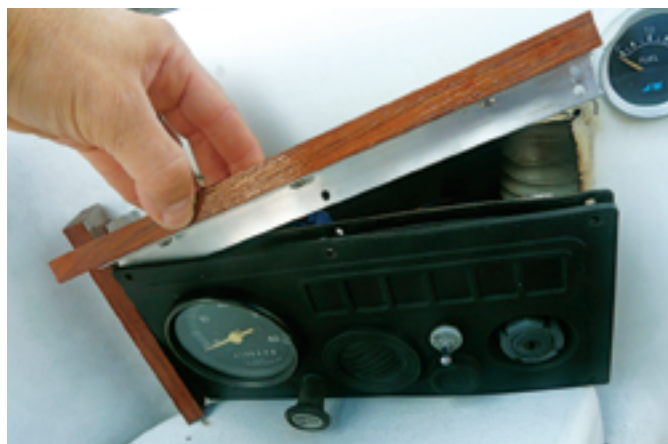
The components await assembly. Chris discarded the parts for one short side because they wouldn't fit next to the fuel gauge.
