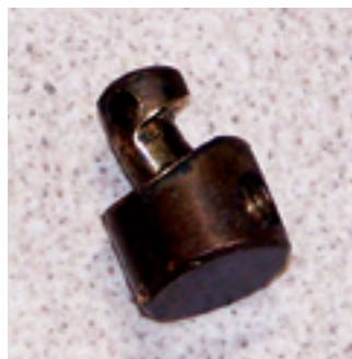
The worn pivot at the throttle-lever connection contributed to the failure of the cable.
