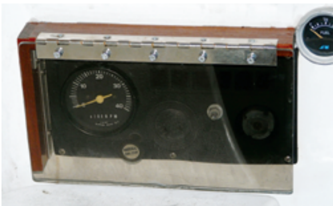
When closed, the cover protects the panel from wayward feet. Sealant along the edges keeps water from dripping behind the panel.
