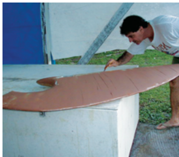
Randy used epoxy resin and biaxial fiberglass fabric for the rudder's structural skins, wrapping the fabric around the edges for strength, at left. Once the glasswork was complete, he applied a layer of microballoon paste that he would sand to give the rudder its final smooth shape, at right.
