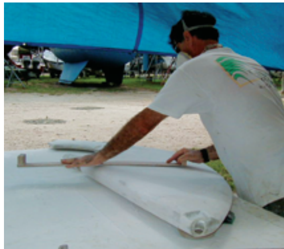
After building up the rudder's core with foam and fiberglass, Randy applied a microballoon paste, above left, which he then sanded with a longboard to eliminate any unevenness, above right.
