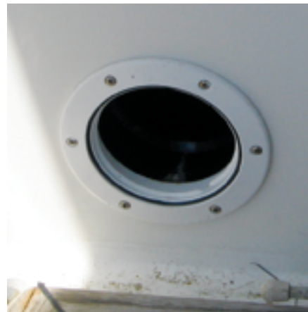
After cutting the holes in the cockpit side and the hull, John test fit the pipe that passes through the hull before marking it for cutting, at left. The trim ring on the cockpit side assures a solid installation and can be fitted with a cover if needed, at right.
