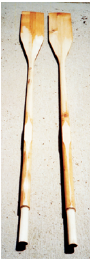
All but finished, the oars need only the means to attach them to the dinghy, above. Richard drilled holes for the bolts, at right, and cut recesses for washers with a spade bit, at top right. The shiny wooden oars lend Sigfrid's dinghy some much needed class, below.
