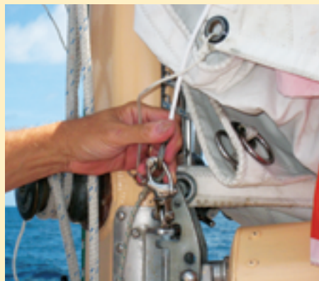
The Mainster's wire luff hooks to a snapshackle attached to the gooseneck.
