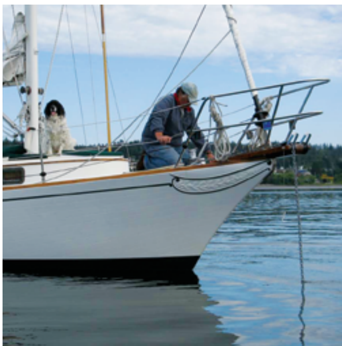
For looks and durability, Gary built the sprit of teak, at top, and stainless steel, middle, and the end result fits the boat to a T, at bottom.
