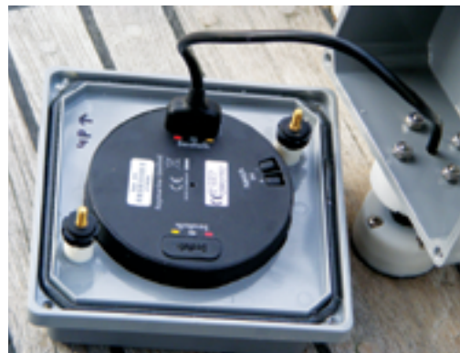
The foam gasket around the cover ensures that the junction box is waterproof.
