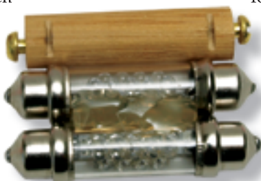
The dowel is aligned with the bulbs and notches cut in it for the binding wire.
