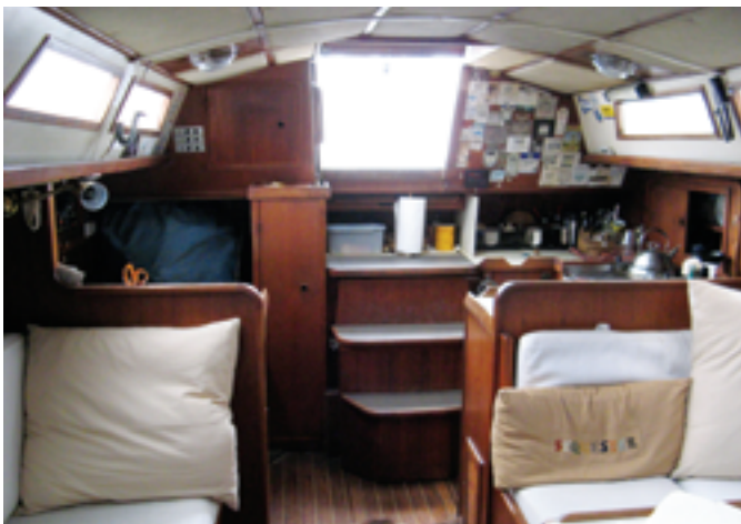
The view from the saloon looking aft, at left, shows a conventional arrangement with the chart table, quarter berth, and wet locker next to the companionway to starboard and the tight U-shaped galley to port. Forward, Duane installed a wood-burning stove to cheer up the already cozy cabin when cruising in the cool Pacific Northwest autumn, at right. The plywood bulkheads are bonded to the hull and deck for strength and stiffness.
