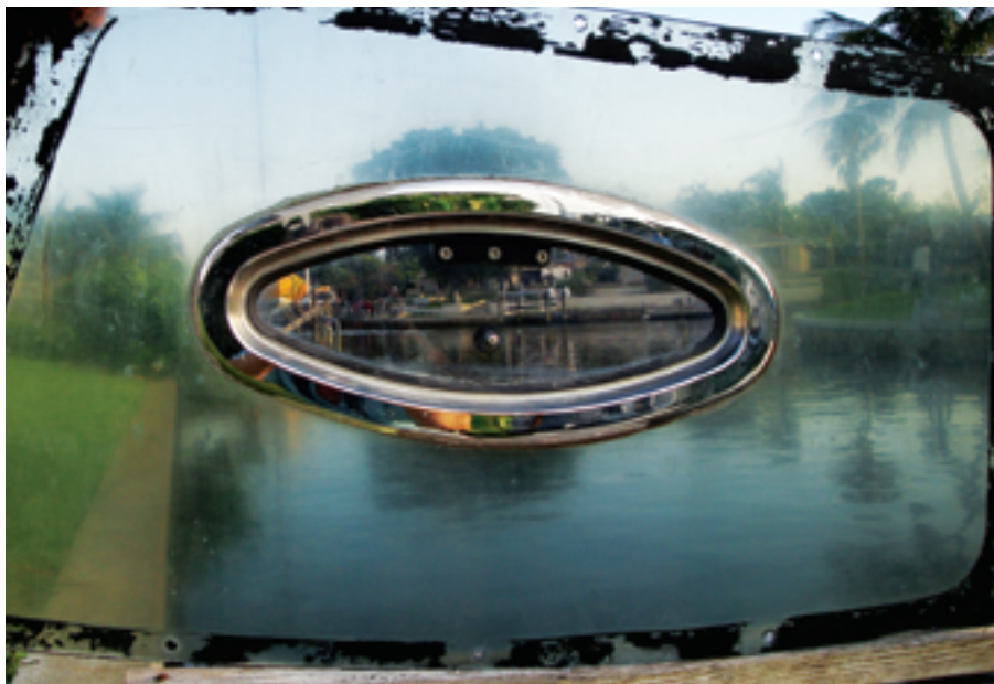
An acrylic port mounted in the center of a now sun-fogged non-UV-protected polycarbonate window provides a good comparison of how the two types of plastic withstand weathering.
