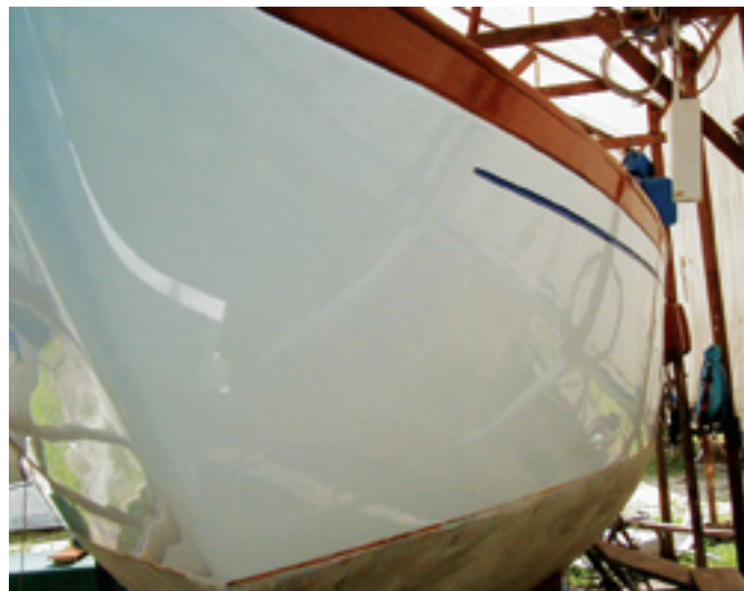
Caribee's reflection in a neighbor boat, which Randy helped paint, shows that a high-gloss finish highlights imperfections of all magnitudes in the surface it covers, from dust specks to unfairnesses bequeathed by the original hull mold, at left above. By repairing nicks, dings, and scratches, though, it's possible to get a finish at least as good as the one that emerged from the factory, at right above.
