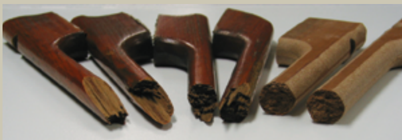
The aftermath: the through-bolted teak handhold (left), screwed teak handhold (center), and Trex handhold (right).
