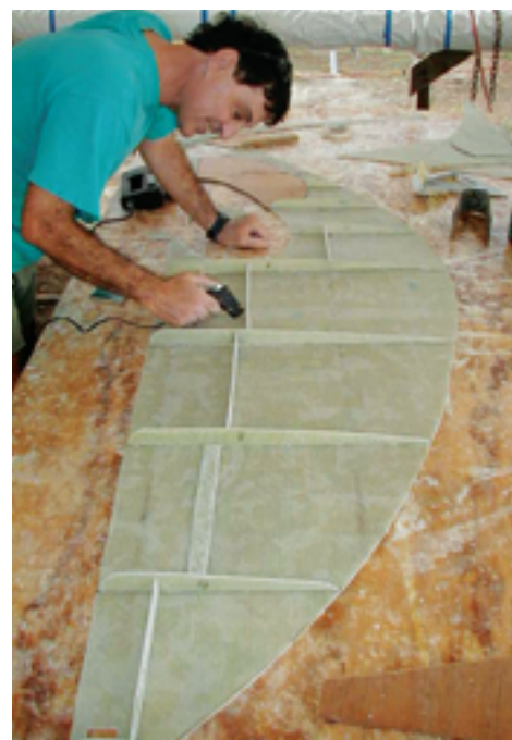
Using excess material from the same sheet, Randy cut ribs, at left, and stringers, at right, that he used to define the sectional shape of the rudder and connect the skins to the backbone.
