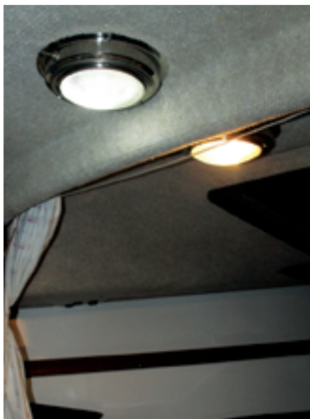
The cool-white LED bulb, above left, left fixture, is as bright as the incandescent bulb it replaced, right fixture. With its LED replacement bulb, the stern light is very bright, at right.
