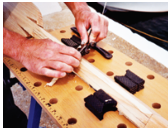
The spokeshave also came in handy for tapering the loom toward the blade.
