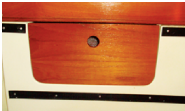
Ken made his cubby covers from plywood. They lock in place with wooden tabs and an elbow catch.
