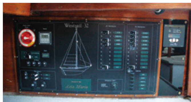
Aaron used a computer program to make a sketch of the electric panel to show to Mobile Marine Electrical Systems (MMES), at left. MMES made suggestions and, after exchanging a few drafts with Aaron, assembled a panel that met all the Norlands' needs with room for future additions, at right.
