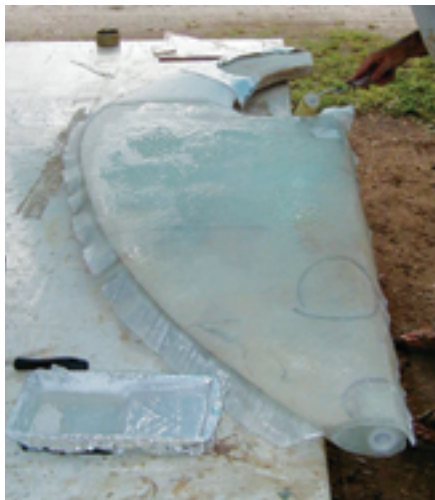
Randy used epoxy resin and biaxial fiberglass fabric for the rudder's structural skins, wrapping the fabric around the edges for strength, at left. Once the glasswork was complete, he applied a layer of microballoon paste that he would sand to give the rudder its final smooth shape, at right.
