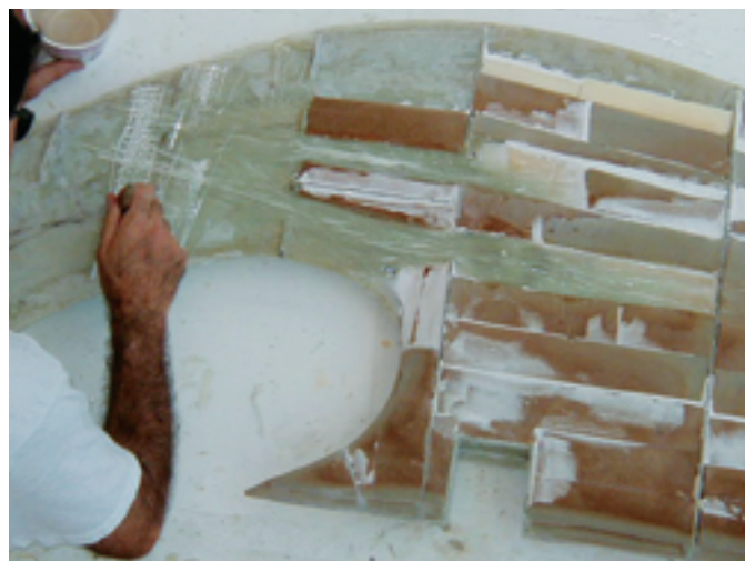
With foam strips fitted between the ribs and stringers, the rudder really begins to take shape, at left. At the top of the rudder, Randy built up the backbone with solid laminate to ensure a strong connection to the rudder stock's attachment plates.
