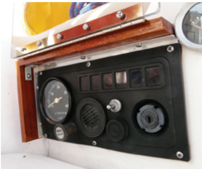
Even without the right-hand side of the frame, which he omitted because of the fuel gauge, Chris says the cover is still plenty strong.
