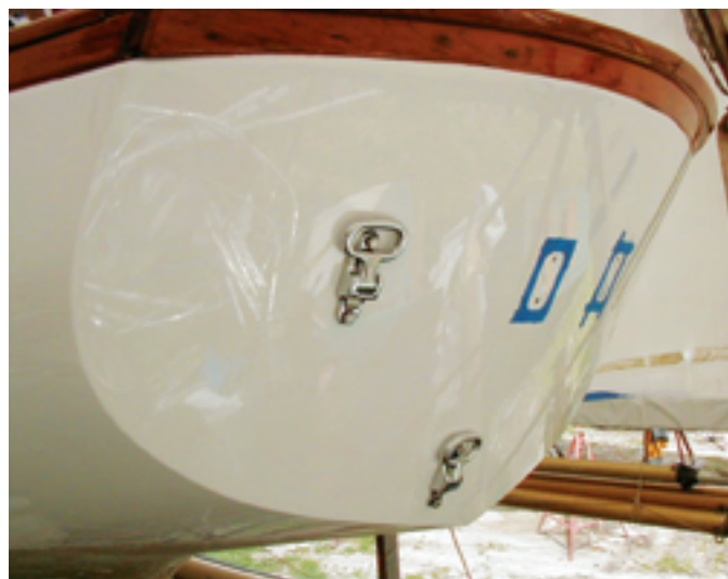
The camera caught Cheryl reflected as she appraised the finish she and Randy achieved on Caribee's topsides, at left above. The photo also shows how well the hull withstood 30-some years of sailing before receiving this treatment. The Nicholson 32's transom provided a definite edge that Randy used as a start and finish point as he rolled his way around the hull, at right above.
