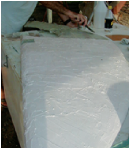
After building up the rudder's core with foam and fiberglass, Randy applied a microballoon paste, above left, which he then sanded with a longboard to eliminate any unevenness, above right.
