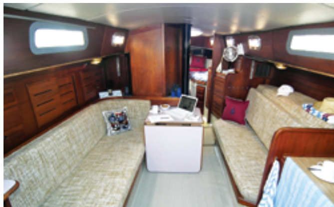
The layout of the Islander 36 broke the mold for sailboat interiors, using a disappearing table and low partitions to create an openness imitated in many designs to this day. Its designer, Joe Artese, also employed angled partitions and bulkheads to make the spaces more interesting.
