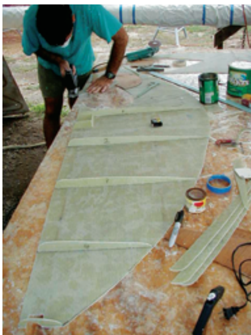
Using excess material from the same sheet, Randy cut ribs, at left, and stringers, at right, that he used to define the sectional shape of the rudder and connect the skins to the backbone.
