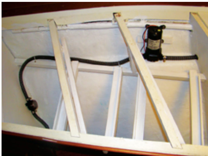
From the head intake, the wash-down supply hose passes through the bulkhead into the forward cabin, to a strainer, then to the pump, at left. The hose continues forward under the berth, at right, and into the chain locker, where it connects to the on-deck hose bib via a pipe extension, below.
