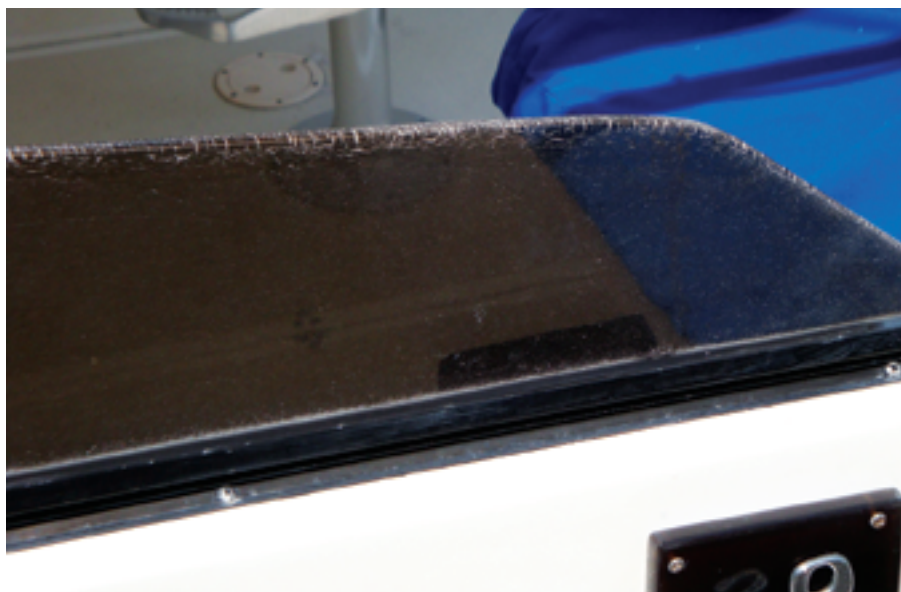
Over time, stress crazing has developed along the edge of this acrylic windscreen. It is most likely the result of overheating during fabrication caused by incorrect cutting or polishing.
