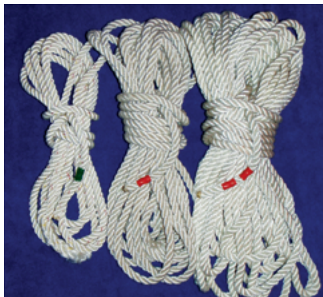
Three-strand docklines look much alike when stowed together in one place. Steve tagged the ends of his with colored tape according to their lengths.
