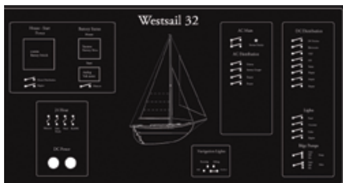
Aaron used a computer program to make a sketch of the electric panel to show to Mobile Marine Electrical Systems (MMES), at left. MMES made suggestions and, after exchanging a few drafts with Aaron, assembled a panel that met all the Norlands' needs with room for future additions, at right.
