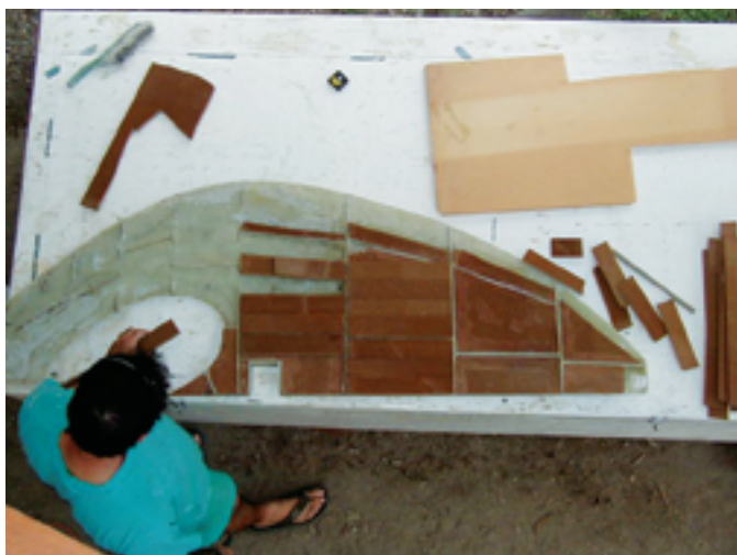
With foam strips fitted between the ribs and stringers, the rudder really begins to take shape, at left. At the top of the rudder, Randy built up the backbone with solid laminate to ensure a strong connection to the rudder stock's attachment plates.
