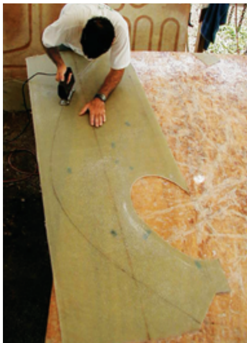
The rudder's backbone is a fiberglass sheet, above left, that is bigger than Cheryl, above right.
