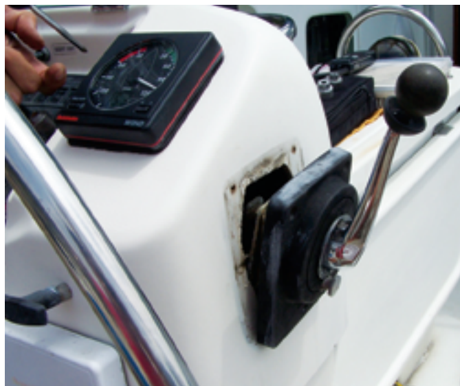
Getting to the problem end of the throttle cable, at left, entailed removing the engine instrument panel, at bottom.
