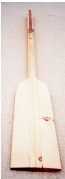
A roughed-out oar awaits refining touches to its shape.
