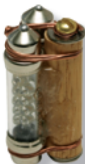
The dowel is aligned with the bulbs and notches cut in it for the binding wire.
