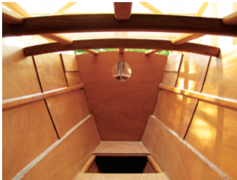
Flat plywood takes on curves in the lower part of a hull, top left, to be joined by the upper hull, top right. Sole boards and deck beams tie everything together, above.
