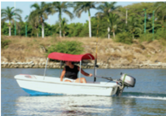
The WaterTender 9.4 has a tri-hull configuration, facing page, and can be stowed below the boom. It can plane at 15 knots with just one person, at left, and serves as the family washing machine after a rainfall, at right.
