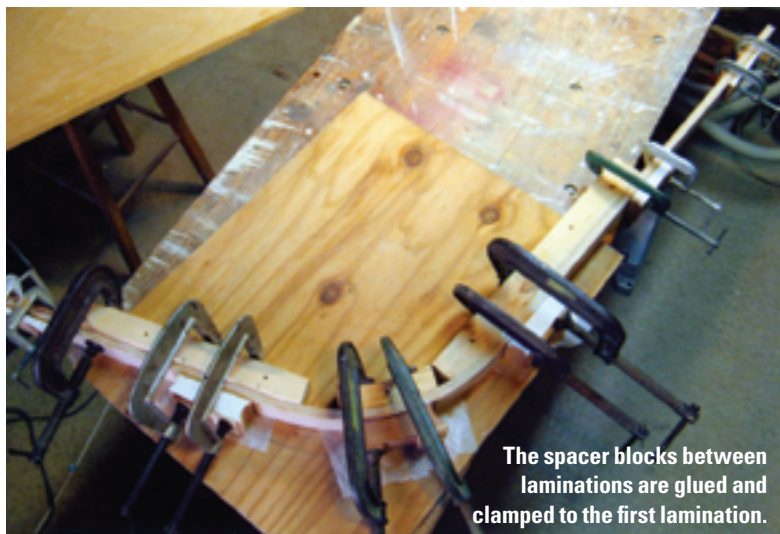
Paul wrapped a towel around the three boards to be used in the lamination and poured hot water over them. After soaking for about 20 minutes, they were pliable enough to conform to the laminating jig without cracking.
