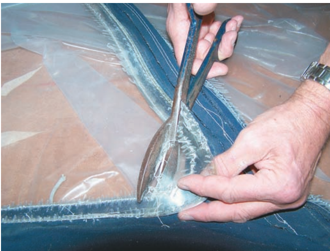
Cut away the corners of the old pane to make it easier to remove the old pane once the new pane has been sewn in, at left. Sew the new pane in place. Note the double-sided tape to the left of the sewing machine head, at right.
