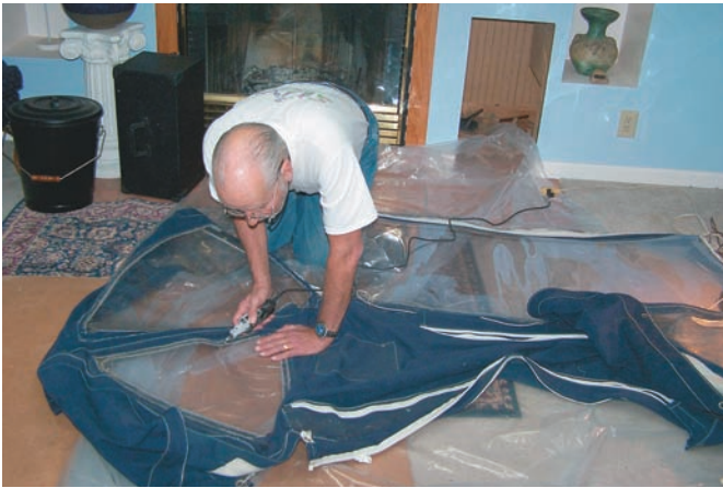
Method 2: A Dremel tool with a wire brush cuts the stitching holding the panes in place, at left. Use masking tape to lay out the shape of the opening on the replacement pane to avoid distorting the dodger when the panel is sewn in place, at right.
