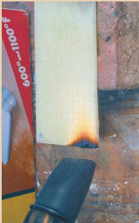
A heat gun on the 1,100° F setting charred this epoxy/fiberglass laminate, but was incapable of causing flames or glowing embers.
