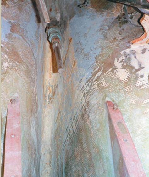
A view of the new engine beds and propeller shaft. The deep, narrow V-shape of the hull in the engine location is what created this exhausting problem.
