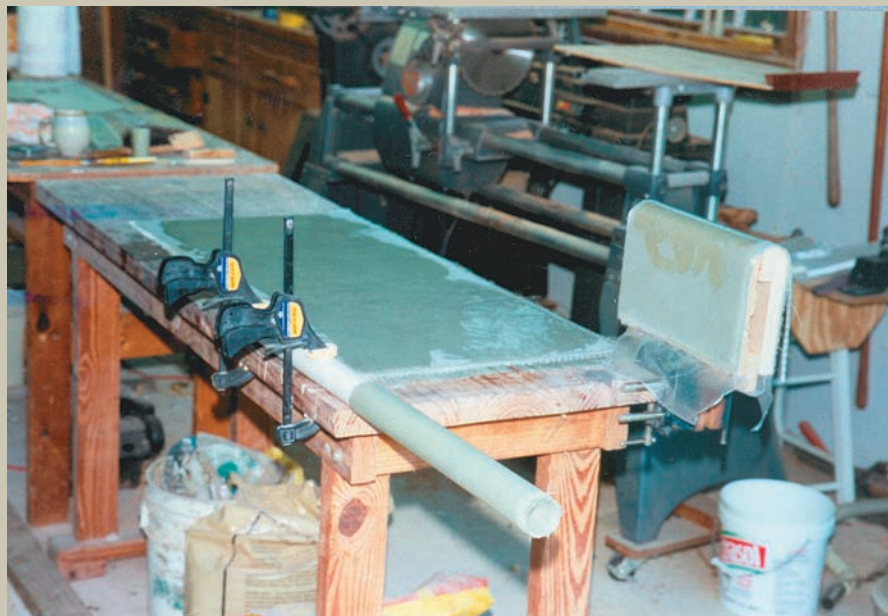
On Paul's workbench are the three components from which the waterlift muffler was built: on top of a waxed plate-glass mirror, he laid up a sheet of fiberglass for the sides, top, bottom, and ends. The fiberglass tube, made by winding epoxy-saturated fiberglass cloth around a PVC pipe, became the inlet, outlet, and crossover tubes. He also laid up — over a wooden male mold — the valley to allow the propeller shaft to pass through the waterlift. That assembly is to the right.
