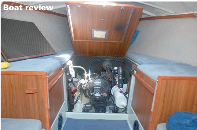
Lifting the center panel of the V-berth, at left, provides excellent access to the single-cylinder Yanmar diesel engine. During the late 1970s, Yanmar manufactured three models of small, horizontal diesels. When restored to its full size, the V-berth, at right, is very spacious. A portable toilet is located underneath the seat cushion to starboard.
