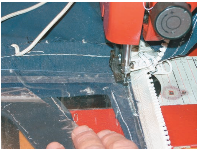
Cut away the corners of the old pane to make it easier to remove the old pane once the new pane has been sewn in, at left. Sew the new pane in place. Note the double-sided tape to the left of the sewing machine head, at right.
