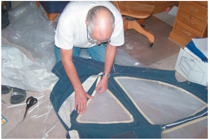
Method 2: A Dremel tool with a wire brush cuts the stitching holding the panes in place, at left. Use masking tape to lay out the shape of the opening on the replacement pane to avoid distorting the dodger when the panel is sewn in place, at right.
