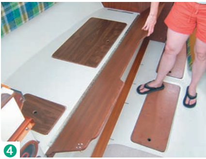
Andie unbolts the bunk board and lets it swing down into berth extension mode (4). The forward end of the berth extension rests on a block in the bulkhead (5). The fiddle will retain the new insert cushion, yet to be made (6).
