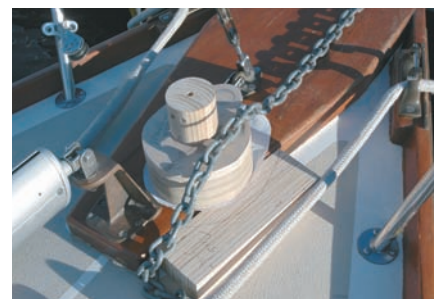
John used scale models to try out possible areas on the deck for the location of the windlass. The chain stretching aft pointed the way to the best location for the equipment.
