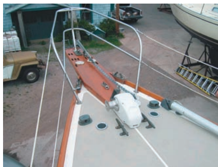
John's Cape Dory 36, in top photos, before and after the installation of an anchor windlass. He selected a vertical windlass after considering both types. A horizontal windlass is shown above.
