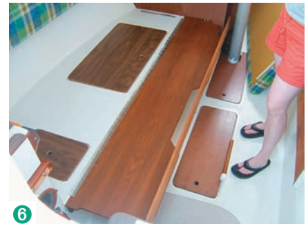
Andie unbolts the bunk board and lets it swing down into berth extension mode (4). The forward end of the berth extension rests on a block in the bulkhead (5). The fiddle will retain the new insert cushion, yet to be made (6).
