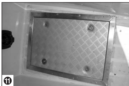
Engine on risers (10). Metal inspection hatch — normally covered by teak grating (11).
