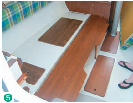
Andie unbolts the bunk board and lets it swing down into berth extension mode (4). The forward end of the berth extension rests on a block in the bulkhead (5). The fiddle will retain the new insert cushion, yet to be made (6).
