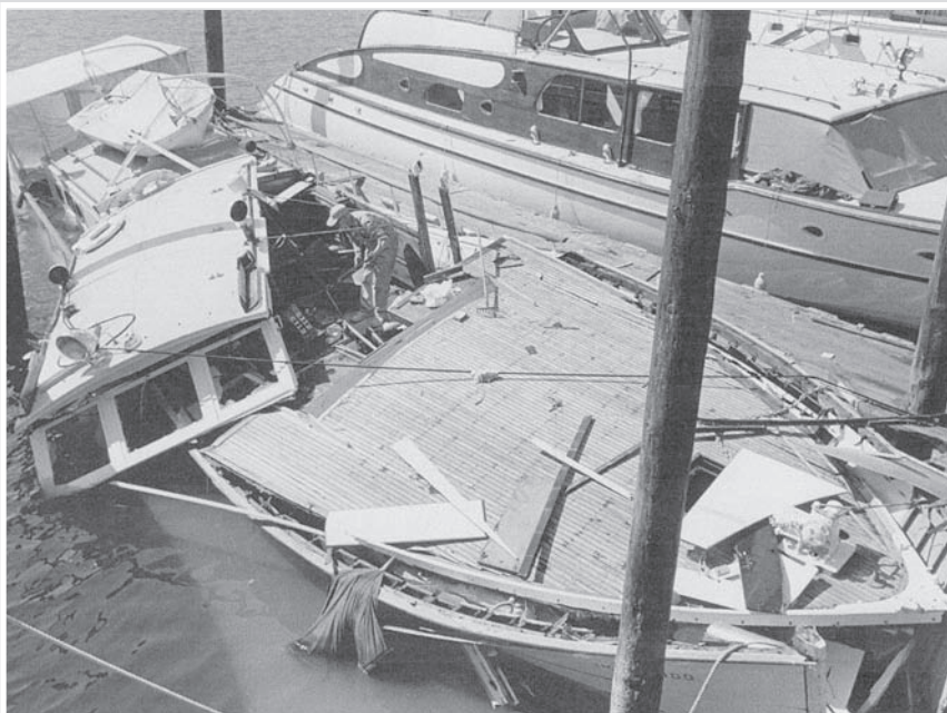
I was standing about 100 feet away on a dark night in Sausalito, California, when the propane heating unit of this power yacht blew up with an explosion that was heard 2 miles away. A woman was aboard who was blown out of bed but not hurt. Note how the stem has been ripped apart.
