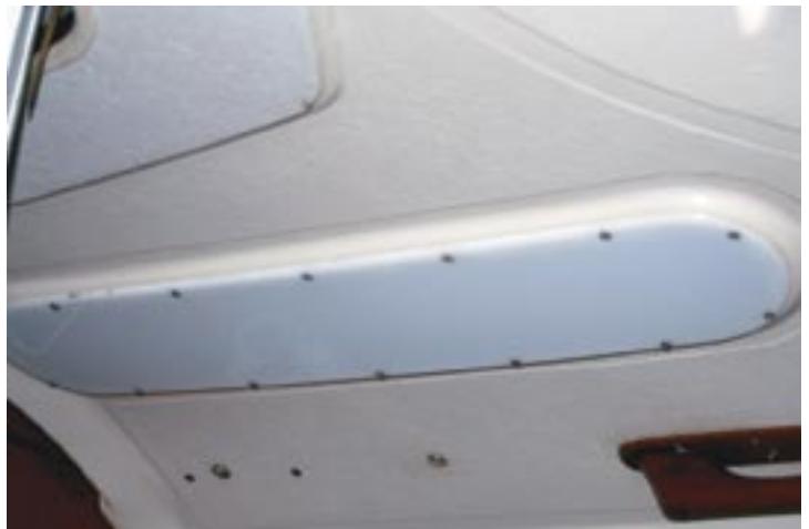
At left above, forward-facing navigation station, and at right, one of the many overhead panels giving access to deck hardware.
