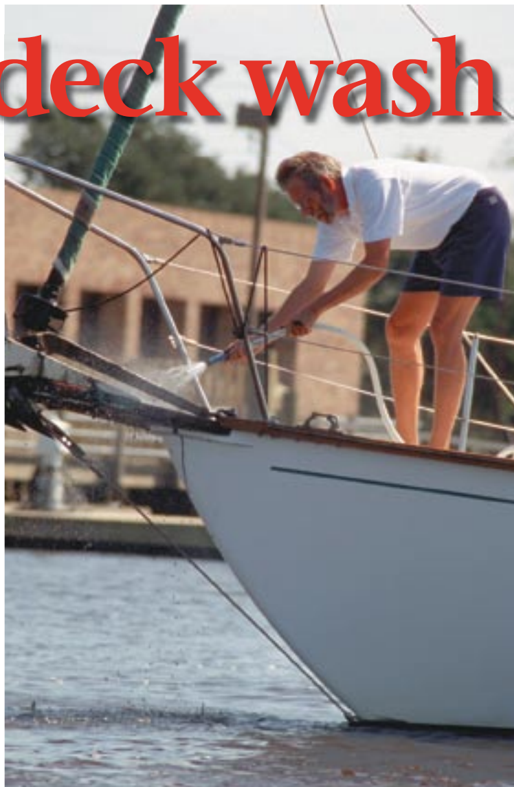
Don Casey puts his deck-wash system to good use after the anchor is hauled, above. The on-deck portion of the system, on Page 38, consists of a short hose and a small deck fitting.
