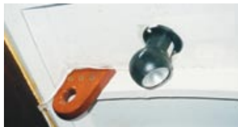
Detail of one of the mahogany blocks fastened to the cabin's rafter to hold one end.
