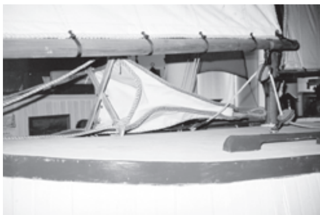
Capt. Voss' famous sea anchor lies atop Tilikum's coachroof, above left. Folding wooden braces hold the mouth open. The material is thick canvas, heavily roped around the edges. The fearsome Canadian Indian figurehead, above right, was kicked by a horse and damaged when Voss took Tilikum overland on exhibition to Pretoria, South Africa. After repairs, it was as good as new.
