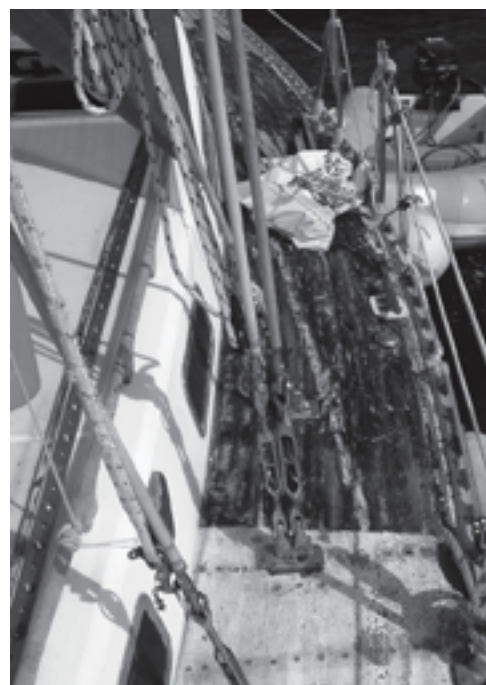
Doug removes the last piece of teak, at top. The tar bedding, at right, was removed with diesel fuel.
