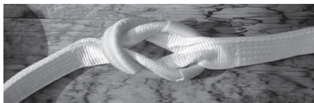
Two heavy-duty vehicle recovery straps, top, when looped together, center, become a boat-retrieval belt, bottom, with a rated capacity of 18,000 pounds.
