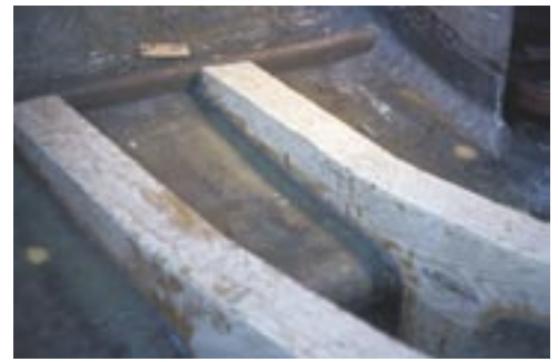
To stabilize the keel, Dave built box-section keel floors using \frac{3}{8} -inch marine plywood, sheathed in fiberglass, then laminated to the hull, above. A hard dodger and fiberglass doghouse, below left, prevented seas from entering the cabin. Launch day, below right.
