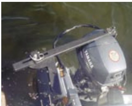
The outboard-motor/rudder connecting bar.
