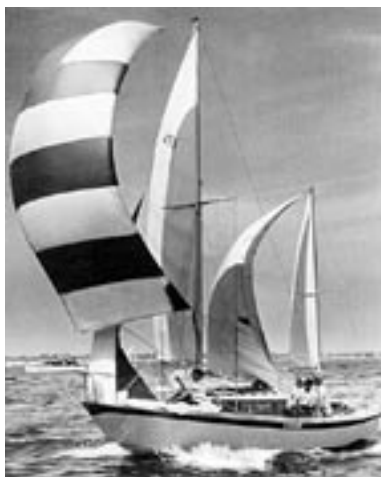
Charley Morgan's first boat, Brisote . Demonstrating considerable resourcefulness, she had a Star Boat keel and rudder, a Thistle mainsail, and a modified Penguin sail for a mizzen.
