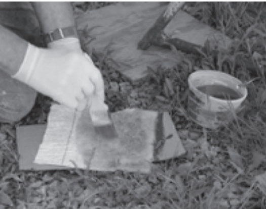
Bob makes the pattern for the patch, top. He cuts the fabric and lays out the patch material in readiness for wetting, middle photos. The laminate is wet out, bottom.
