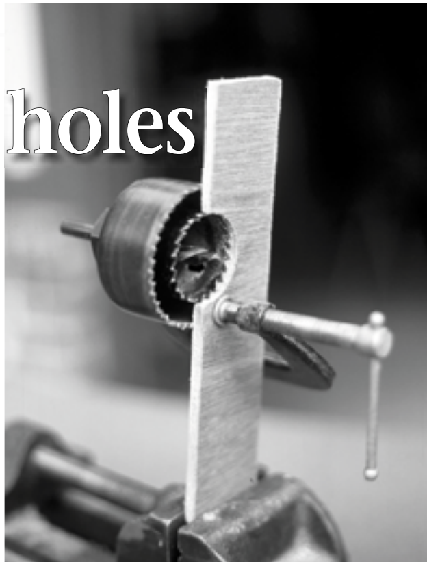
One clever way to enlarge a hole — without having an existing center for your hole saw — is the saw-within-a-saw trick, illustrated here in cutaway view.
