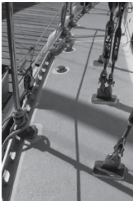
The finished deck with its gray non-skid accent. Doug and Diane say it's cooler on bare feet, and the leaks have been (mostly) conquered.
