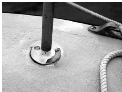
Tracing rust stains to their source can aid in identifying the source and type of corrosion.
