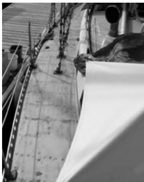
With the teak and the goo gone, Doug templates filling all the holes, at top. The prepared deck awaiting the primer coat, above.
