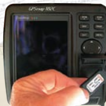
The chart chip is easily accessible, and changing it takes only a few seconds
