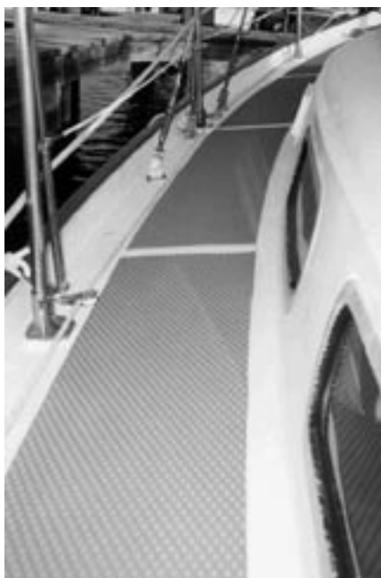
Fitting the Treadmaster to the contours of the deck, trimming the pieces, test-fitting the cut sections, and creating the corner contours.
