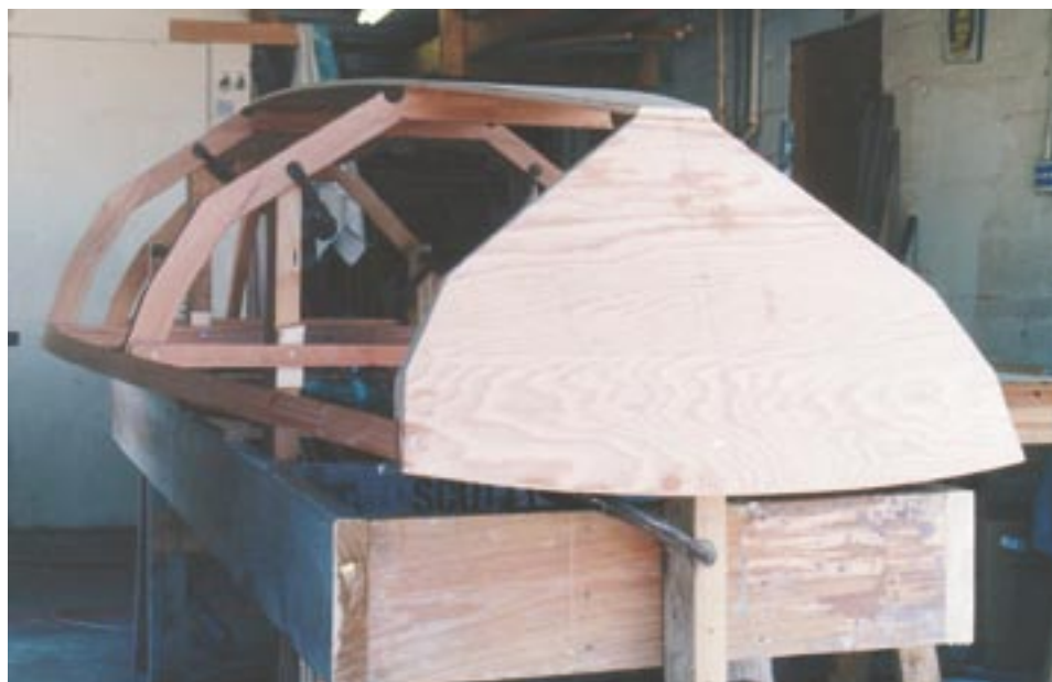
Gandy Dancer under construction in Reuel's Key West shop, showing simplicity of construction. Note the lapped frame components.
