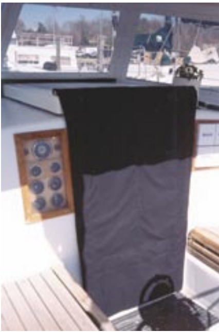
The completed insulated flap, at left above. Top teak strip mounted on the companionway hatch with male-part Lift-the-Dot fasteners in place, above center. The inside of the
