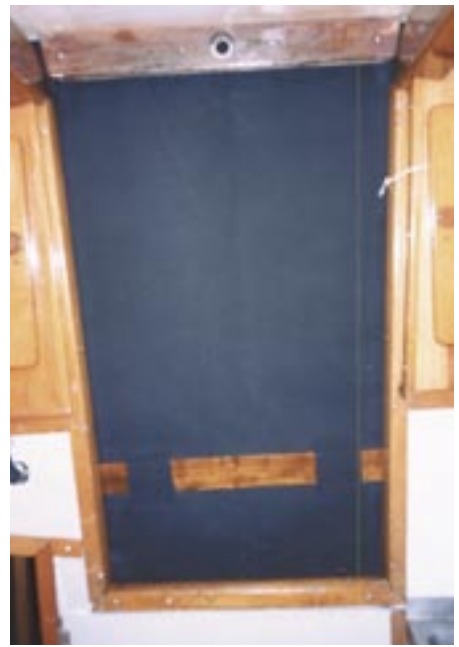
door flap, at right above. The wood piece is secured in the hatchboard slot to keep the flap from being lifted in a following wind.
