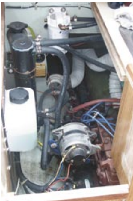
The machinery spaces on Aldebaran , an A model, are accessed through the cockpit seat hatches. Aldebaran has her original Atomic 4 thanks to a rebuild by Don Moyer of Moyer Marine and an improved propeller by Indigo Electronics. Note the screw and crank for tensioning the outhaul on the roller-reefing boom, below.
