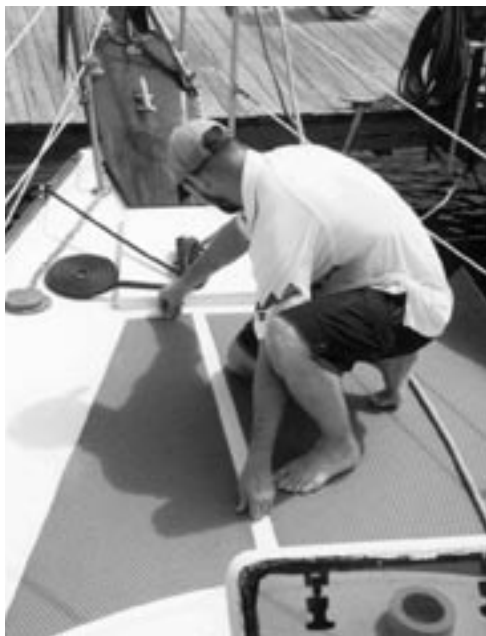
Fitting the Treadmaster to the contours of the deck, trimming the pieces, test-fitting the cut sections, and creating the corner contours.
