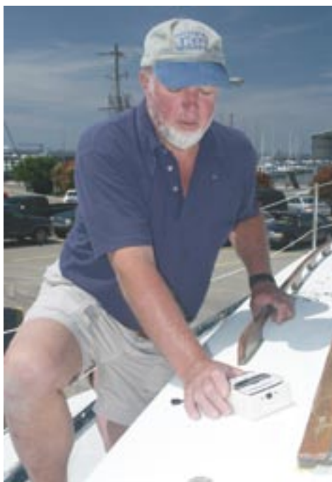
Bill Sandifer measures a deck on a boat under survey. Fortunately for the owner, the deck and hull proved to be dry with no problems.
