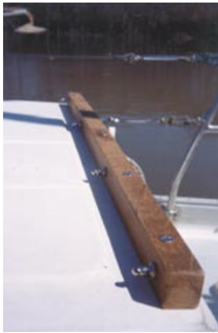
The completed insulated flap, at left above. Top teak strip mounted on the companionway hatch with male-part Lift-the-Dot fasteners in place, above center. The inside of the
