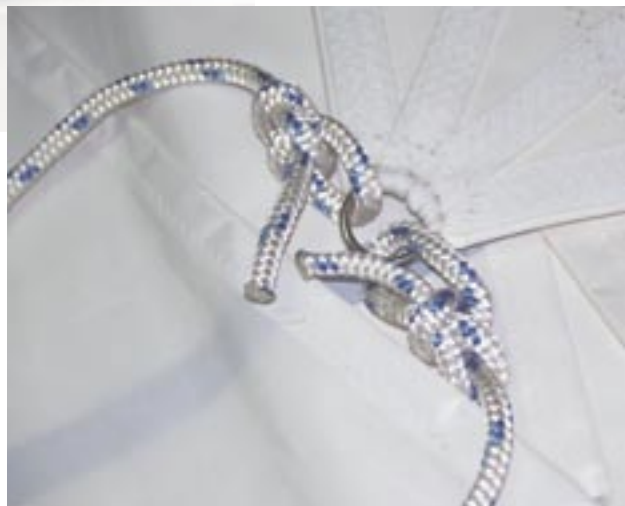
A properly cleated line, top. Bowlines, above, used to tie genoa sheets to the sail's clew. A clove hitch used to secure lifelines to the stanchions on a gangplank, at left.
