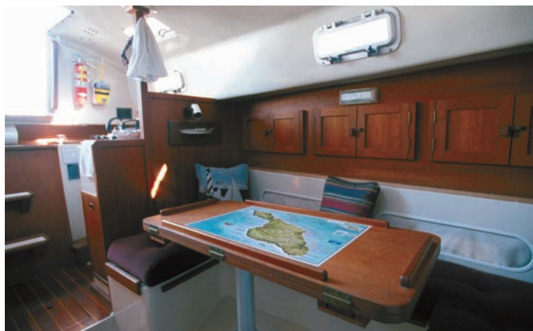
Headroom in the Contessa varies from 6 feet 1 inch to about 5 feet 10 inches. Views here are of Gerry and Allan Hodge's Contessa , at left, and Richard Whitehouse's Ceres , at right. Both are J. J. Taylor boats and show that builder's trademark fiberglass interior moldings trimmed with wood.
