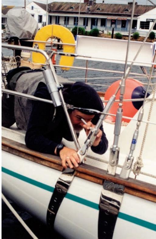
Brion inspects the rigging on Ono with a 50x handheld microscope.
