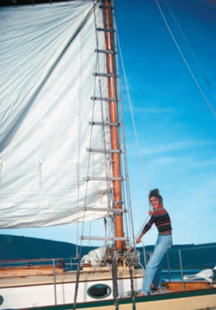
At left, Jill Knight raises Cooe 's big gaff mainsail. Three-to-one purchase on both throat and peak halyards means this is not difficult even without winches. The headsails, center, are raised using belaying pins: easy and simple (See "Advanced swigging," Page 59). At right, even engines can be beautiful. Cooe has a lightweight Westerbeke 20B. Jill is adjusting the valve clearances with guidance from the manual.
