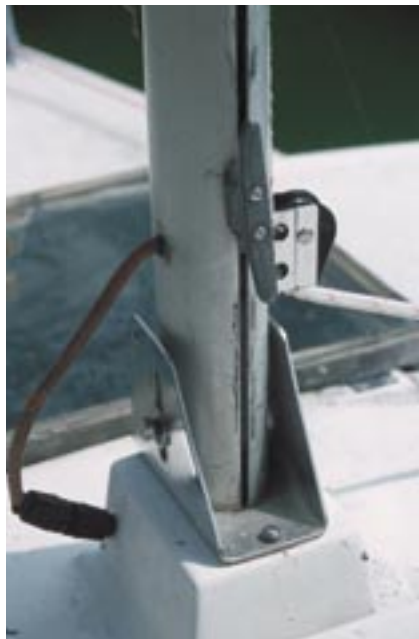
The deck-stepped mast is supported by a wooden compression post belowdecks.
