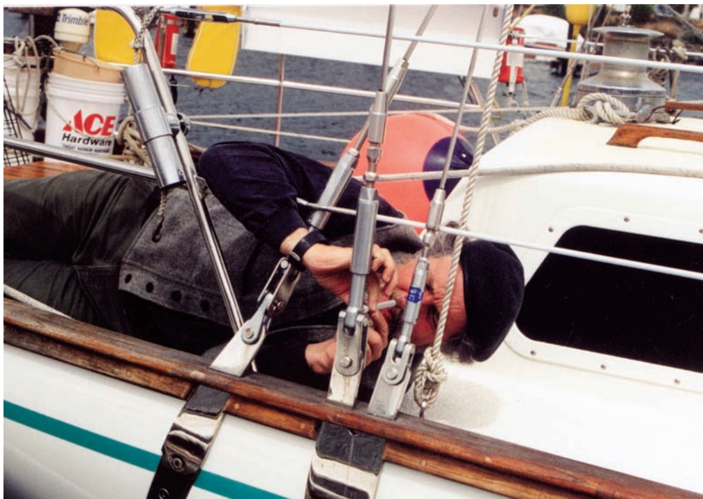
Brion inspects the shroud terminals on Ono , a Mariner 60.
