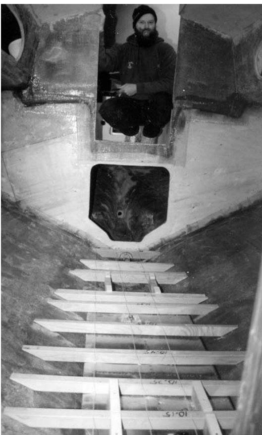
Dave Fox surveys the newly installed floor beams in the gutted interior, at left.
