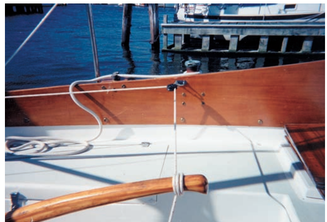
A Norvane installation showing the use of a windvane system with a tiller
