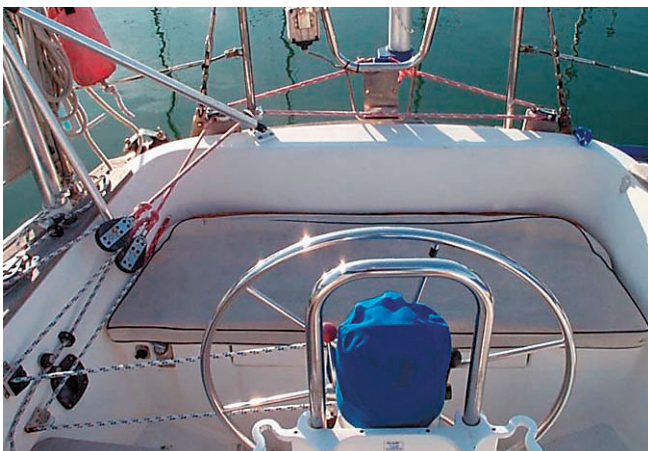
A Sailomat installation leads lines off to one side of the helm so climbing over lines is unnecessary.
