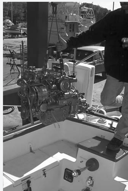
The Travelift brings in the new engine.
