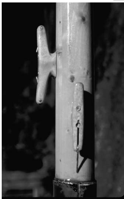
Cleat, at left, in normal use and, above, with "fingers" deployed to prevent line from snagging on the cleat.
