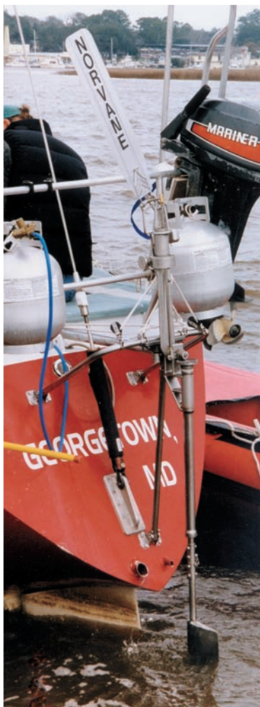
A Norvane installation, at left. The Sailomat installation, center, allows for autohelm steering . . . a help when the wind doesn't blow. A typical Cape Horn installation is shown, at right.
