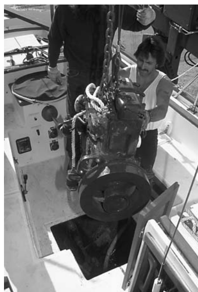
The old diesel is lifted out using the marina's Travelift.
