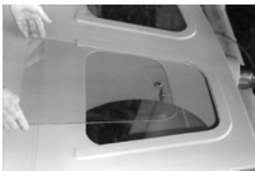
Dabbler's removable, waterproof, polycarbonate windows.
