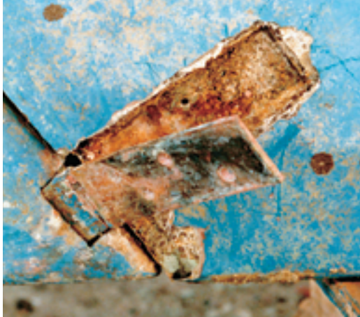
A corroded and unsalvageable hinge, above. Melissa inspects the empty rudder shell, at right, after chiseling out the bronze shafts for inspection.
