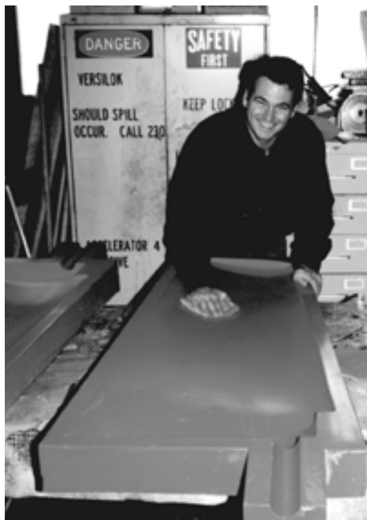
Rob waxes a rudder mold.
