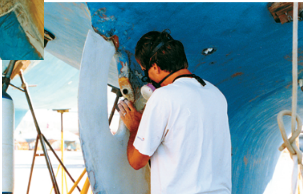
Sandy fills the large voids around the upper shaft with polyurethane insulation foam, above, before doing the final glassing and fairing at right.
