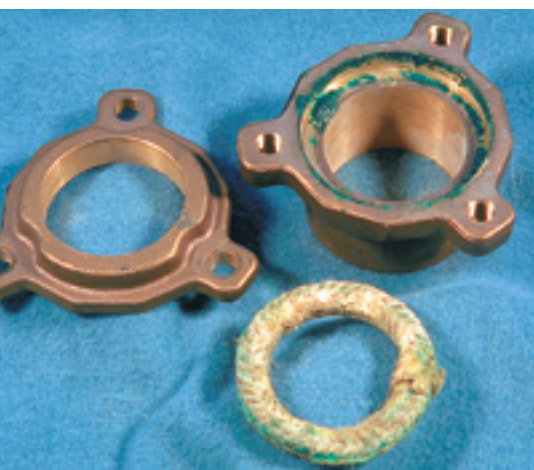
Stuffing box parts, above, and the stuffing box glassed to the rudder tube, at right. Courtesy of Edson International.
