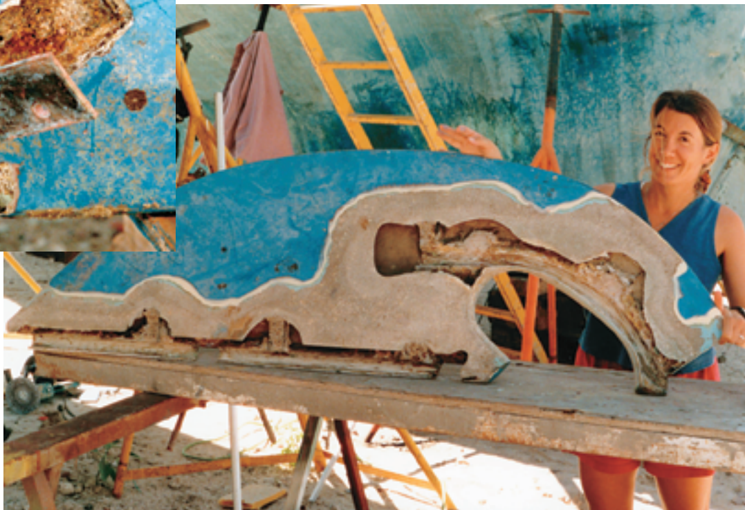
A corroded and unsalvageable hinge, above. Melissa inspects the empty rudder shell, at right, after chiseling out the bronze shafts for inspection.
