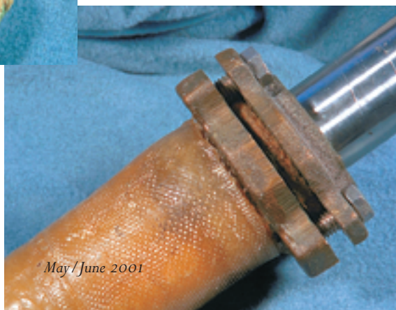
Stuffing box parts, above, and the stuffing box glassed to the rudder tube, at right. Courtesy of Edson International.
