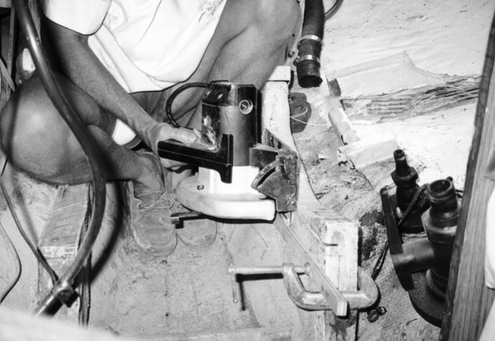
Cutting down the engine stringers to the correct height.
