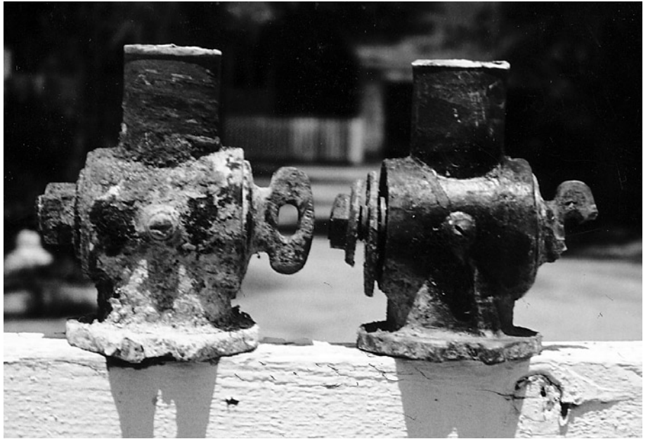
Badly corroded seacocks which Bill removed from his "new" Eastward Ho 31.
