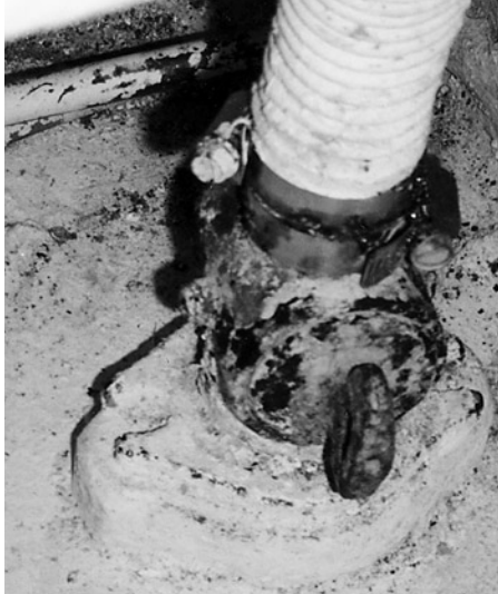
A hose clamp and fitting "with bad attitudes" from Bill's boat.
