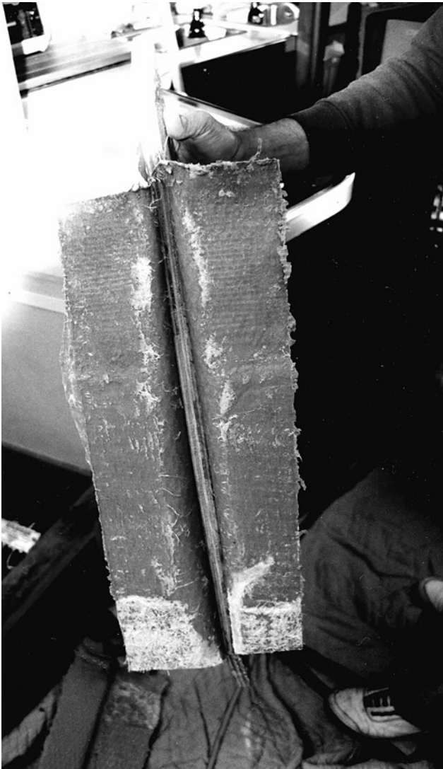
This secondary bond failed when yanked on with one hand. The builder didn't pay attention to getting a good secondary bond and didn't fillet the corners before tabbing.
