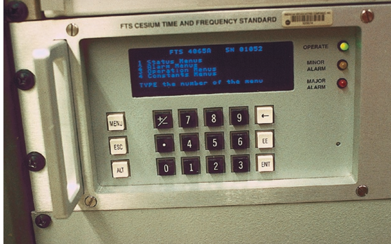
Cesium Standards (atomic clocks) such as this are used by the television networks to control their time and frequency. (Photograph courtesy of David Fredericks, ABC-TV.)
