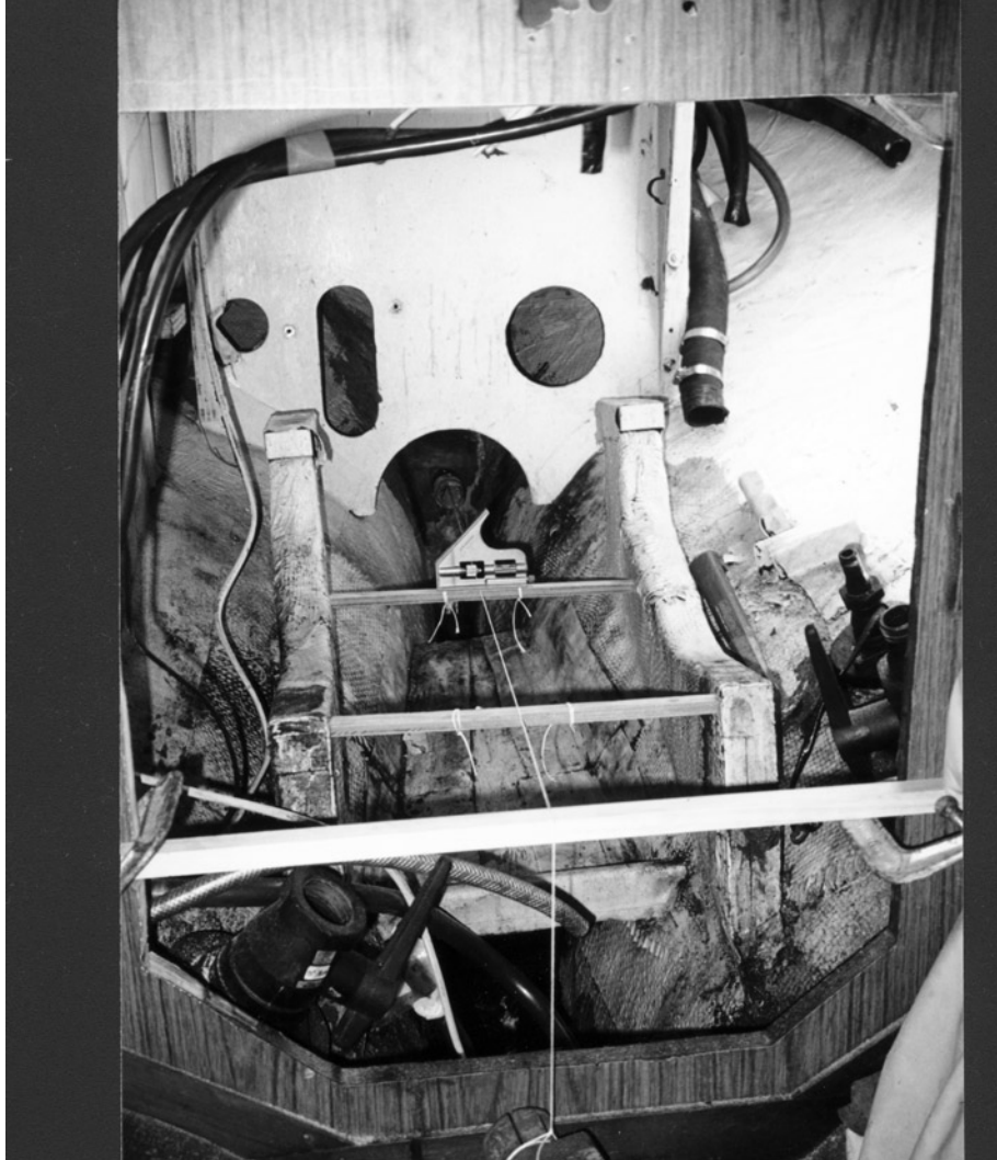
Leveled cross pieces just touch the centering string and help transfer the shaft centerline to the stringers.
