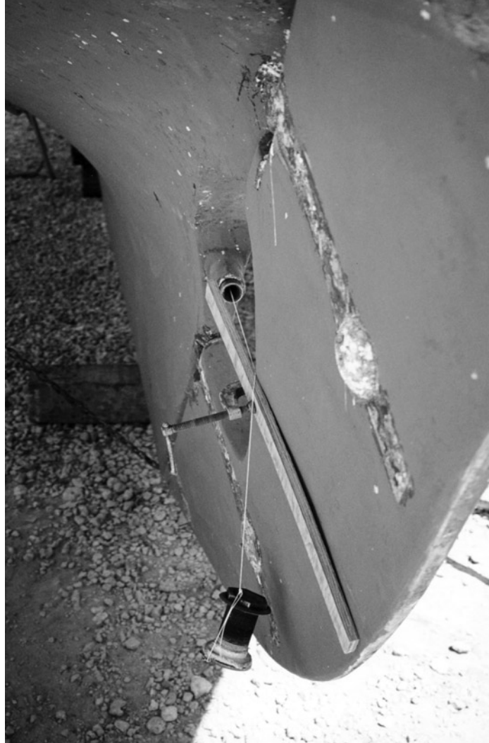
Using a centering string to determine the propshaft centerline.
