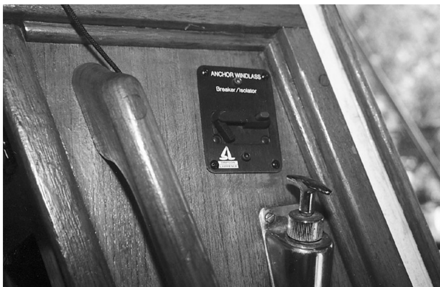
For easy access from the cockpit, the 50-amp circuit breaker and up/down toggle switch is mounted inside the companionway, adjacent to the controls for starting and stopping the engine.
