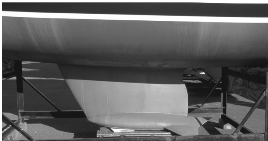
At top, a rather squared-off fin, not unlike the Cal 40 keel. In center, a less extreme fin than the one pictured on Page 13, with a more parallel tip. At bottom, a contemporary bulb fin with winglets.
