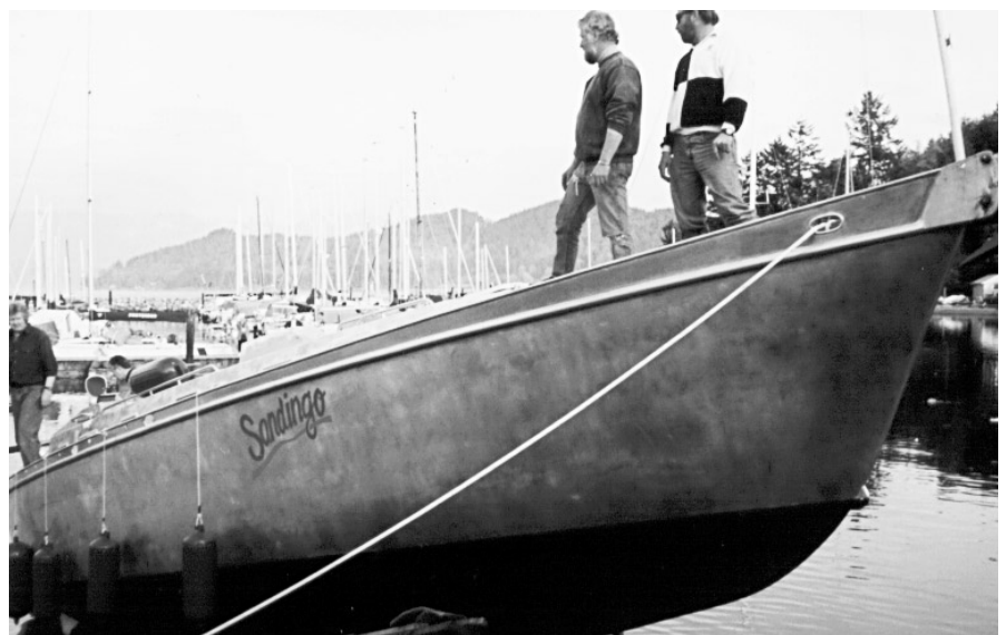
Nomad (top) has an aluminum deck and house on a steel hull. Sandingo (bottom) is launched with unpainted aluminum topsides and deck.
