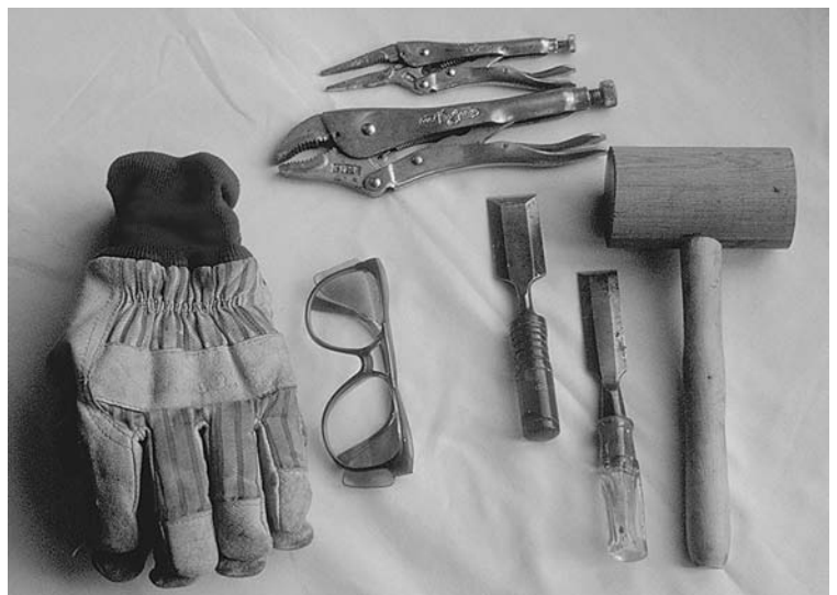
It takes gloves, eye protection, Vise-Grip pliers, wood chisels, and a wooden mallet to safely remove some obstinate gear.
