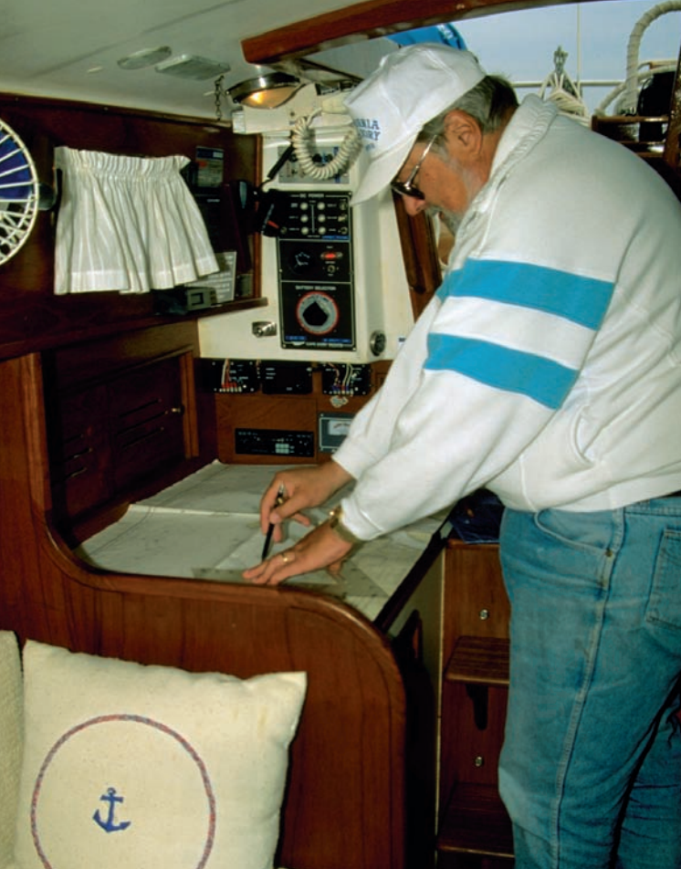
Larry made the ice box serve a double purpose when he created a fold-down cover that makes use of a two-way piano hinge to create a chart table.
