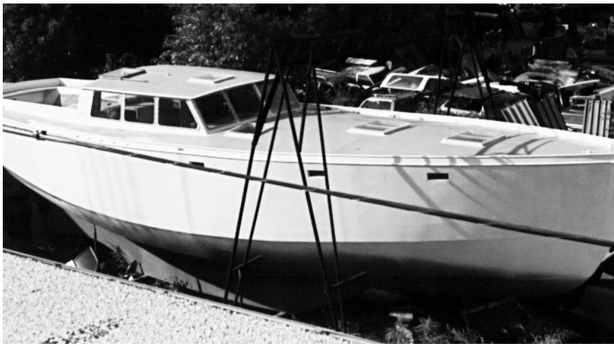
Brewer's Alaska 43 is an example of a double-chine steel hull.
