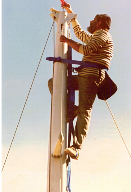
Mast Mate steps and the Workbelt patterned after a lineman's belt, above. A close up of the steps, below left.
