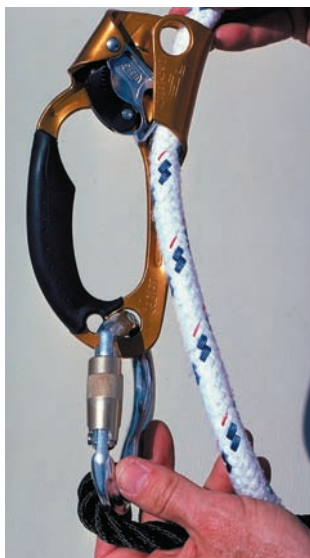
The Petzl ascender slides up and locks on a 1/2-inch line.
