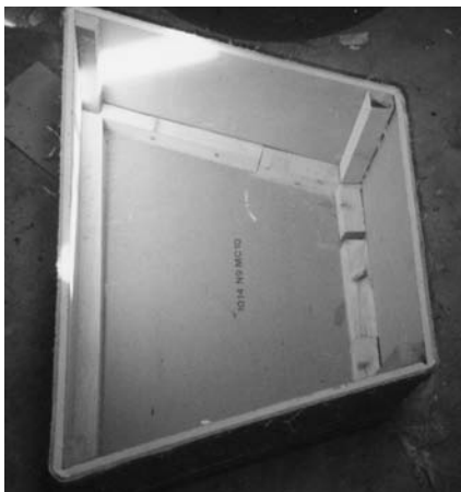
Tank with mold inside shows framing and corners.
