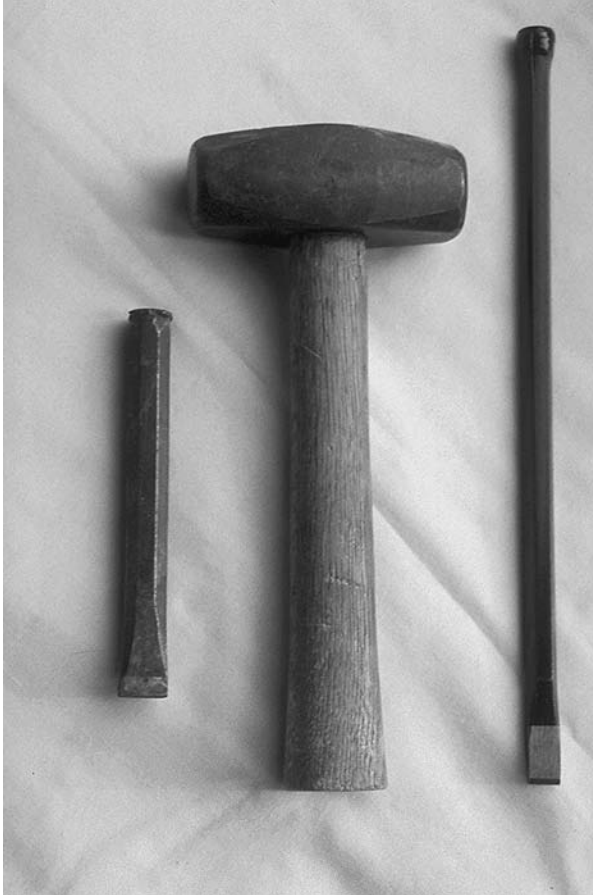
Cold chisels and a two-pound hammer are used to break the fault line once a stubborn nut has been weakened.
