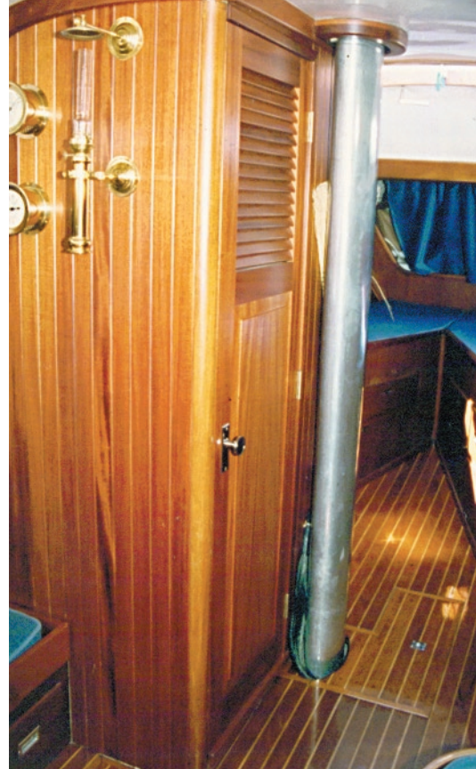
The original linoleum floor was replaced with a handmade teak-and-holly sole, and original mahogany veneer was replaced with solid mahogany.
