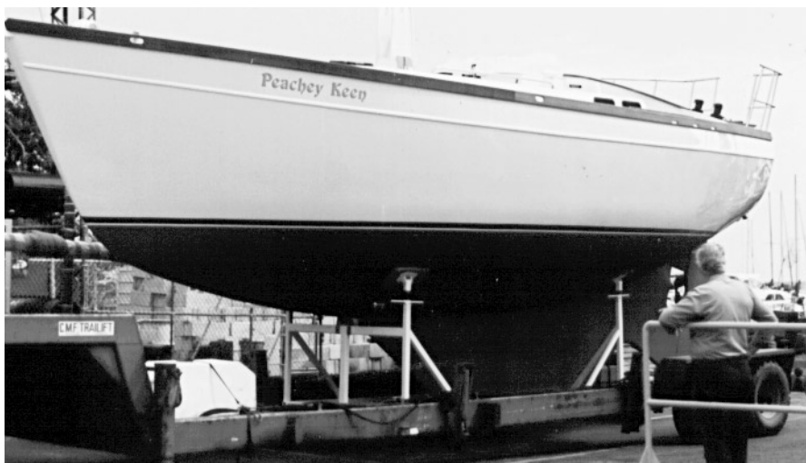
Peachy Keen, in various stages of development, shows Brewer's radius bilge with straight frames above and below the radius bilge. When plated, the radius bilge goes on in short sections while the flat areas are installed in long plates. Ready to launch, the boat's a beauty.
