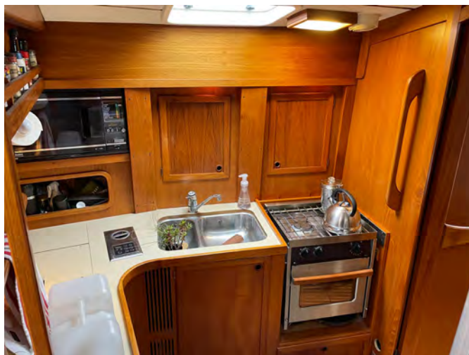
The L-shaped galley features a double sink, gimbaled stove/oven, a microwave, icebox with refrigeration, and good storage, top left.
