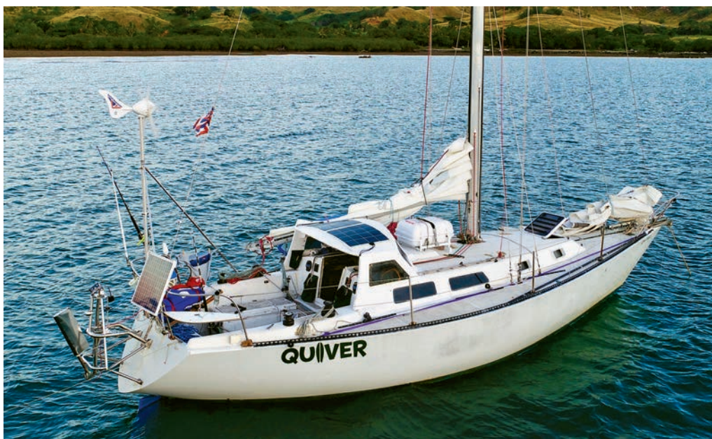
Quiver at anchor. Note the split genoa tracks, with a section far forward, which lets Ronnie closely sheet his smallest headsails, at left.
